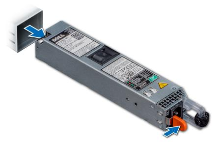
Figure 97. Removing a power supply unit
