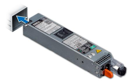
Figure 98. Installing a power supply unit
