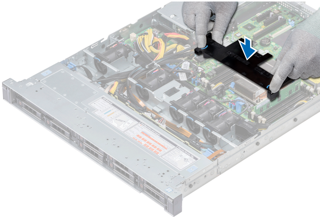
Figure 24. Installing the air shroud
