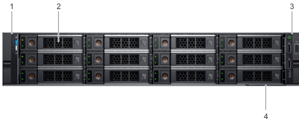
Figure 2. Front view of 12 x 3.5-inch drive system
