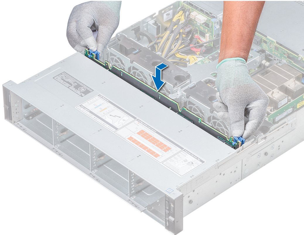
Figure 102. Installing the backplane
