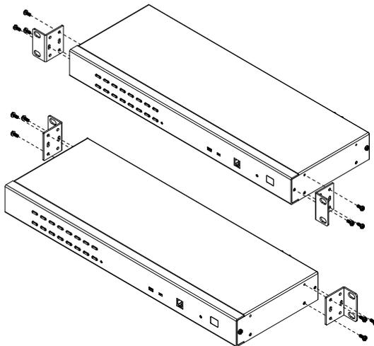
3. Slide the unit into the front or rear of the rack and secure it to the rack.
