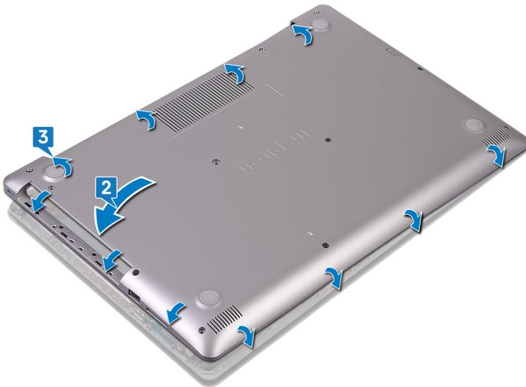
4. Replace the six screws (M2.5x7) that secure the base cover to the palm rest and keyboard assembly.
