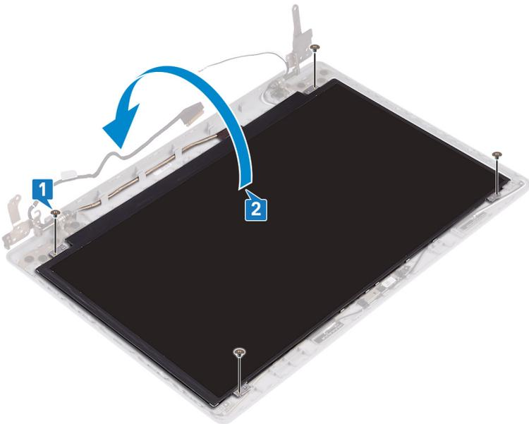
3. Peel the tape adhering the display cable to the back of the display panel.
