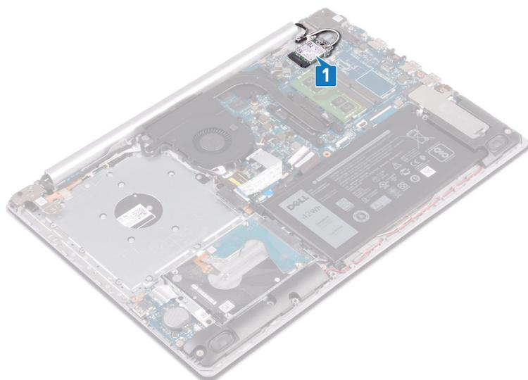
2. Remove the screw (M2x3) that secures the wireless-card bracket to the system board.
