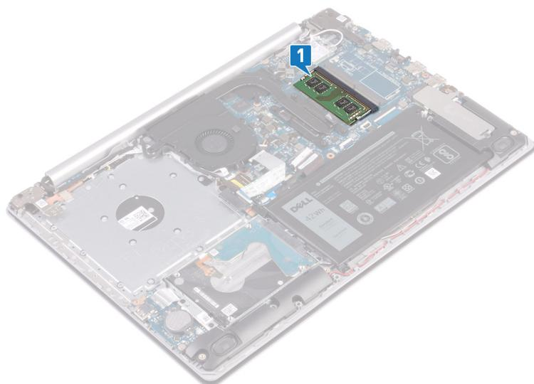
2. Use your fingertips to carefully spread apart the securing-clips on each end of the memory-module slot until the memory module pops up.
