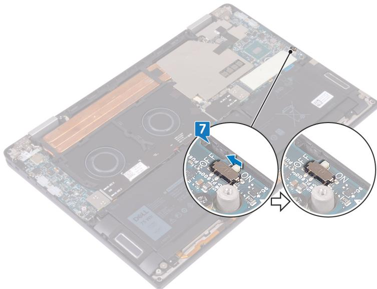
**NOTE:** Turn-off the battery switch before you proceed to remove any other component from your computer.
