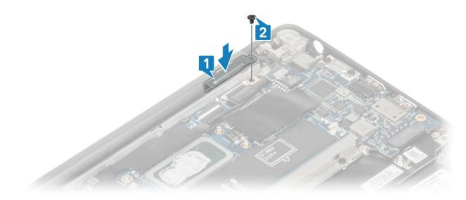
8. Install the rubber routing channel on the coin cell.
