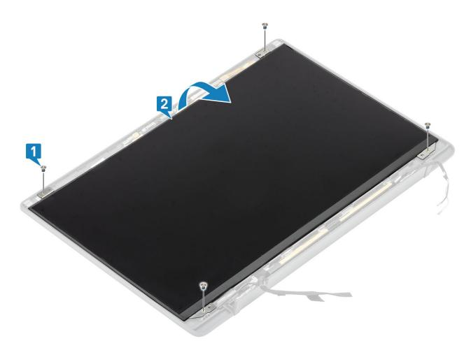
2. (i) NOTE: Do not pull and release the Stretch (SR) tapes from the display panel. There is no need to separate the brackets from the display panel.
