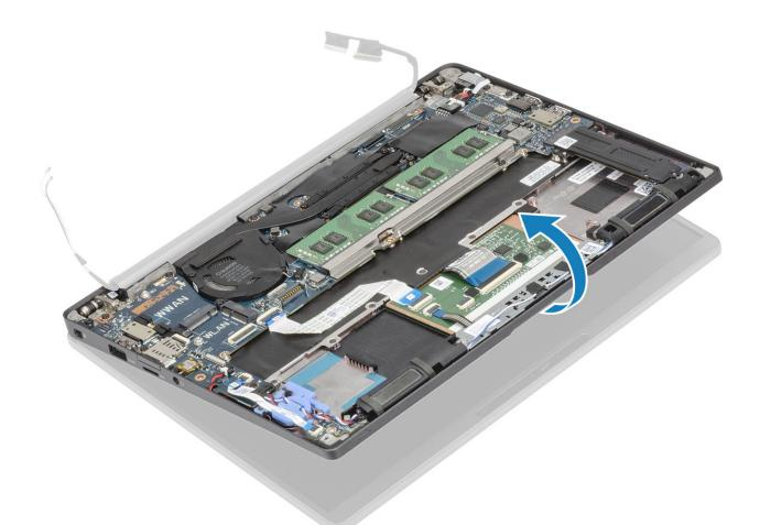
2. Remove the six (M2.5x4) screws [1] and remove the display assembly from the palmrest assembly [2].
