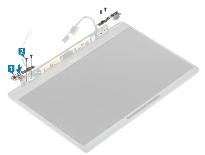
3. Route the antennae and display cable along the hinges.
