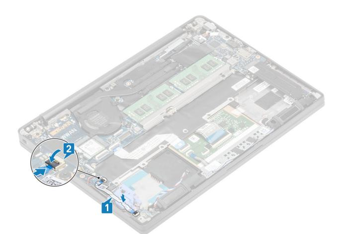
CAUTION: Route the speaker cable [1] over the LED daughterboard and then connect it to the system board [2] to prevent damage to the speaker cables.
