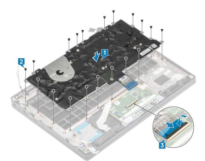
(i) NOTE: Backlit keyboards have an extra backlight cable to be connected to the touchpad module.
