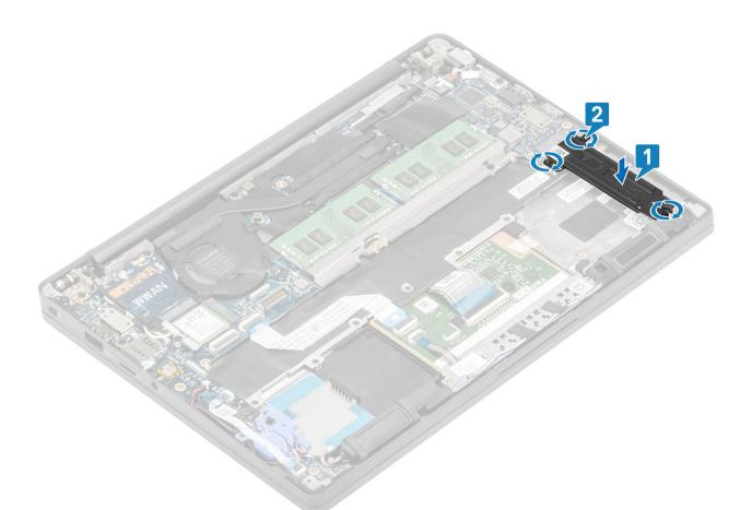
i NOTE: This procedure illustrates a M.2 2280 SSD. M.2 2230 SSD requires a special bracket and plate to secure it to the palmrest assembly.
