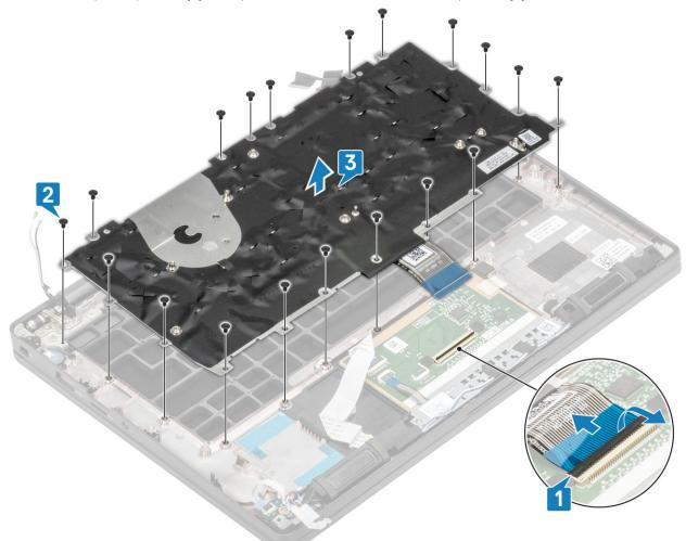
3. Remove the two (M2x2) screws [1] to lift the keyboard from the keyboard support plate.
