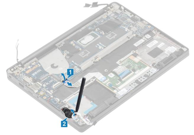
10. Remove the single (M2x4) screw [1] and remove the metal bracket over the WWAN Darwin antennae cable [2].
