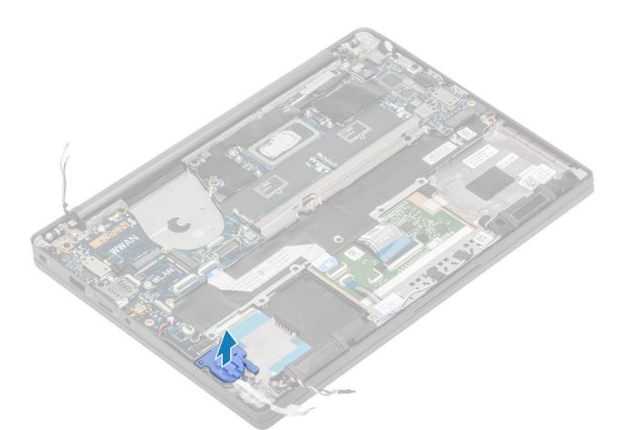
6. Remove the single (M2x3) screw from the display cable bracket [1] and remove it from the system board [2].
