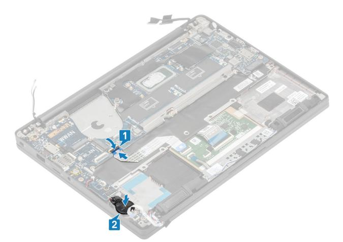
6. Connect the display cable to the camera-touchscreen [1] and the EDP cable connectors [2] to the system board.
