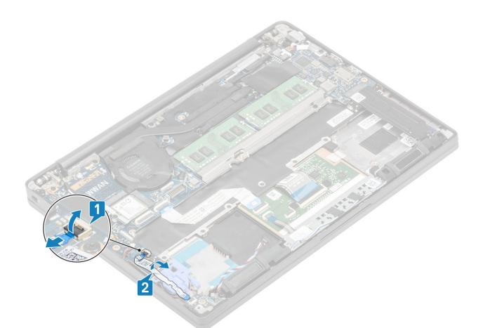
**3.** Remove the single (M2x2.5) screw [1] and remove the LED daughterboard from the palmrest assembly [2].
