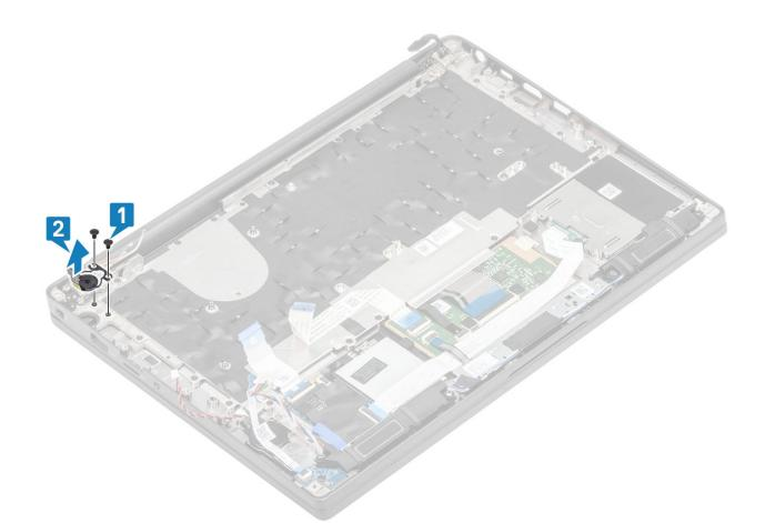
Figure 4. Removing the power-button board with FPR
