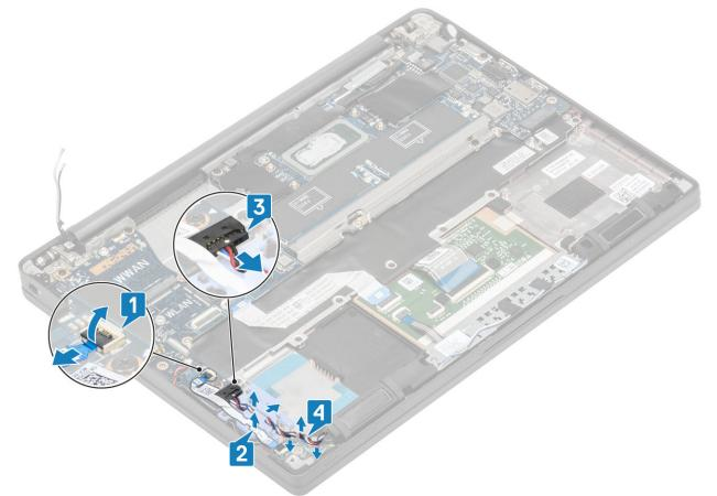
5. Peel off the rubber routing channel from the coin cell.
