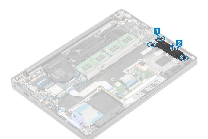
3. Slightly lift and remove the SSD out from its connector on the system board.
