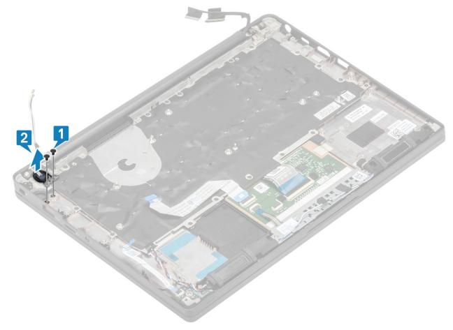
Figure 3. Power-button board without FPR
