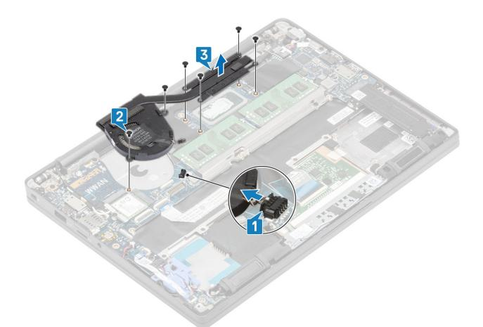
4. Remove the single screw securing the fan to heatsink.
