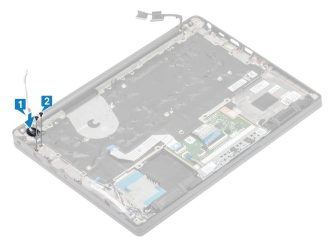
Figure 5. Power-button board - without FPR
