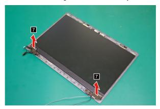
Figure 34. Remove the LCD hinges
