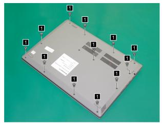
Figure 3. Remove the screws
