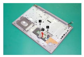
Figure 26. Remove the screws and detach the touchpad
