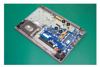
Figure 18. Remove the screws
