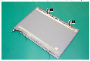
Figure 37. Remove the antenna assembly
