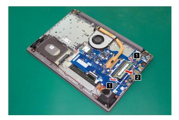
Figure 12. Release the latches and unplug the DIMM
