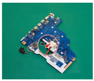
Figure 24. Remove the backup battery
