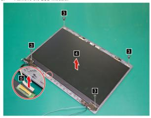
Figure 32. Remove the screws and LCD module connector
