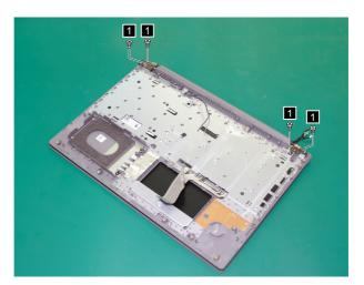
Figure 27. Remove the screws
