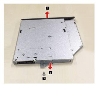
Figure 2. Remove the optical drive bracket and bezel
