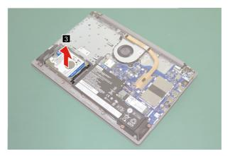
Figure 6. Remove the hard disk drive
