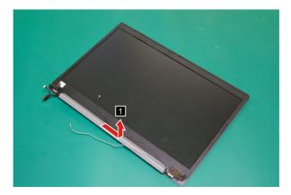
Figure 30. Remove the hinge cap
