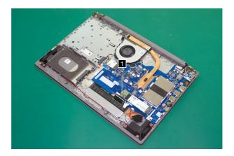
Figure 10. Remove the screw
