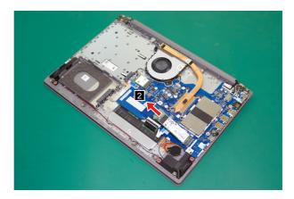
Figure 11. Remove the SSD card
