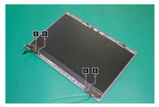
Figure 33. Remove the screws
