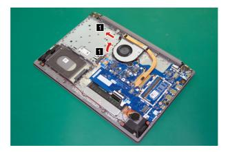
Figure 15. Release the antenna cables
