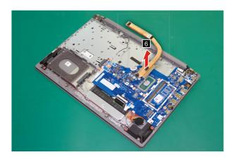
Figure 19. Remove the heat sink
