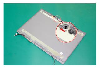
Figure 35. Detach the camera connector
