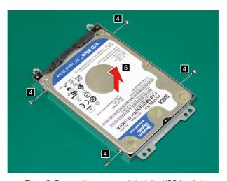
Figure 7. Remove the screws and dtach the HDD bracket
