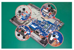
Figure 21. Disconnect the connectors
