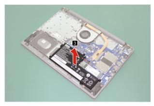
Figure 9. Remove the battery pack
