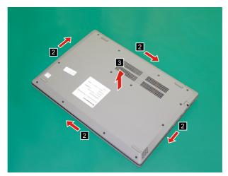
Figure 4. Remove the base cover
