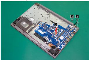
Figure 22. Remove the screws and system board
