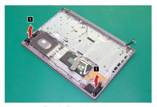
Figure 25. Remove the speakers
