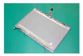
Figure 36. Remove the integrated camera
