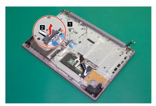
Figure 23. Remove the ODD transfer board
