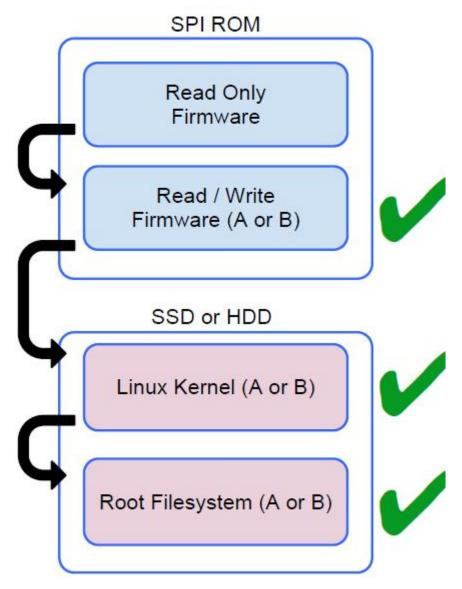
Read Only firmware verifies the integrity of Read/Write (R/W) firmware. R/W firmware verifies the active Linux kernel. During run time, the kernel verifies each block read from disk.
