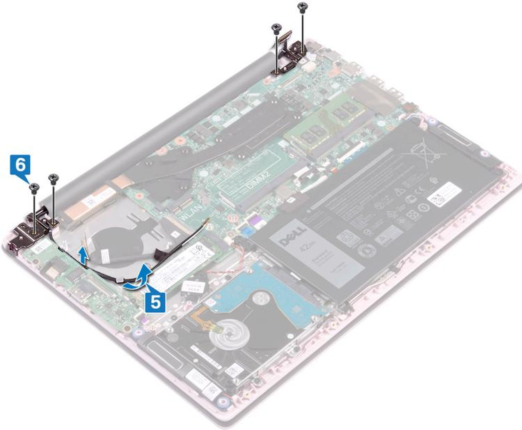
7 Open the display at an angle of 90 degrees.
