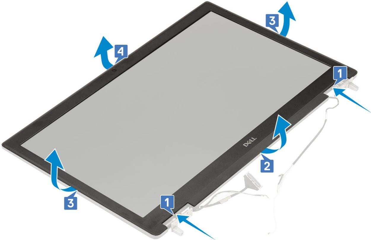
**NOTE:** The display bezel shipped with a non-touch display is a disposable part and should be replaced with a new display bezel anytime it is removed from the system.
