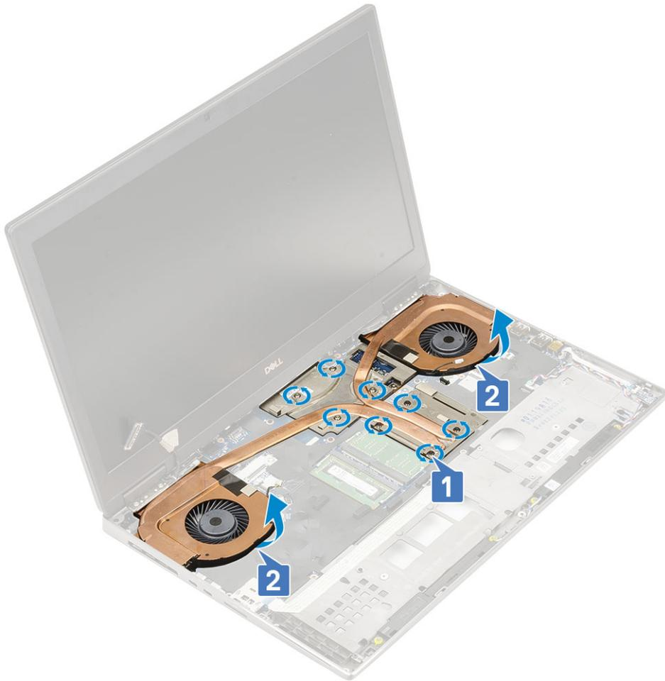
h Slide and remove the heat sink assembly from the system.
