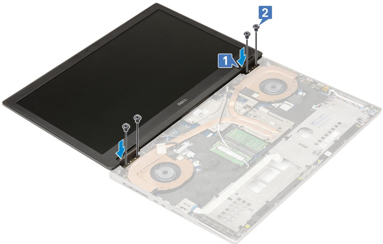
g Close the display assembly and replace the 2 (M2.5x6.0) screws at the rear of the system to secure the display assembly in place.
