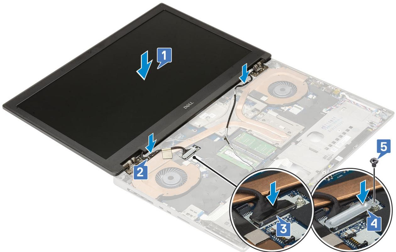
f Align the display hinge caps and replace the 4 (M2.5x4.0) screws to secure the display hinge caps to the system [1, 2].
