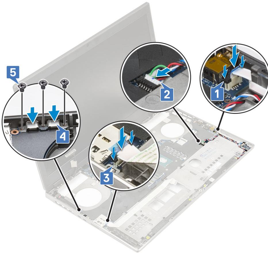
f Connect the power connector cable and battery cable to the connectors on the system board [1, 2].
