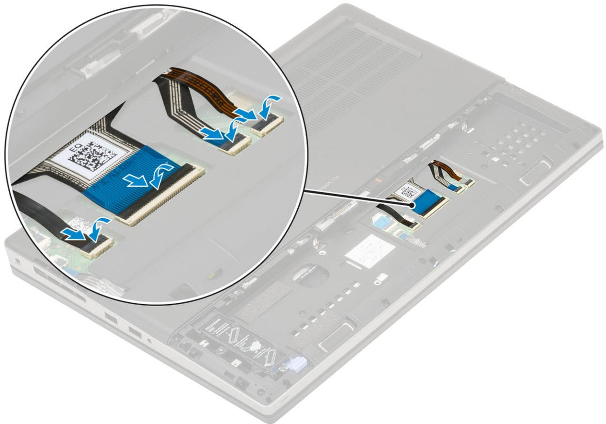
**NOTE:** Ensure that you fold the keyboard data cable in perfect alignment.
