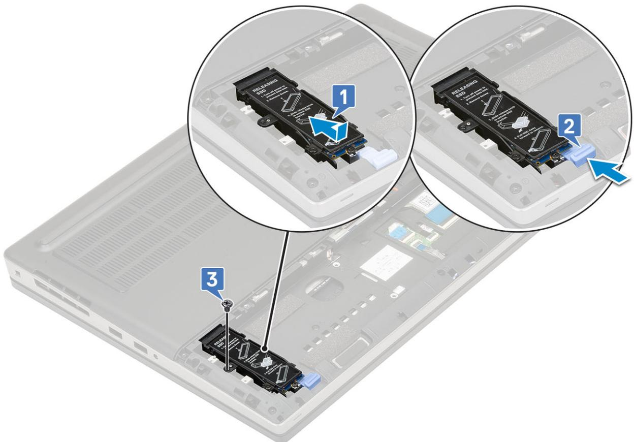
2 To install the M.2 SSD module (Slot 3, 5 or 6):
