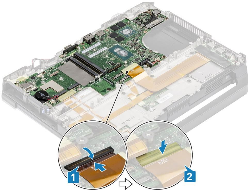
9. Connect the rear I/O board FPC cable [1] and secure it using a piece of tape [2].
