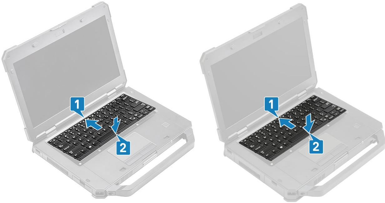
6. Install the six 'M2.5\*5' screws on the keyboard to secure it to the computer.
