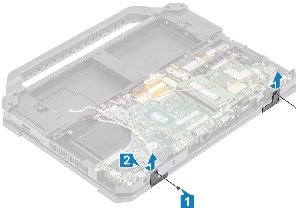
4. Press the latch [1] and open the LCD lid [2].
