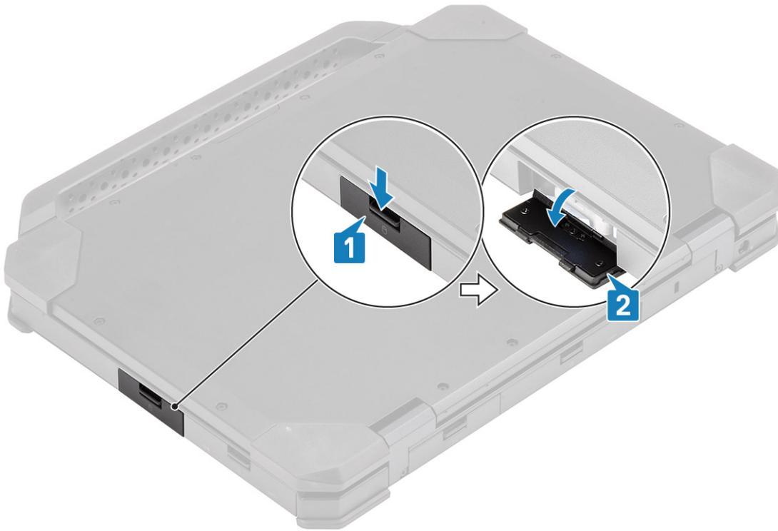
2. Withdraw the stylus out of the slot.
