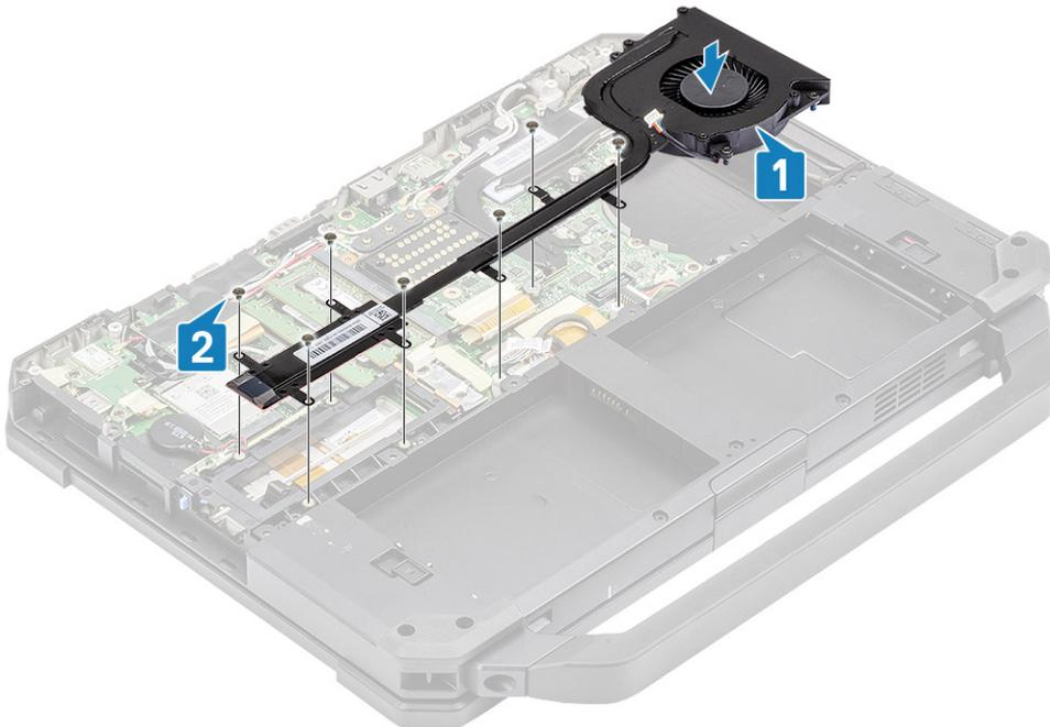
3. Tighten the three 'M2\*3' screws on the fan case [1] and connect the fan cable [2].
