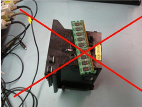
**Acceptable — DIMM separated from the insulator part**
