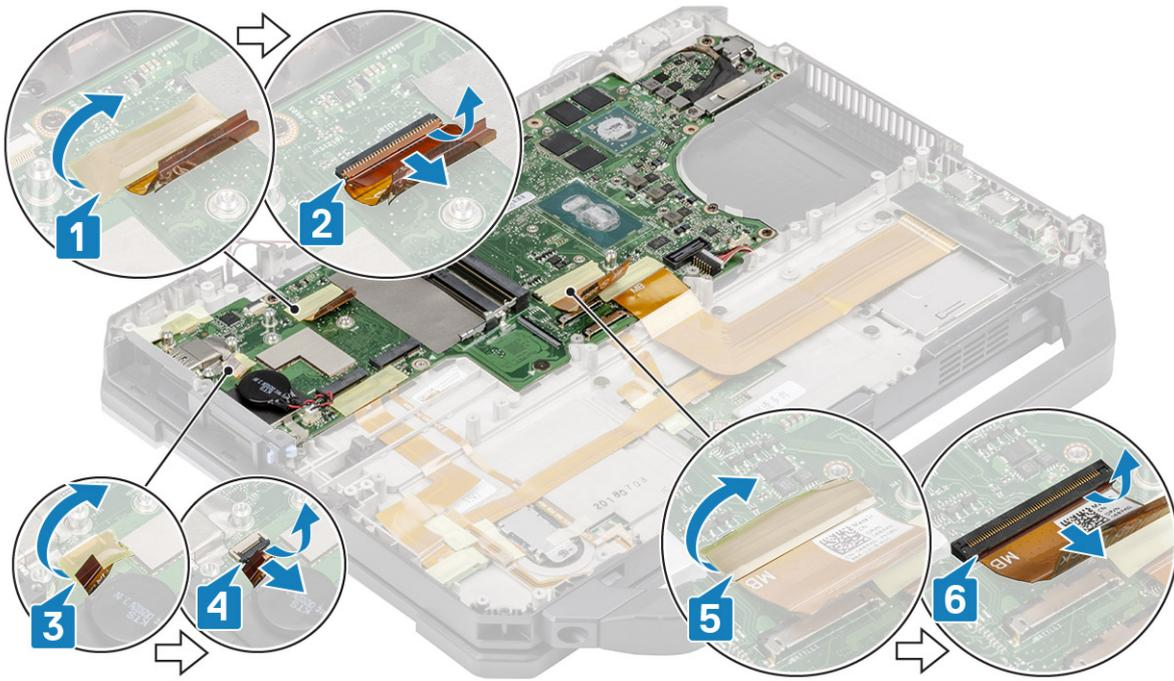
7. Peel off the tape [1] and disconnect the left I/O board FPC connector [2] from the system board.
