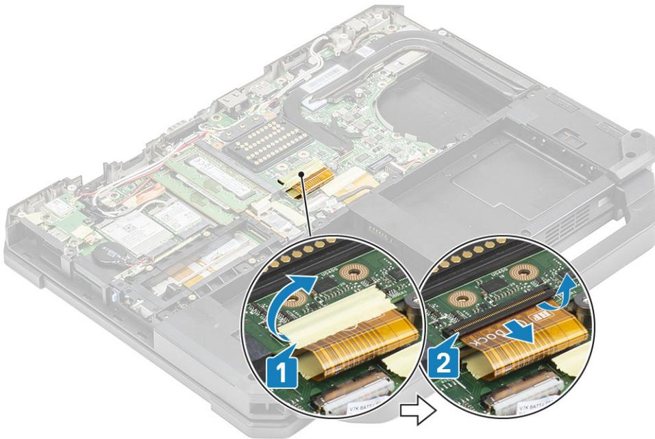
4. Disconnect the antennae cables from RF passthrough connectors [1] and unroute the antennae cables [2] from the routing channels on the dock assembly.
