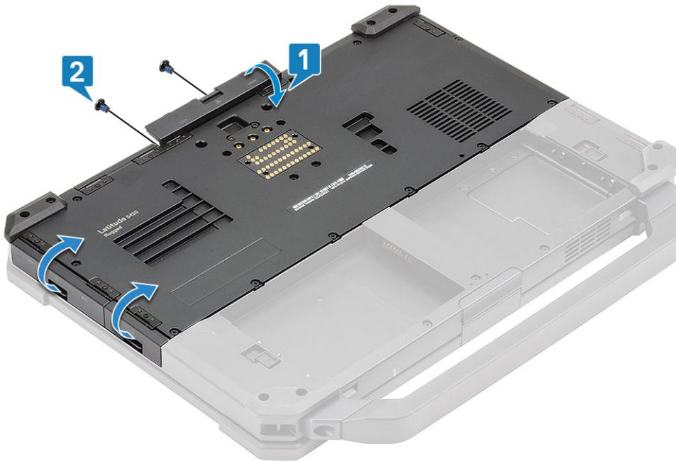
4. Remove the 17 'M2.5\*5' screws on the bottom chassis cover [1] and remove the bottom chassis cover [2] from the computer.
