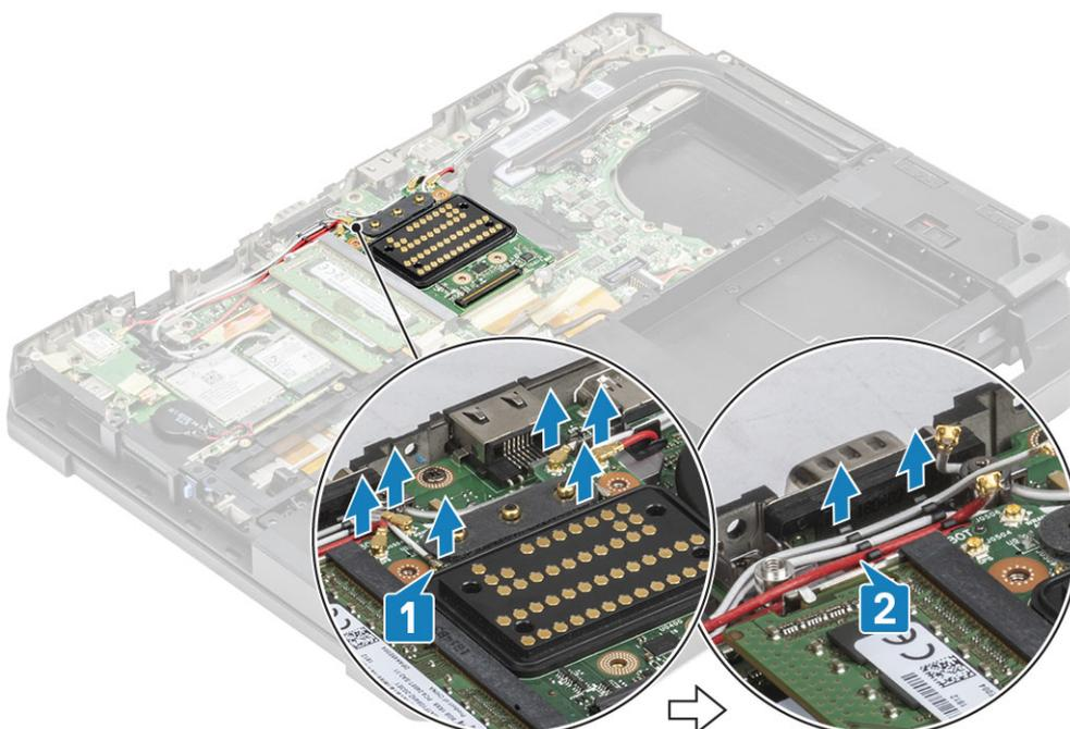
5. Remove the two 'M2.5\*5' screws [1] and separate the docking board assembly from the chassis [2].
