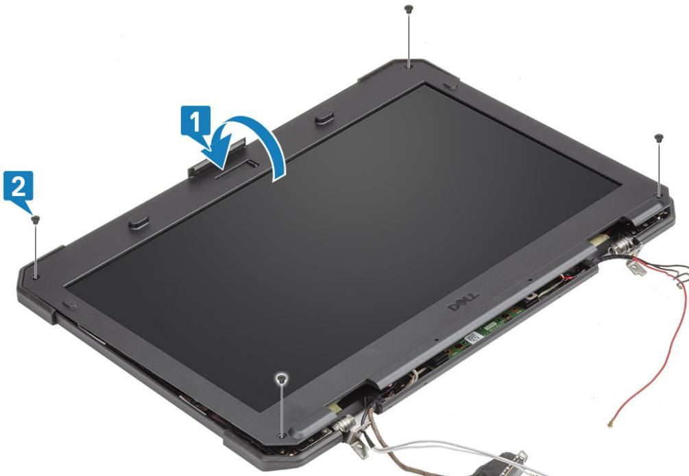
5. Install the 12 'M2.5' screws to secure the back cover to the LCD with bezel assembly.
