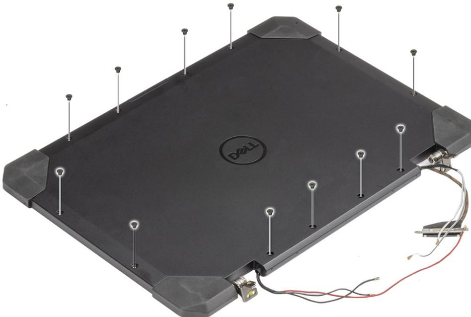
4. Remove the four 'M2.5' epoxy screws securing the bezel to the back cover [1] and pry at bottom edge to separate the two subassemblies [2].
