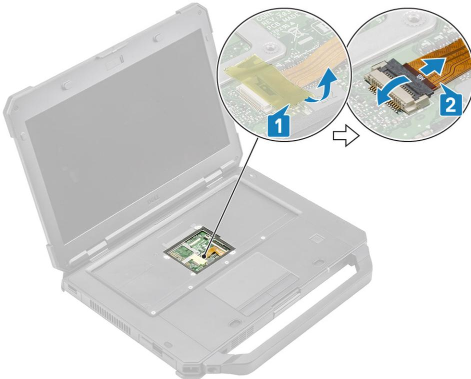
4. Peel off the tape [1] and remove the rear I/O board FPC cable [2] from the system board.
