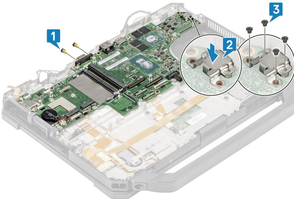
4. Install the EDP cable [1] and place the metal bracket [2] over the EDP connector on the system board.
