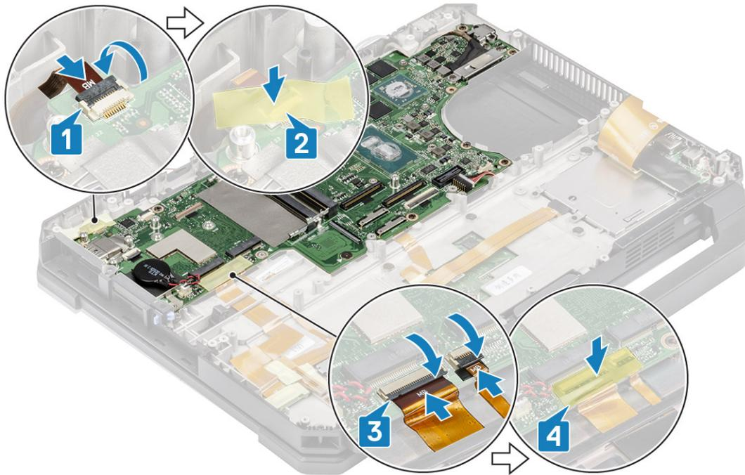
8. Connect the left I/O board FPC cable [1] and secure it using a piece of tape [2].
