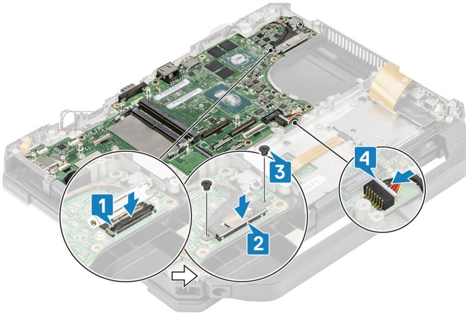
6. Connect the power button cable [1] and secure it using a piece of tape [2].
