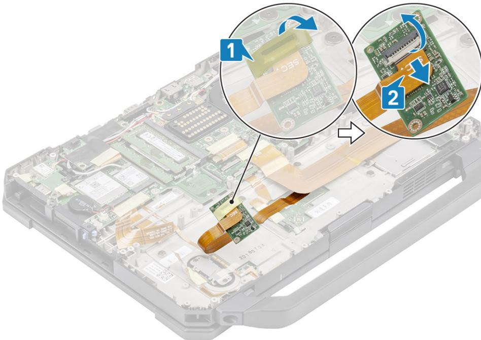
7. Loosen the four 'M2\*3' screws [1] and remove the smart card [2] reader from the computer.
