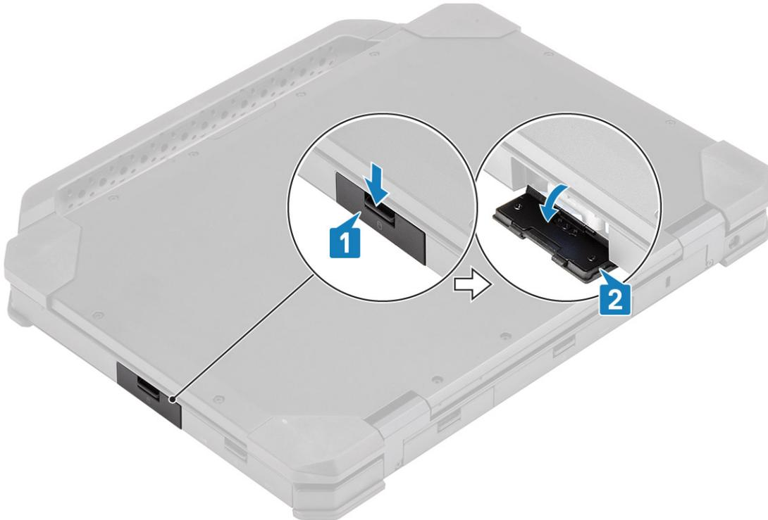
4. Release the SSD carrier by sliding the blue hard drive release latch [1] towards right.
