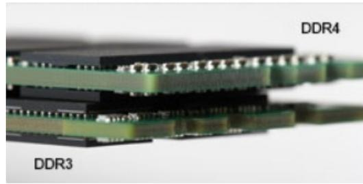
**Figure 5. Thickness difference**
