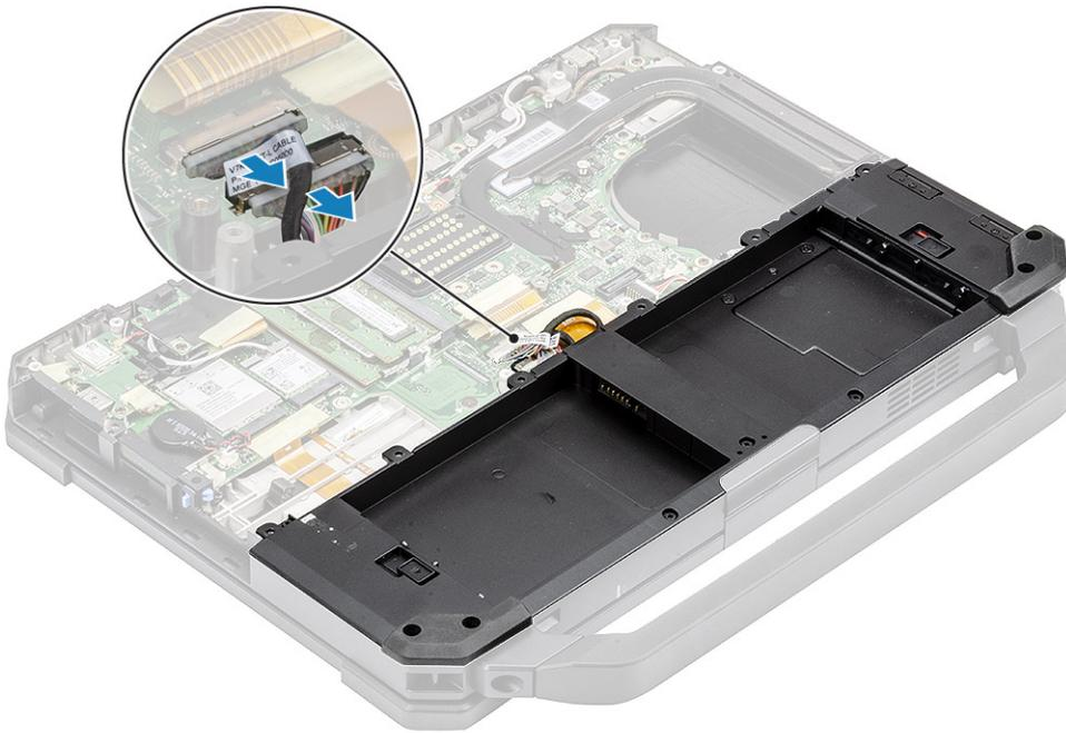
4. Remove the five 'M2.5\*5' [1] and nine 'M2.5\*3' [2] screws securing the battery bay to chassis and lift to separate the battery bay [3] from the computer.
