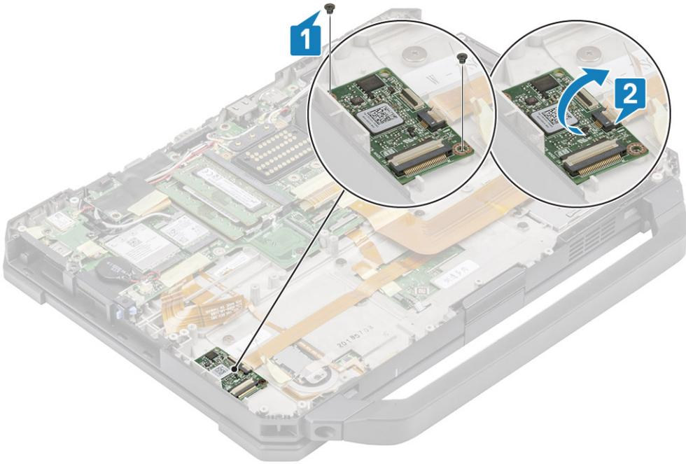
6. Remove the tape [1] and disconnect the Smartcard Reader FPC connector [2] from the USH board.
