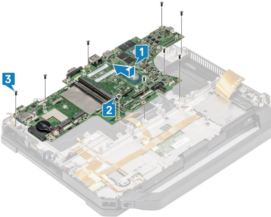
2. Install the two cap screws on the serial port of the system board [1].
