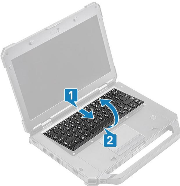
5. Remove the four 'M2\*3' screws [1] on the keyboard cover and remove it from the computer [2].
