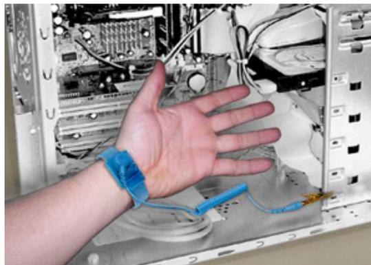
Figure 8. Bonding Properly
