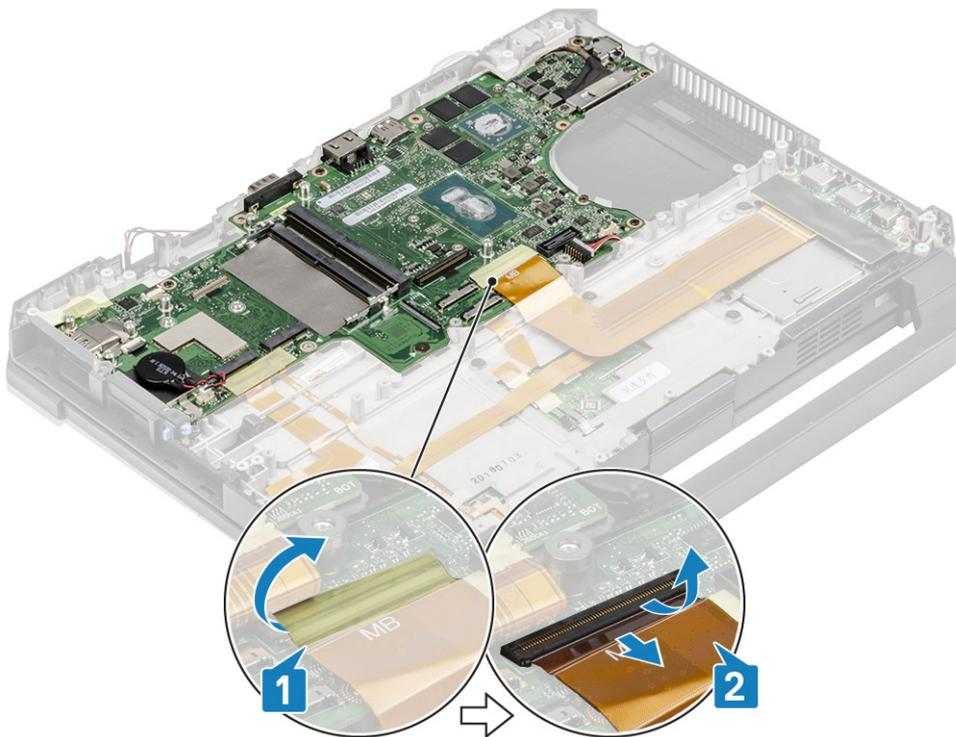
8. Peel off the tape [1] and disconnect the power button cable [2].
