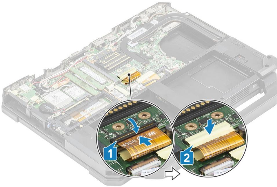
3. Secure the antennae cables along the routing channels [1] and connect the antennae cables on RF passthrough connectors [2].
