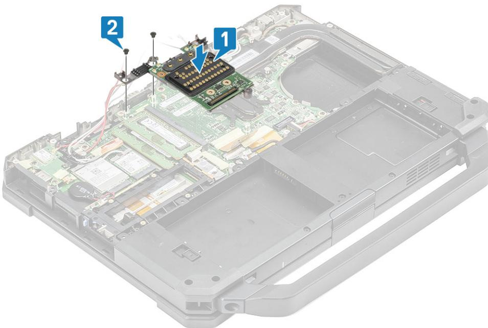
2. Connect the dock FPC [1] and secure it using a piece of tape [2].
