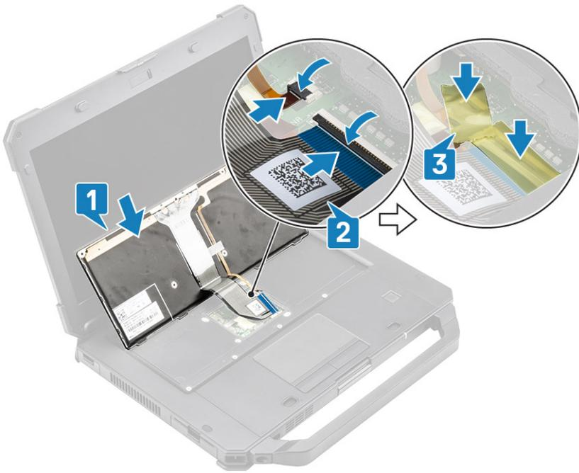
3. Install the keyboard cover [1] and tighten the four 'M2\*3' screws [2] to secure it to the chassis.
