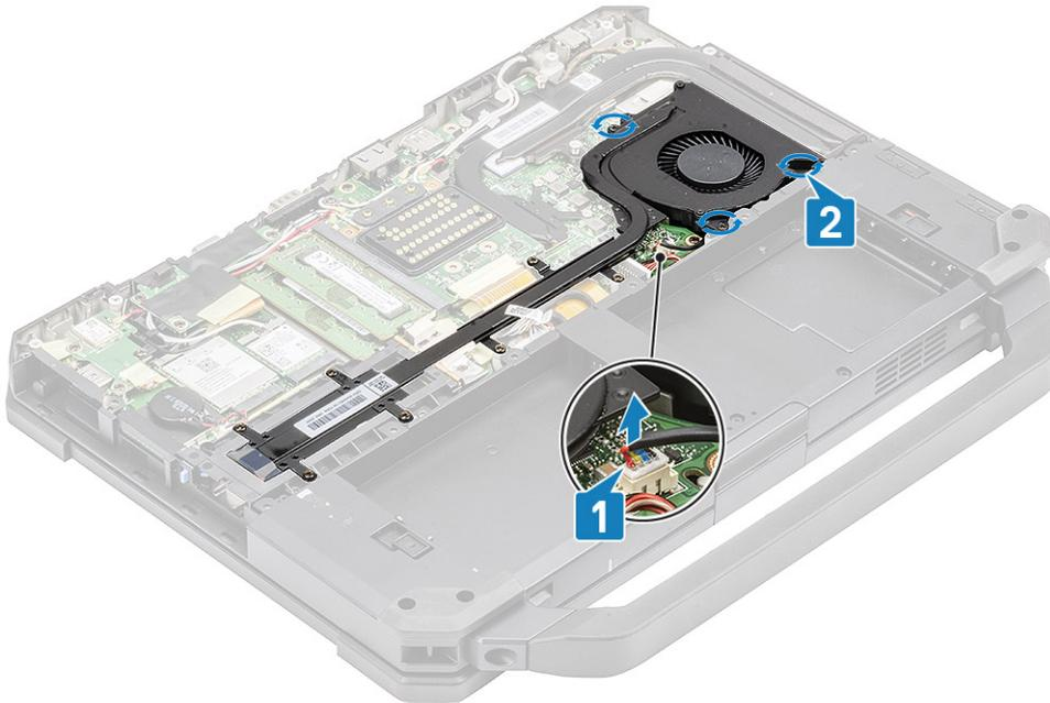
4. Loosen the seven 'M2.5\*5' screws [1] from heat sink pipe and remove the PCIe heatsink assembly from the computer [2].
