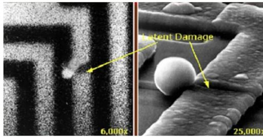
**Figure 9. Intermittent (Latent) Damage to a Wiring Trace**
