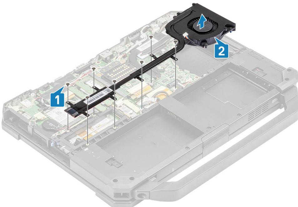
5. Remove the four M2\*3 screws [1] to separate the heatsink from the fan [2].
