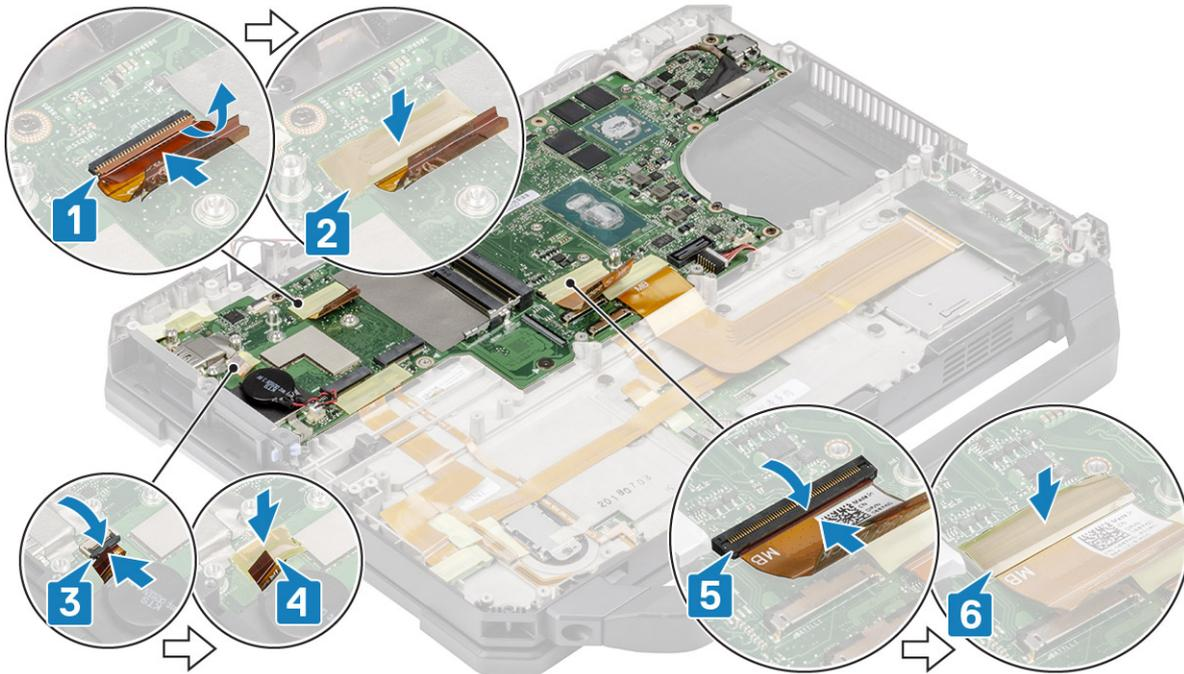
12. Connect the touch pad connectors to the system board [1] and secure it using a piece of tape [2].
