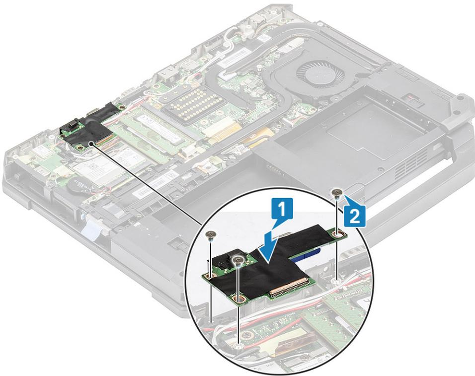
3. Tighten the two cap screws on the serial port [1] in the rear I/O space.
