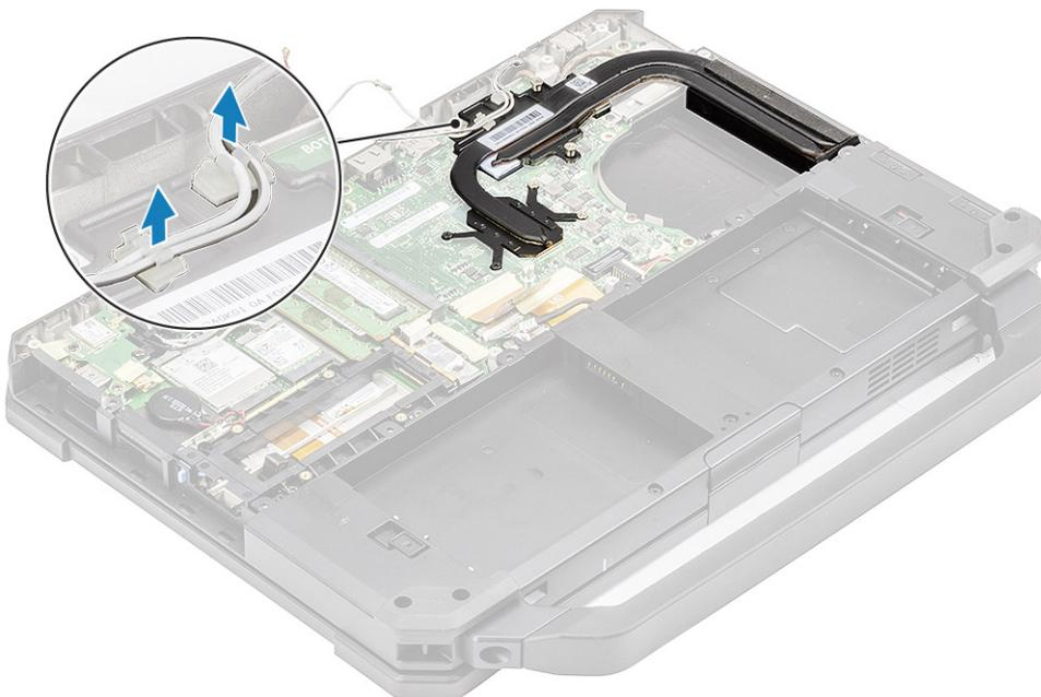
4. Remove the five 'M2.5\*5' screws [1] and two 'M1.6\*5' [2] screw from the thermal module.
