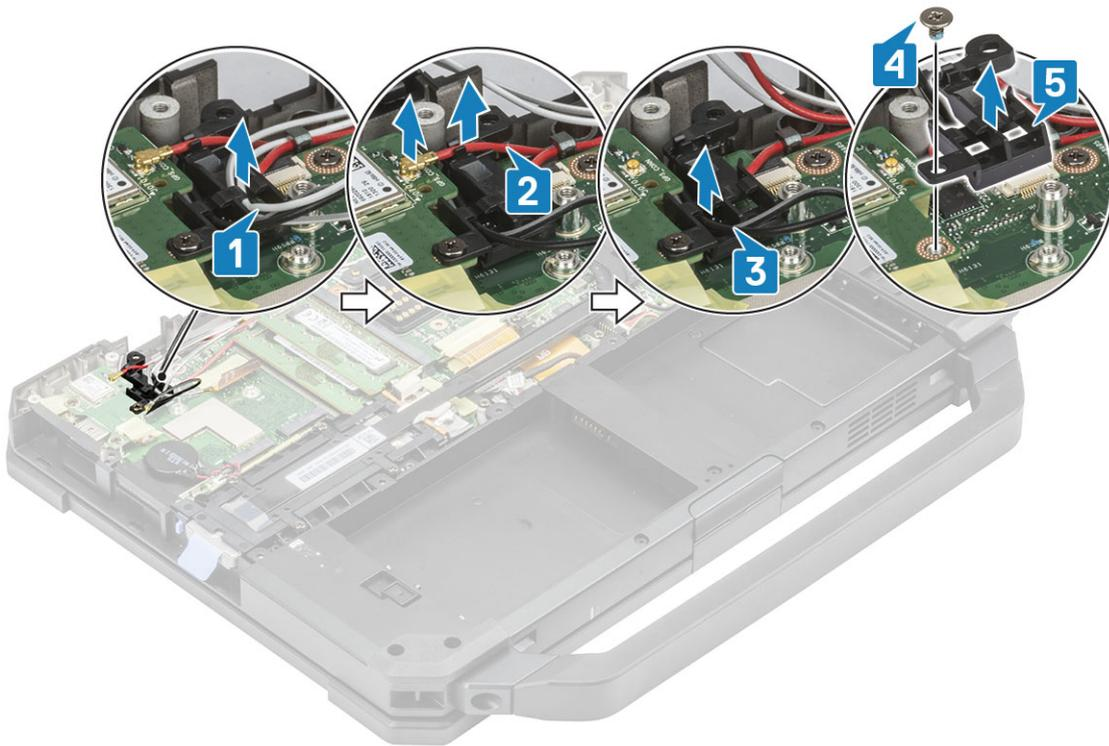
5. Peel off the inductive tape on the GPS FPC connector [1] and disconnect the GPS FPC connector [2] from GPS module.
