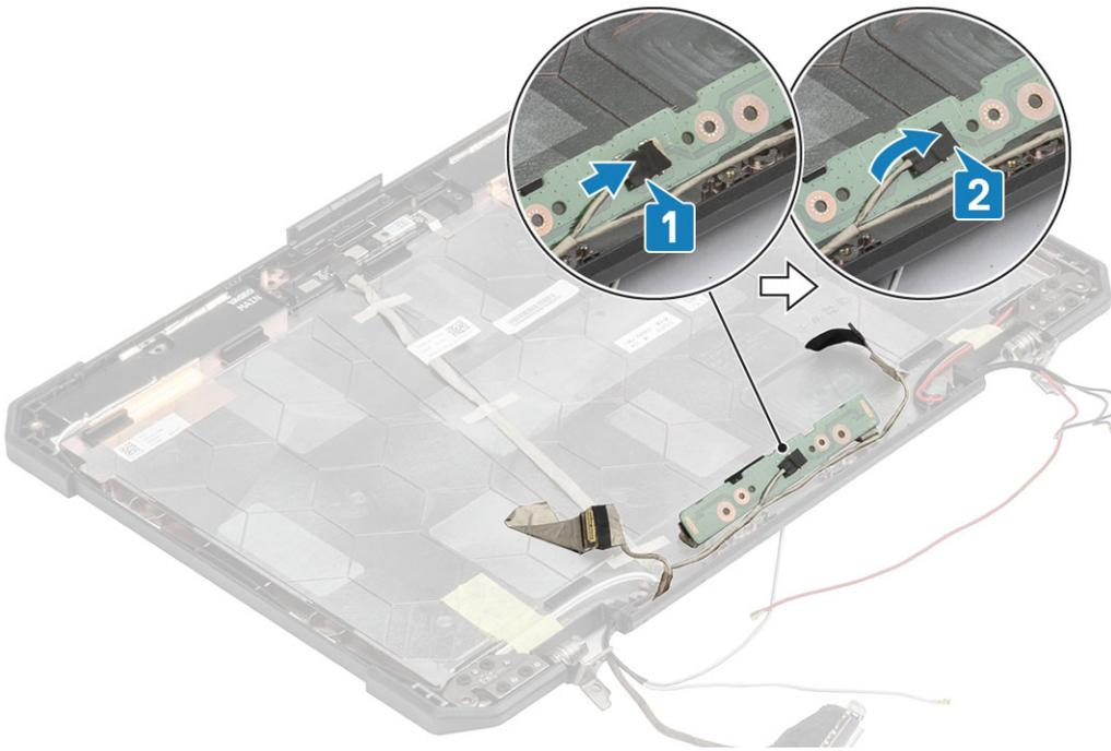
2. Turn over the microphone daughterboard on the back cover [1] and tighten the two 'M2\*3' screws [2].
