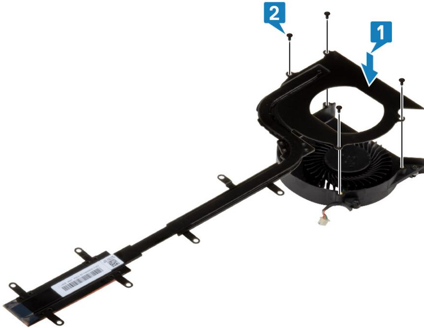
2. Install the PCIe heatsink assembly [1] in the computer and install the seven 'M2.5\*5' screws on heat sink pipe [2].
