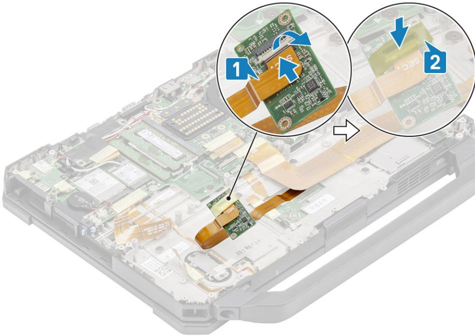
3. Install the two 'M2\*3' screws [1] and turn over the USB board to secure it to the chassis [2].
