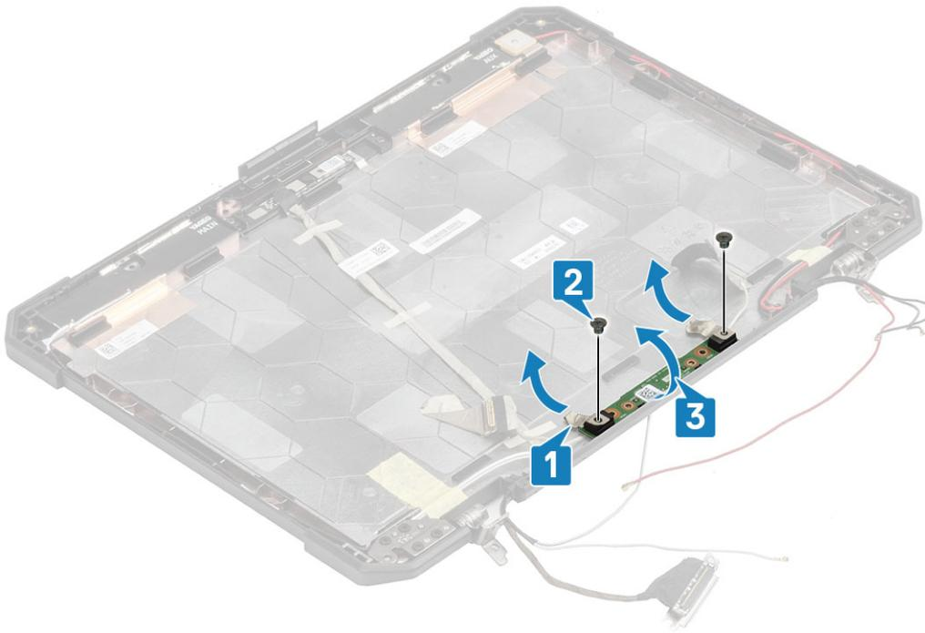
4. Peel off the insulation tape [1] and disconnect the EDP cable connectors [2].
