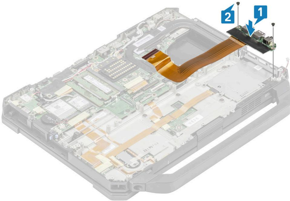
2. Connect the FPC to the system board [1] and secure it using a piece of insulation tape [2].
