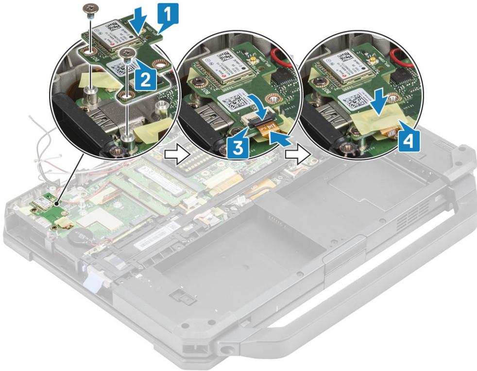
3. Install the RF bracket [1] on the system board and secure it using the single 'M2.5\*5' screw [2].
