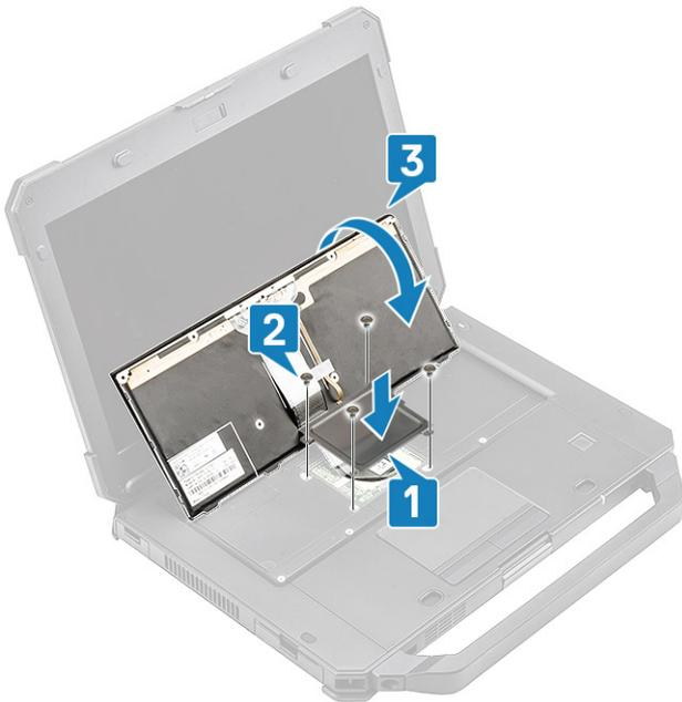
5. Slide the keyboard towards LCD [1] to align it to screw holes [2].
