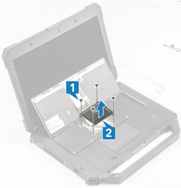
6. Peel-off the tape on the keyboard and back-light FPC [1] and disconnect it from the system board [2].
