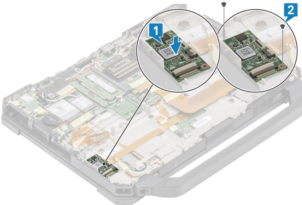
4. Connect the fingerprint reader connector [1] and secure it with a piece of tape [2].
