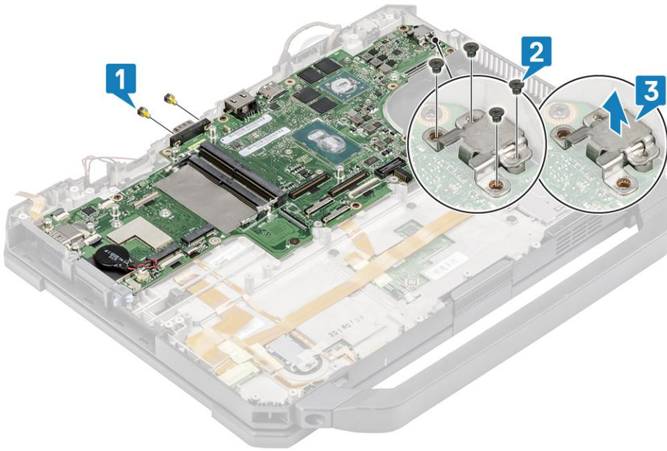
14. Remove the eight 'M2.5\*5' screws [1] and single 'M2\*3' screw [2] on the system board and remove the system board from the chassis [3].
