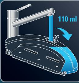
**EN** Open the water tank of the mop support and fill it with 110ml of water.
