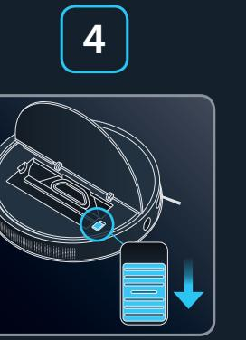
**EN** Toggle the on/off switch to "on".
