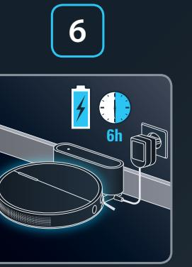
**EN** Wait 6 hours for the robot to be fully charged.
