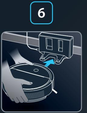
**EN** Position your robot on its docking station until the battery symbols are blinking.
