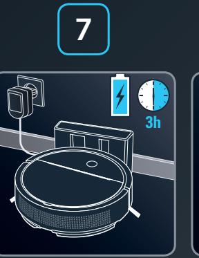
**EN** Wait 3 hours for the robot to be fully charged.
