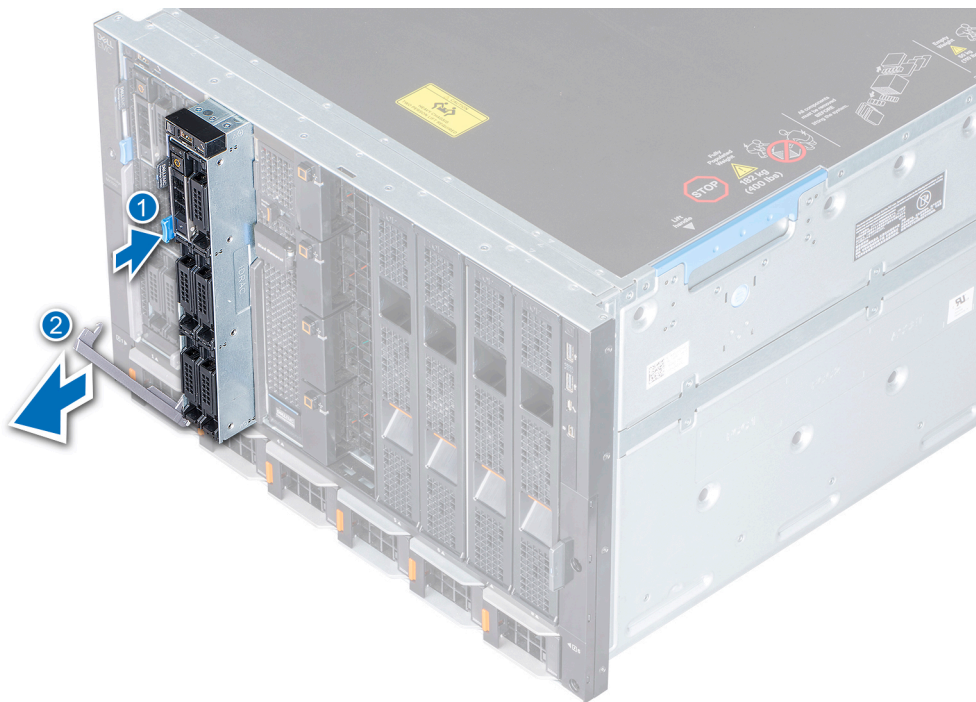
Figure 12. Removing the sled from enclosure
