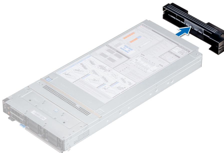
Figure 14. Removing the I/O connector cover from sled
