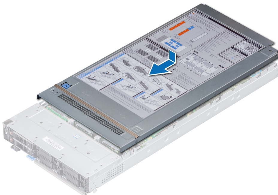
Figure 17. Installing system cover
