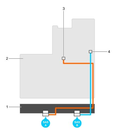
Figure 1. Cabling the S140 controller
