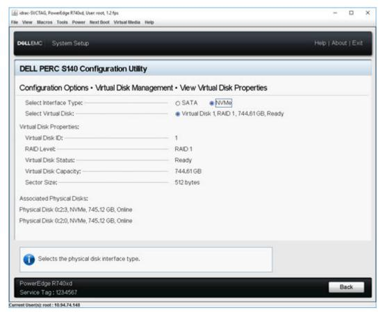
Figure 5. Virtual Disk Properties Screen
