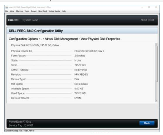
Figure 6. Physical Disk Properties Screen
