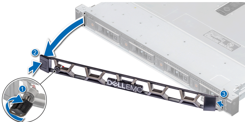
Figure 13. Removing the optional front bezel
