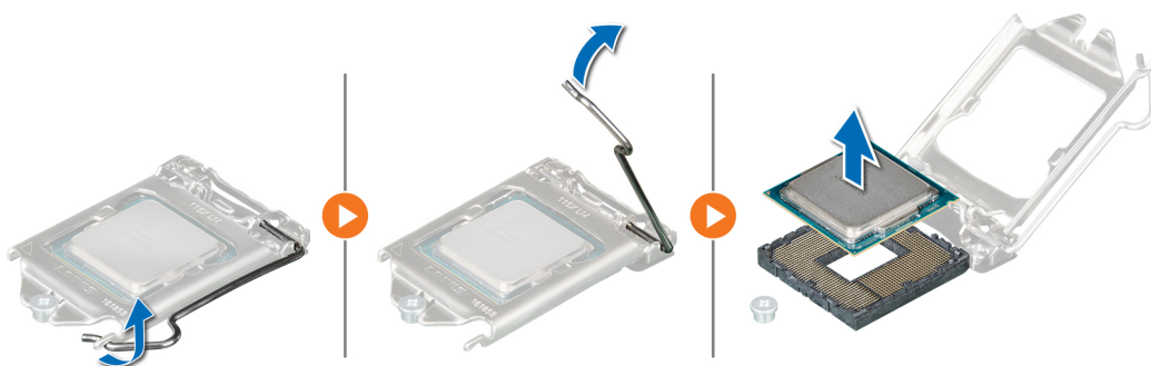
Figure 52. Removing the processor
