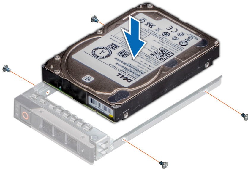
Figure 28. Installing a drive into the drive carrier
