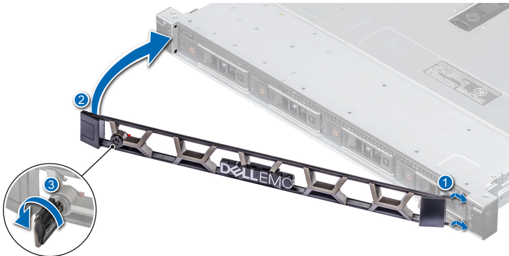
Figure 14. Installing the optional front bezel
