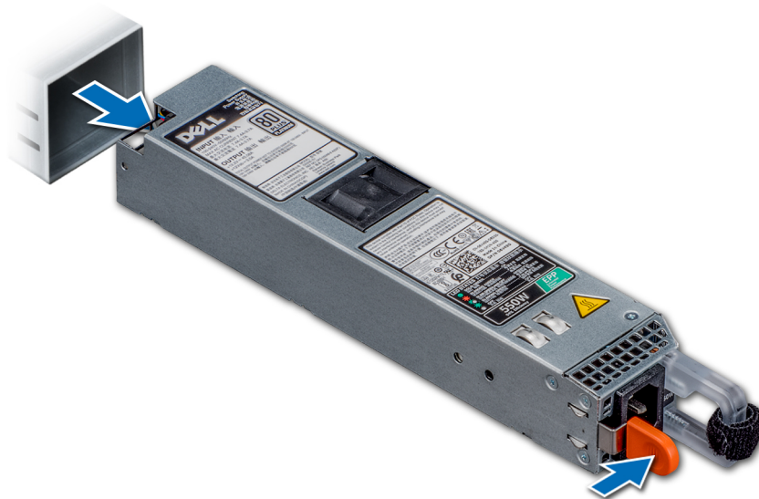
Figure 70. Removing a power supply unit
