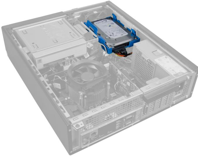
3. Remove the data cable and the power cable from the back of the hard drive.
