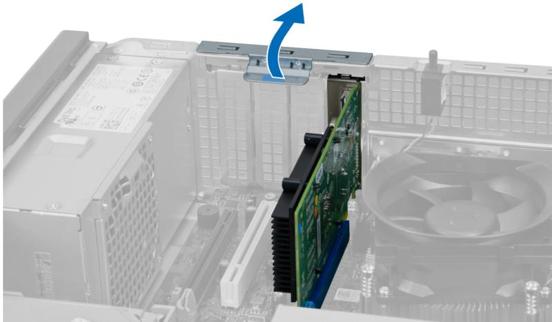
4. Press the release lever away from the expansion card and ease the card up and out of its connector.
