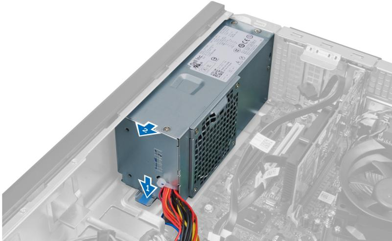
10. Lift the power supply out of the computer.
