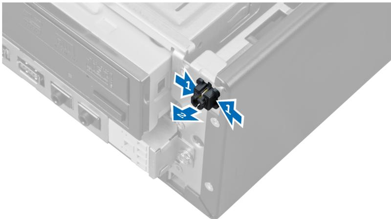
5. Slide the power-switch cable out through the front of the computer.
