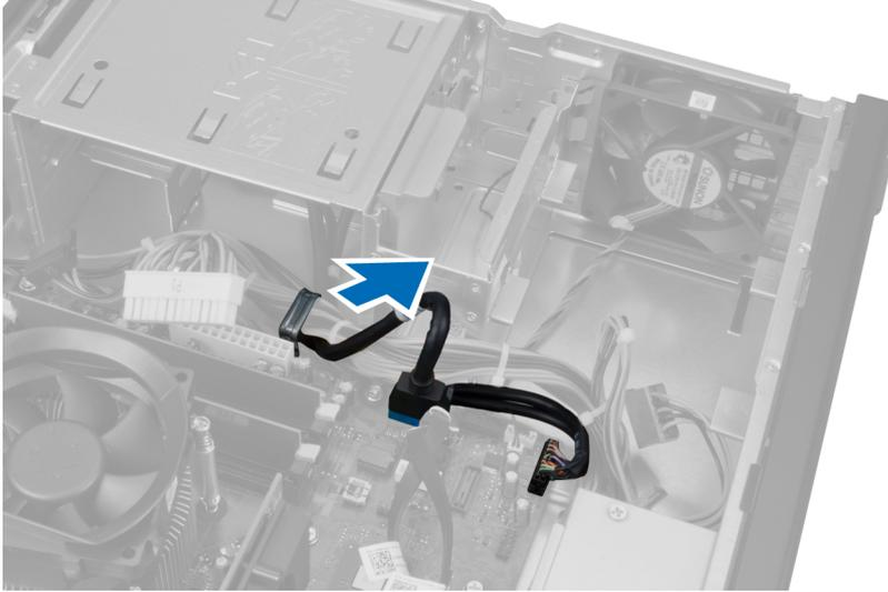
5. Press the metal clip and pull upwards to disconnect the USB 3.0 connector.
