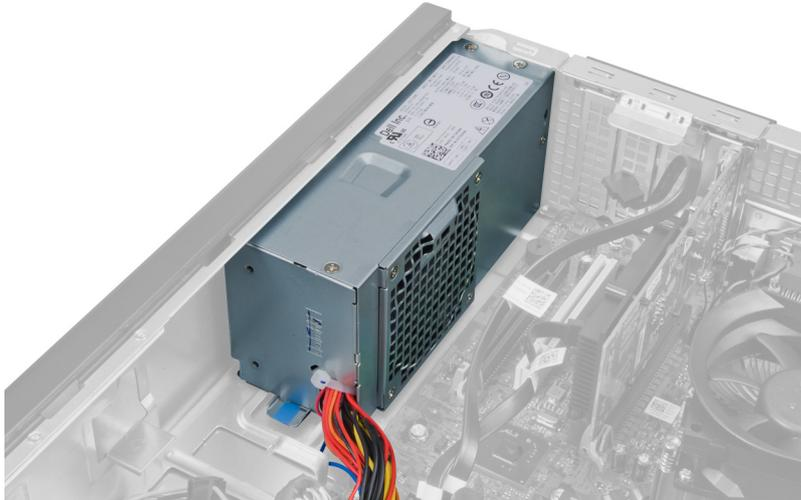
3. Press the plastic clip and disconnect the 4-pin power cable from the system board.
