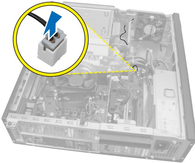
4. Release the thermal-sensor cable from the chassis clips.
