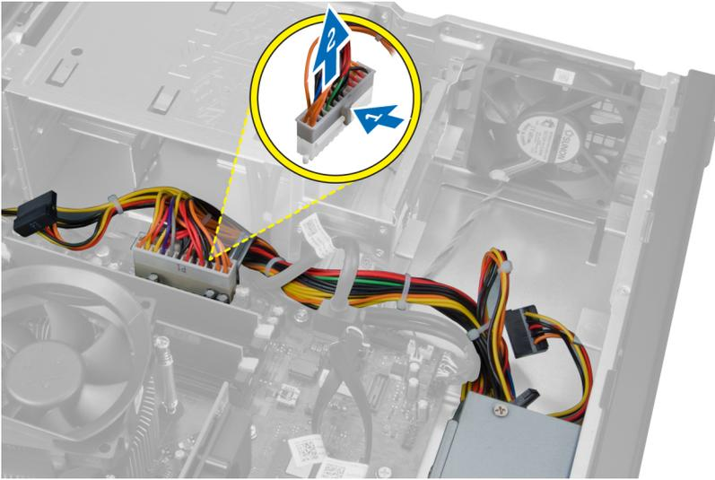
6. Unthread the 24-pin power cable from the chassis clip.
