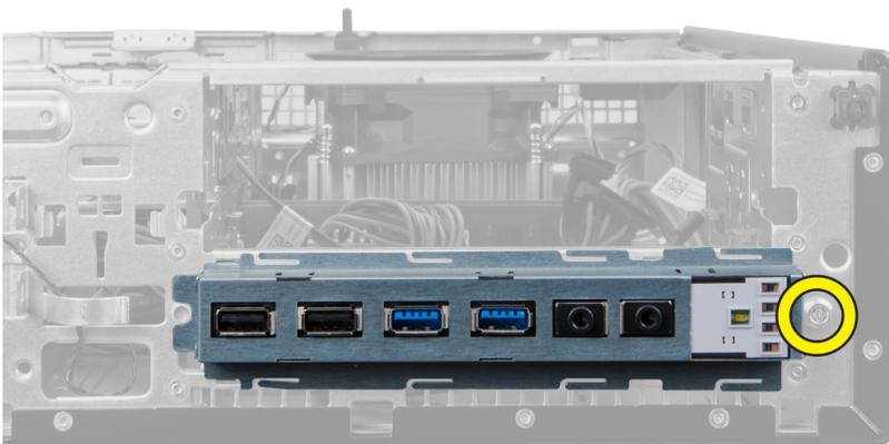
7. Slide the I/O panel towards the left of the computer to release it and pull the I/O panel along with its cable out of the computer.
