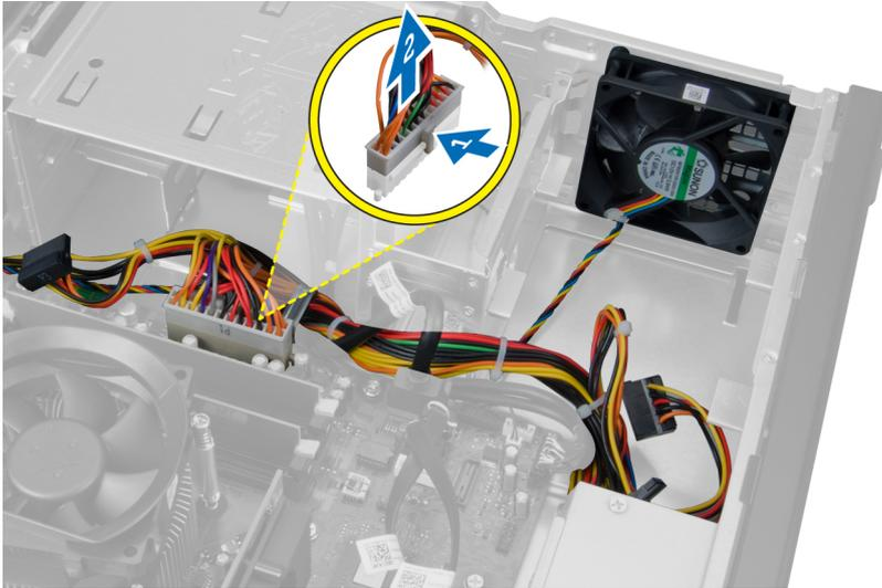
7. Unthread the power cables from the chassis clip.
