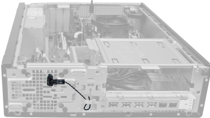
3. Disconnect the thermal-sensor cable from the system board.
