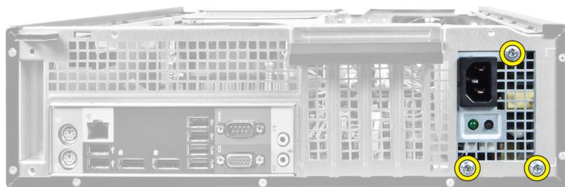
9. Push in on the blue release tab beside the power supply, and slide the power supply towards the front of the computer.
