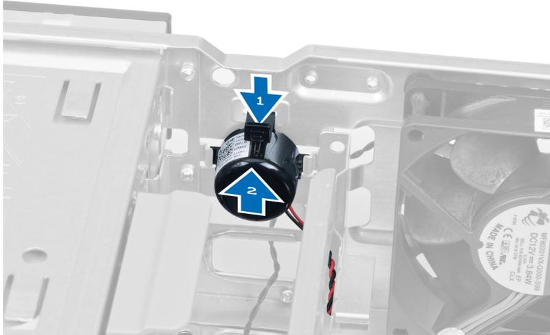
4. Press down the speaker-securing tab and slide the speaker upwards to remove it.
