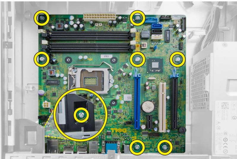
5. Slide and remove the system board from the chassis.
