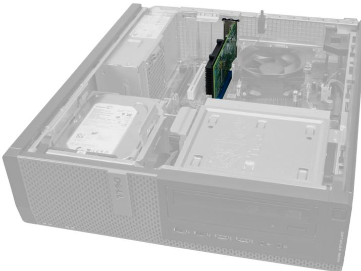
3. Lift the release tab on the card-retention latch upward.
