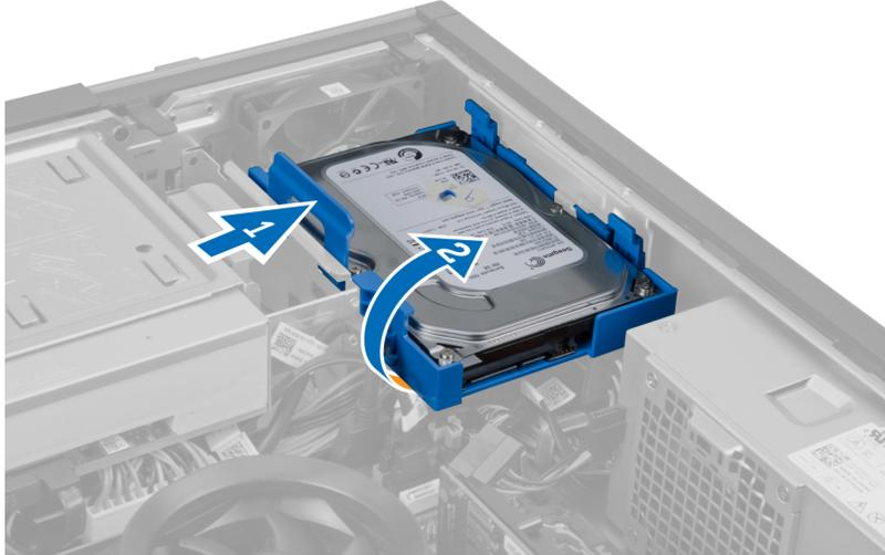
5. Flex the hard drive bracket and then remove the hard drive from the bracket.
