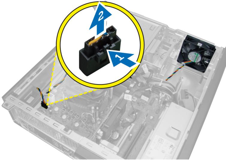
4. Unthread the system-fan cable from the chassis clip.
