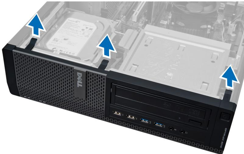
4. Rotate the front panel away from the chassis to release the hooks on the opposite edge of the panel.
