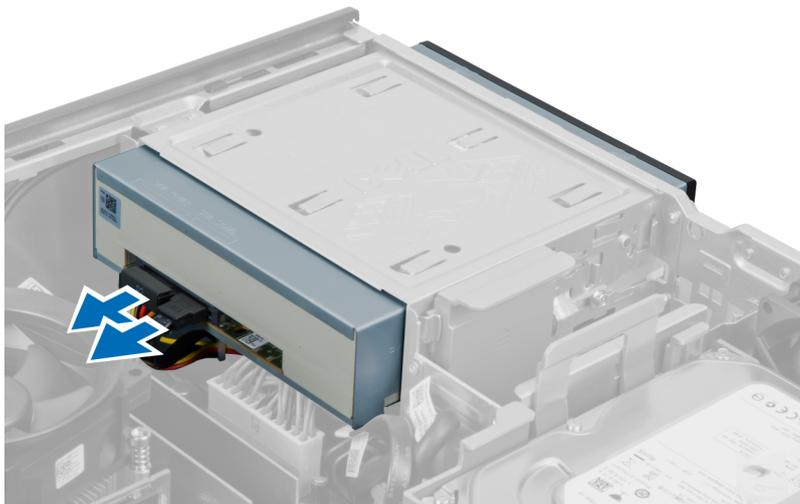
4. Lift up the optical-drive latch and then slide the optical drive towards the front of the computer.
