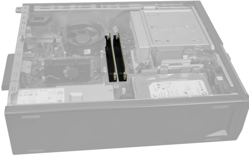
3. Press down on the memory retaining tabs on each side of the memory modules, and lift the memory modules out of the connectors on the system board.
