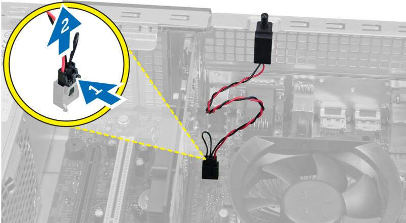
4. Slide the intrusion switch outward and remove it from the chassis.
