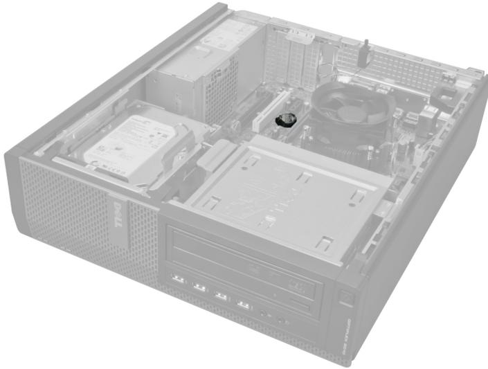
3. Carefully press the release latch away from the battery. The battery pops out from the socket, lift the coin-cell battery out of the computer.
