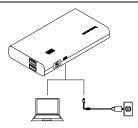
To charge the power bank, connect the power bank to ac power or your computer. **Note:** If the power bank is turned off due to short-circuit protection, charge the power bank to activate it.
