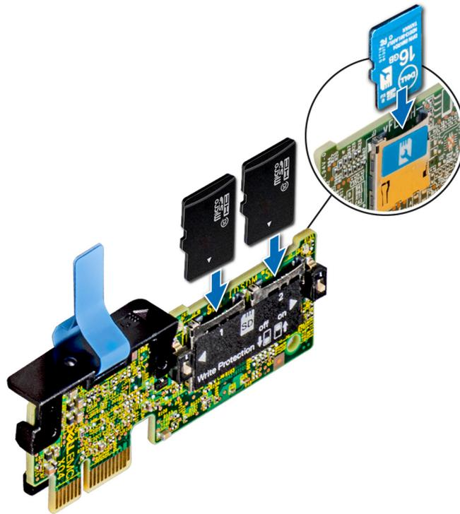
Figure 59. Installing the MicroSD card
