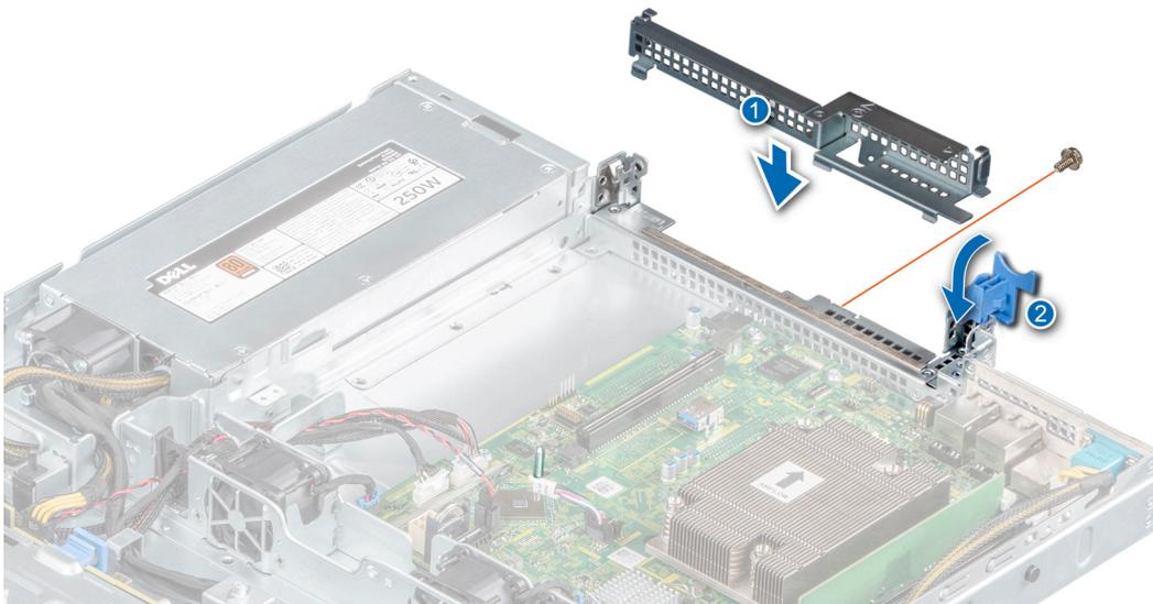
**Figure 40. Installing the expansion card riser filler**
