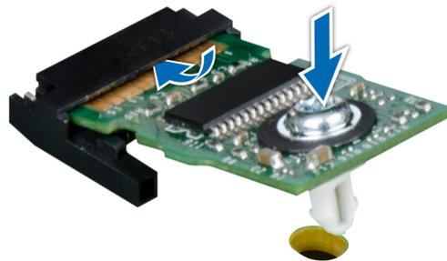
**Figure 74. Installing the TPM**
