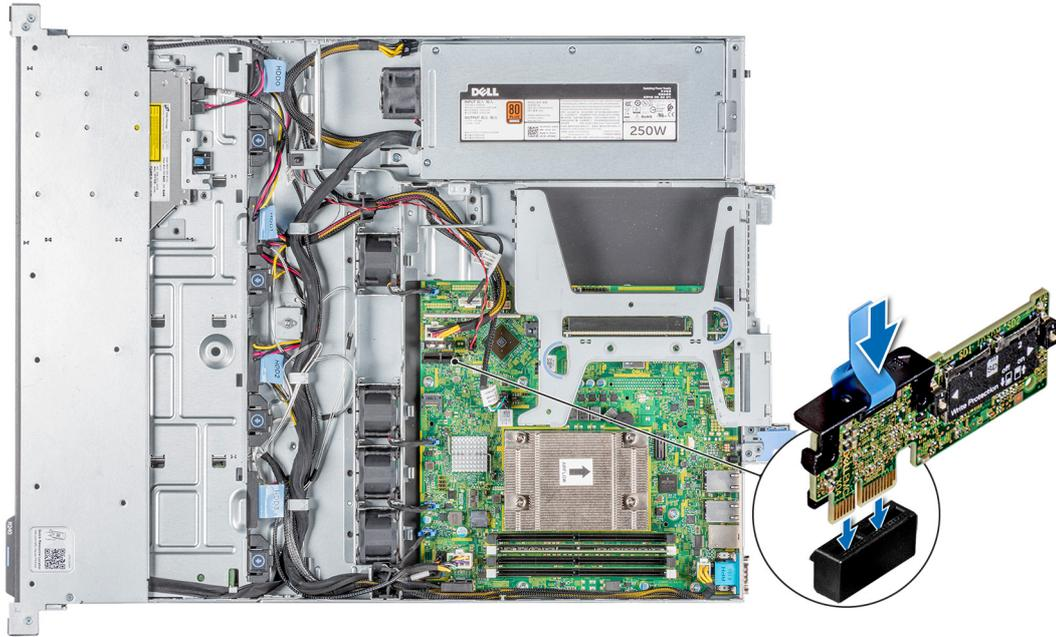
**Figure 57. Installing the optional IDSDM or vFlash card**
