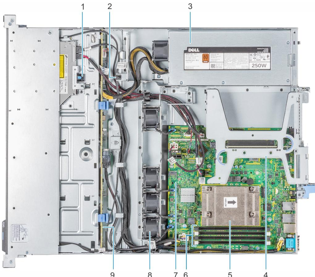
**Figure 6. Inside the system - 4 x 3.5-inch drive system**
