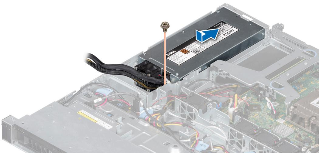
**Figure 70. Installing a cabled power supply unit**
