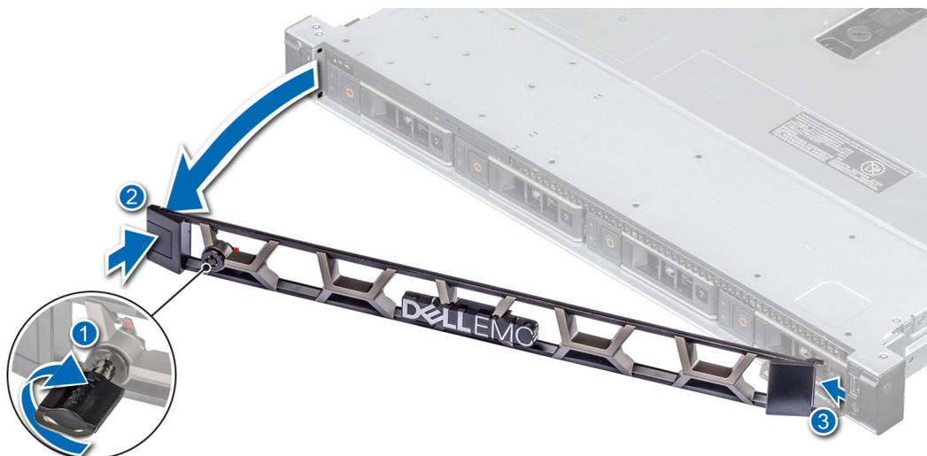
Figure 9. Removing the front bezel
