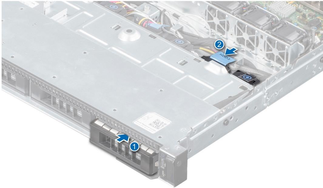
**Figure 30. Installing a cabled drive**
