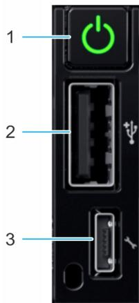
**Figure 4. Right control panel view**
