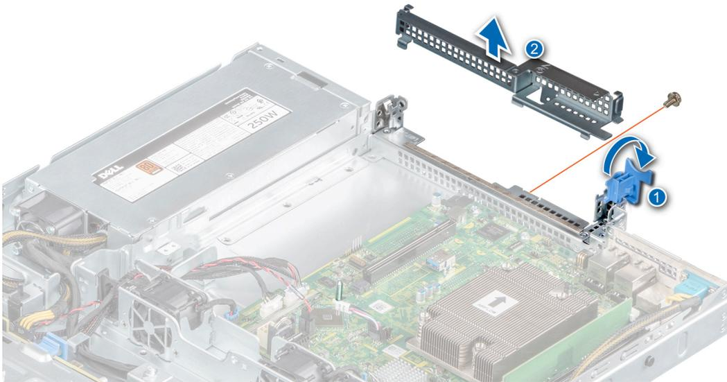
**Figure 41. Removing the expansion card riser filler**
