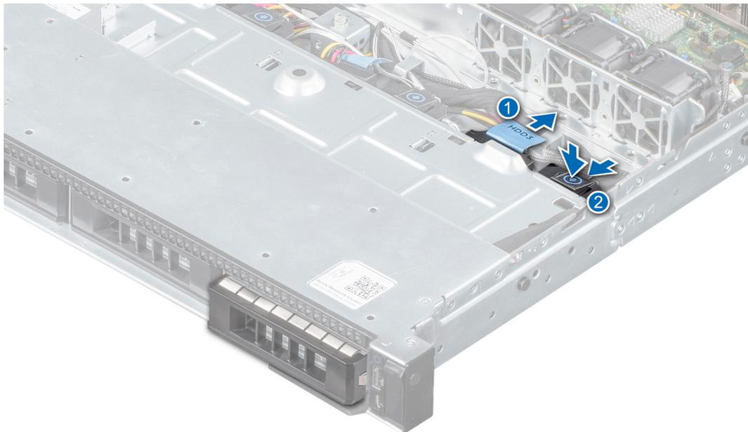
Figure 29. Removing a cabled drive
