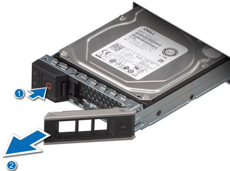
Figure 21. Removing a hot-swappable drive
