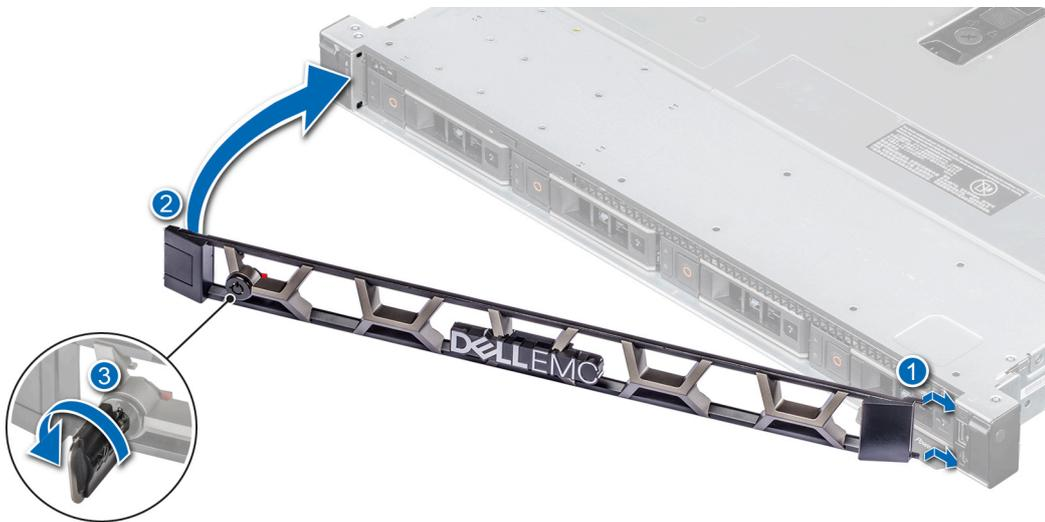
Figure 10. Installing the front bezel
