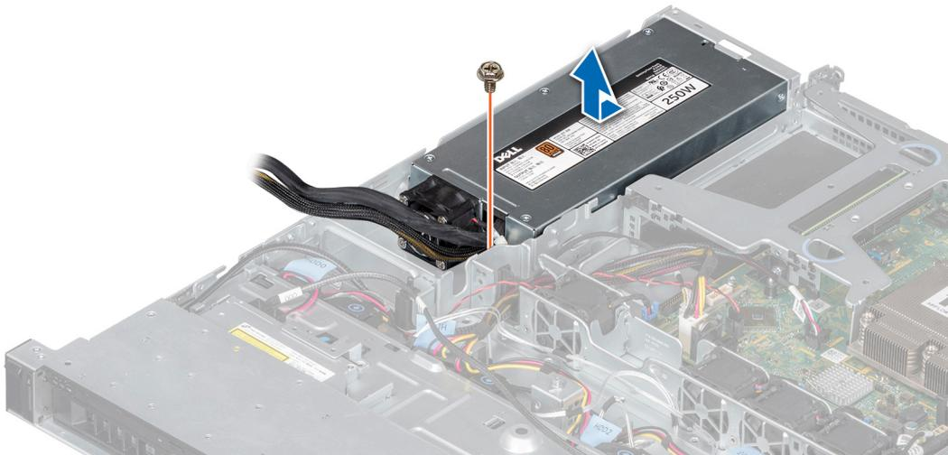
**Figure 69. Removing a cabled power supply unit**
