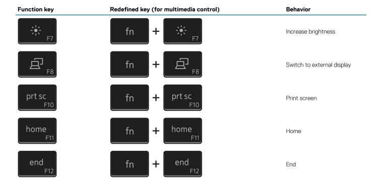
The **Fn** key is also used with selected keys on the keyboard to invoke other secondary functions.
