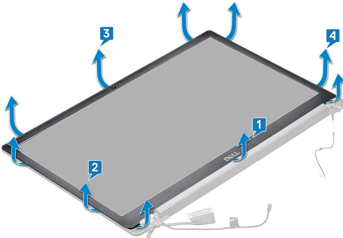
① **NOTE:** Adhesive is used to secure the display bezel to the display panel.
