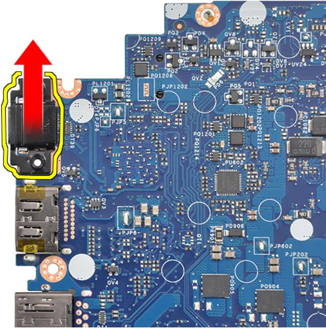
**NOTE:** When removing or reinstalling the USB Type-C bracket to the system board, technicians must place the system board on an ESD mat to avoid damage.
