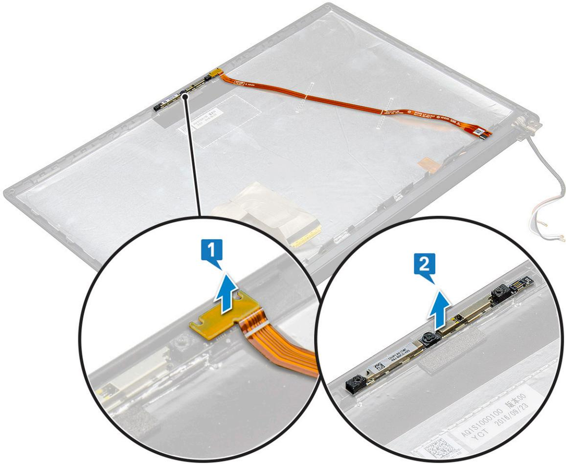
4 To remove the camera module:
