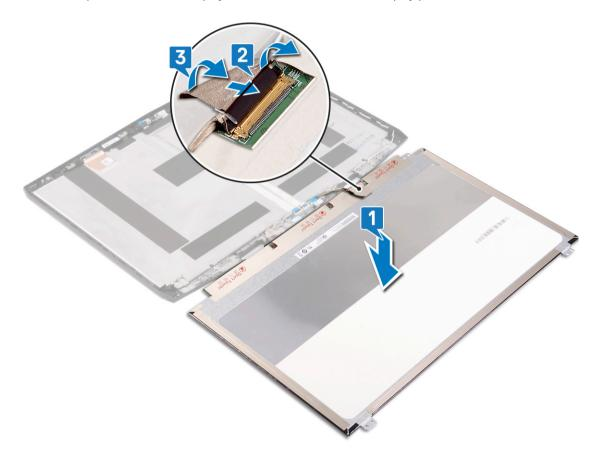
4 Turn over the display panel and gently place it on the display back-cover and antenna assembly.
