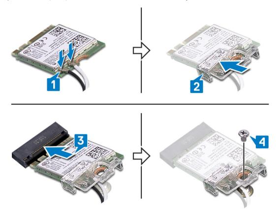
**5** Route the antenna cables on to the securing clips on the system board.
