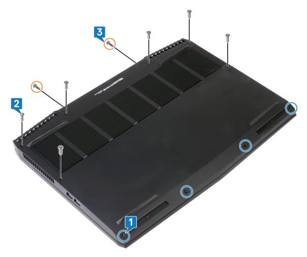
4 Rotate the base cover from front to back and remove the base cover off the palm-rest assembly.
