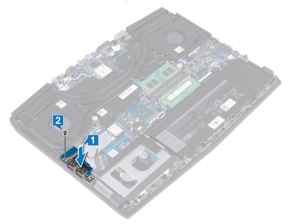
3 Connect the I/O-board cable to the connector on the I/O board and close the latch to secure the cable.
