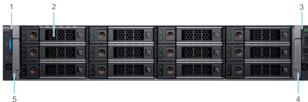
Figure 1. Front view of 24 x 3.5-inch drive system
