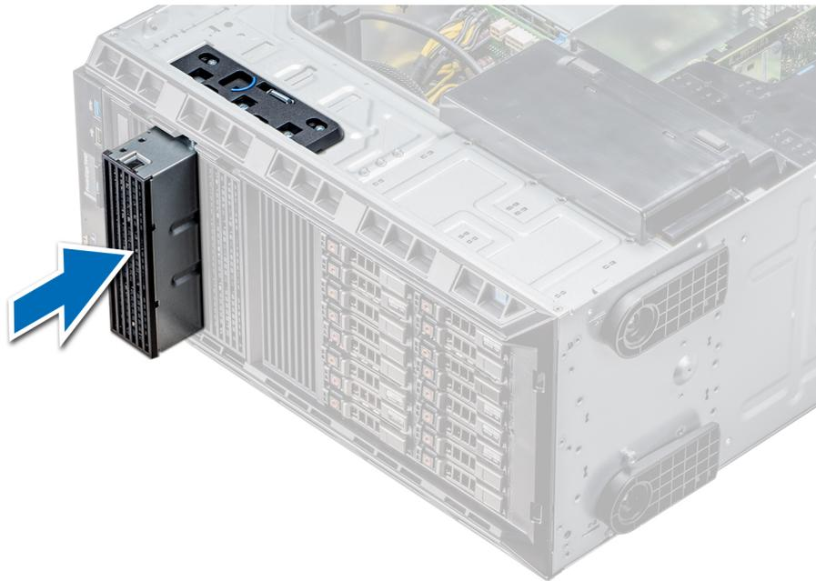
**Figure 39. Installing the optical or tape drive blank**
