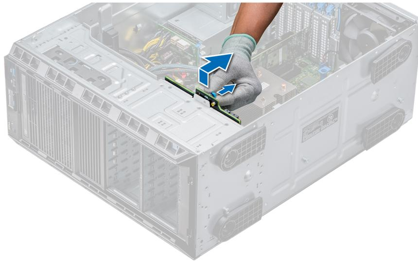
**Figure 51. Removing a backplane**
