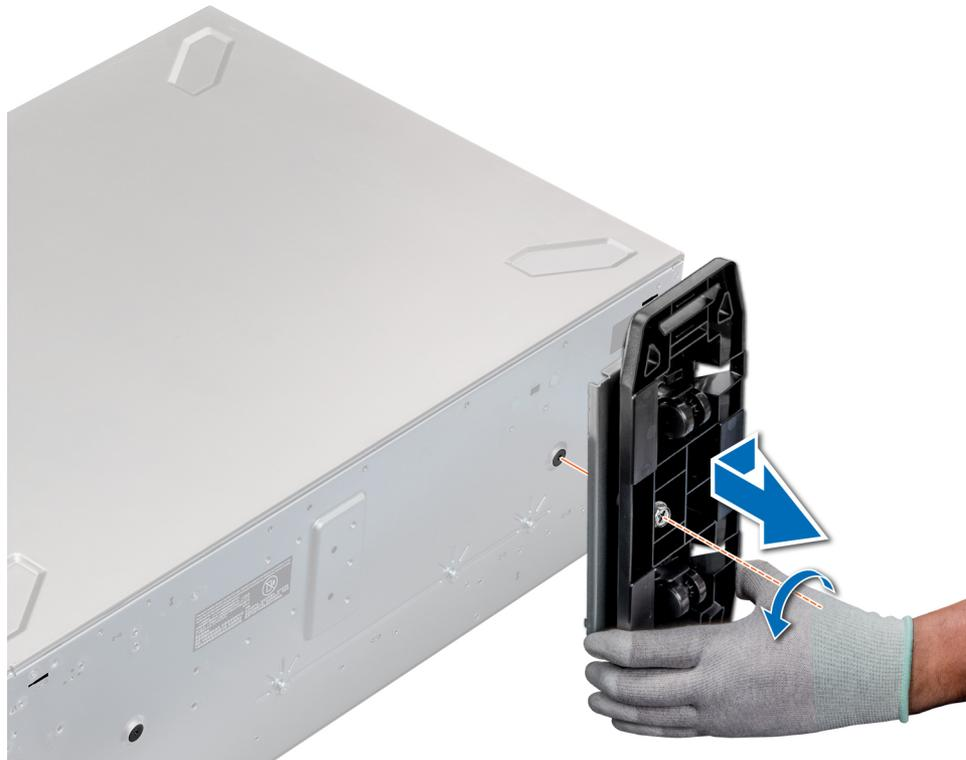
Figure 22. Removing caster wheels
