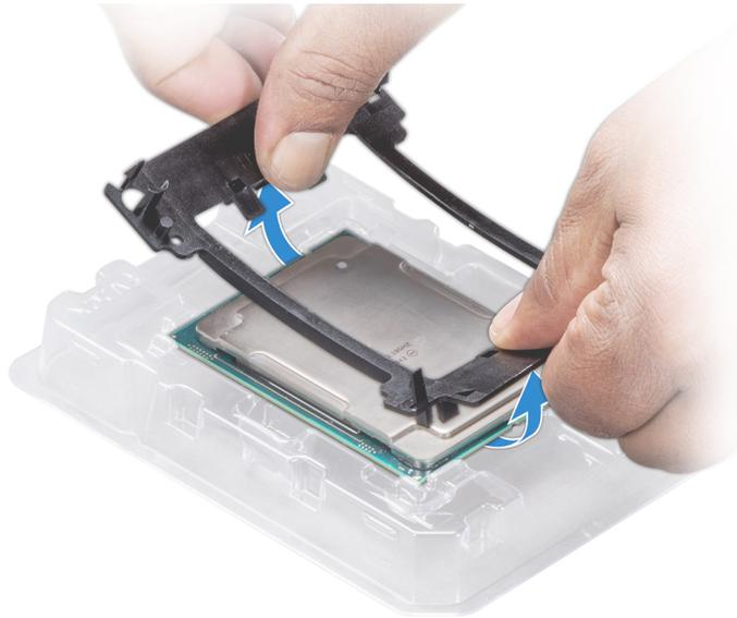
**Figure 72. Removing the processor bracket**
