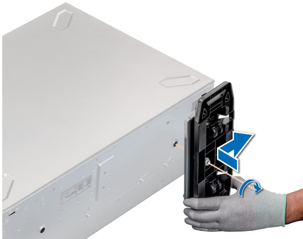
**Figure 23. Installing caster wheels**
