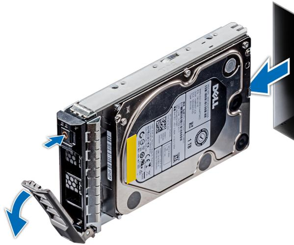
Figure 30. Removing a drive carrier
