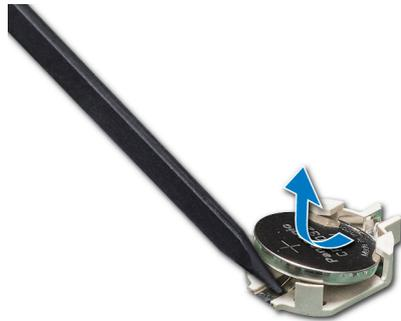
Figure 85. Removing the system battery
