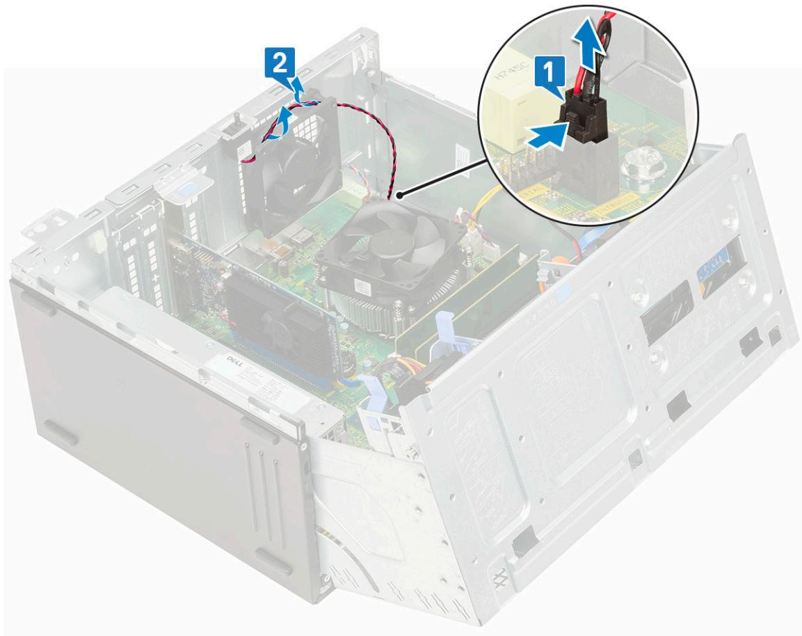
c Disconnect the system fan cable from the connector on the system board [1].
