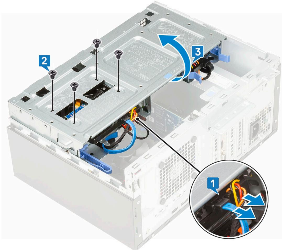
d Remove the 3.5 inch hard drive out of the system.
