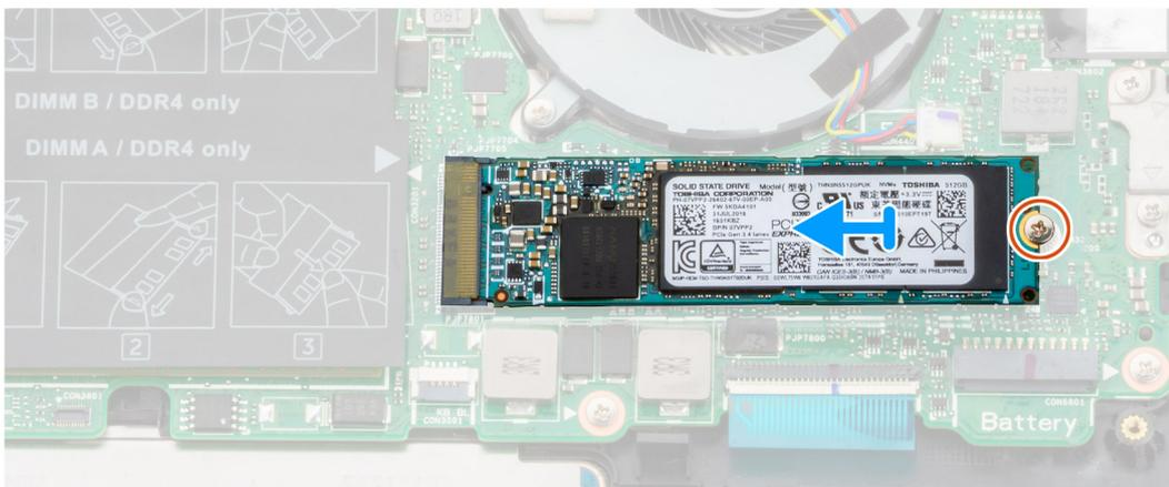
1. Align the notch on the solid-state drive module with the tab on the solid-state drive slot.
