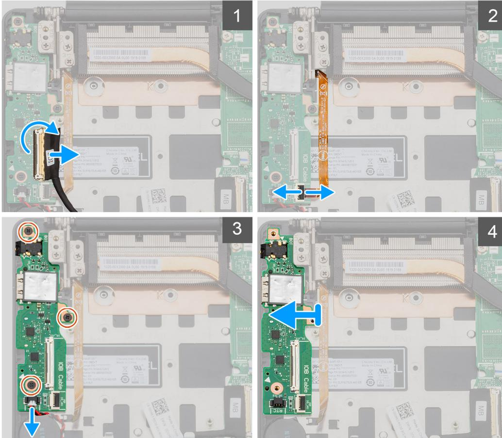
1. Open the latch and disconnect the I/O-board cable from the I/O board.
