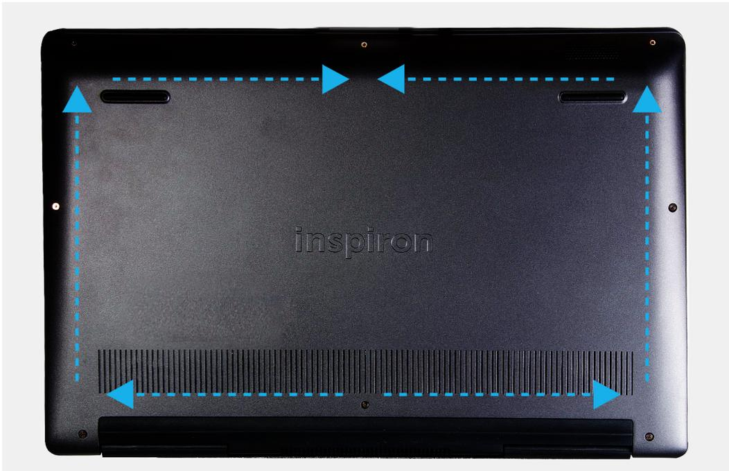
1. Remove the five screws (M2x5) that secure the base cover to the palm-rest and keyboard assembly.
