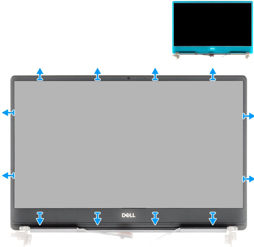
1. Carefully pry the edges of the display bezel off the display back-cover and antenna assembly.
