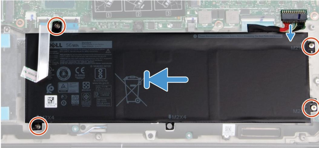
1. Place the battery on the palm-rest and keyboard assembly and align the screw holes on the battery with the screw holes on the palm-rest and keyboard assembly.
