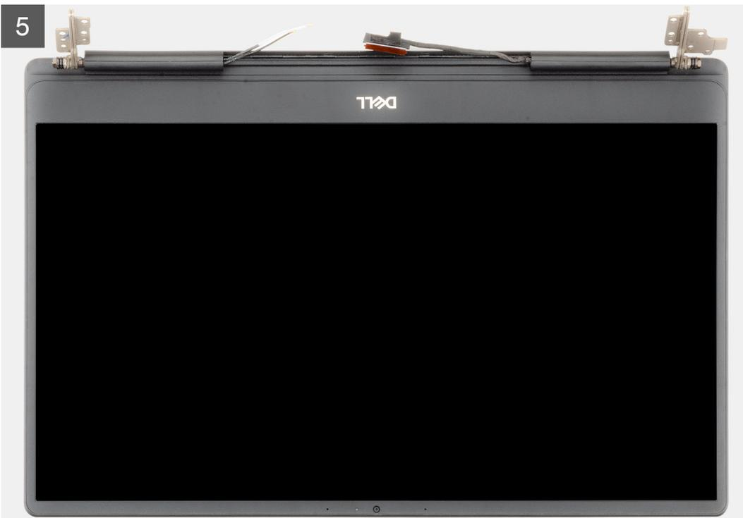
1. Locate the display cable and display hinges on your computer.
