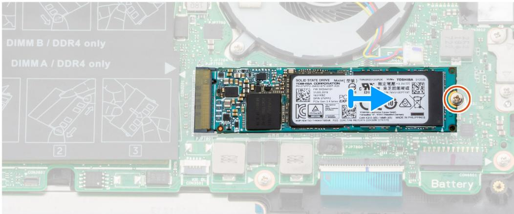
1. Remove the screw (M2x4) that secures the solid-state drive to the system board.
