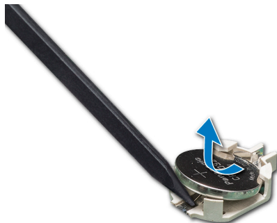
Figure 101. Removing the system battery
