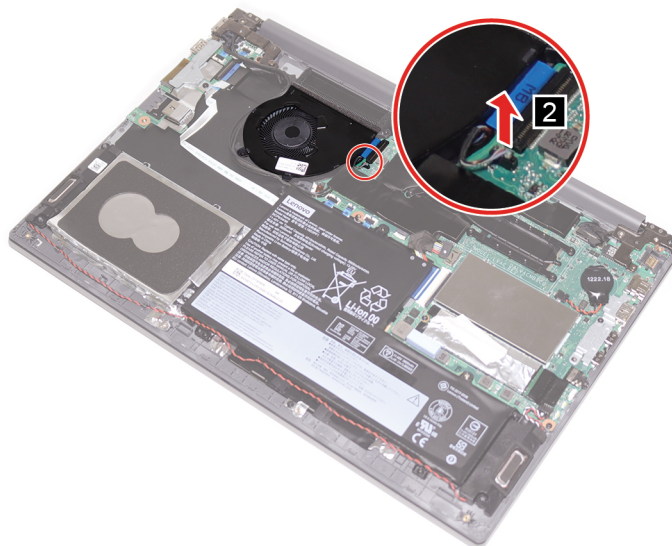
Figure 21. Disconnect the fan cable from the system board
