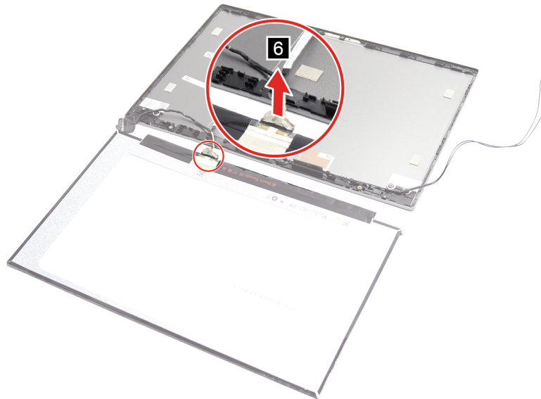
Figure 65. Remove the EDP cable
