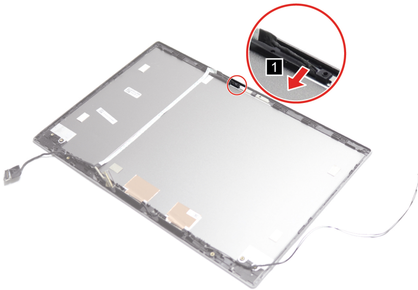
Figure 66. Disconnect the camera connector
