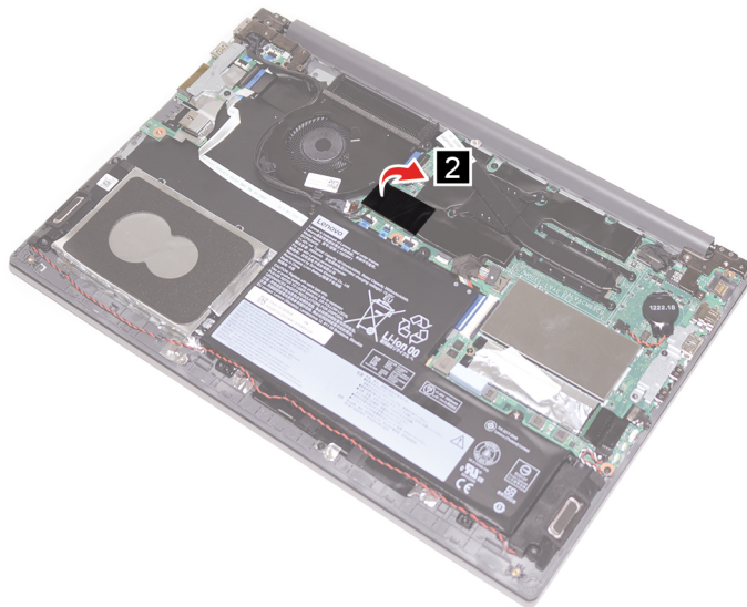
Figure 17. Remove the mylar from the WLAN card
