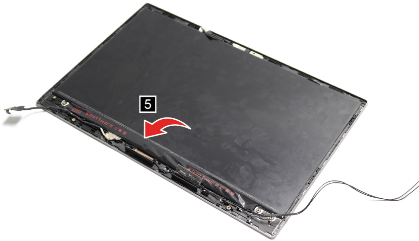
Figure 64. Carefully lift the LCD panel from the LCD cover
