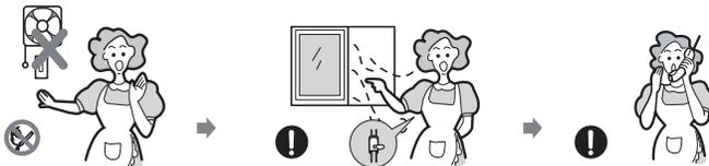
\* The fuel gas contains mercaptan, so that you can smell the gas leak (smell of rotten garlic or egg) even where only 1/1000 of the gas is in the air.
