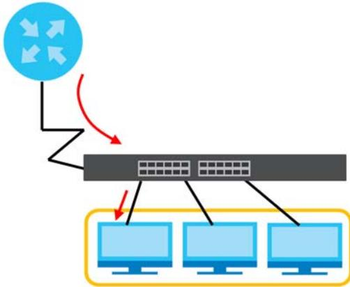
Figure 99 Static Multicast Forwarding to Multiple Ports
