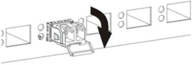
**Figure 16** Transceiver Removal Example
