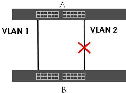
With MSTP, VLANs 1 and 2 are mapped to different spanning trees in the network. Thus traffic from the two VLANs travel on different paths. The following figure shows the network example using MSTP.
