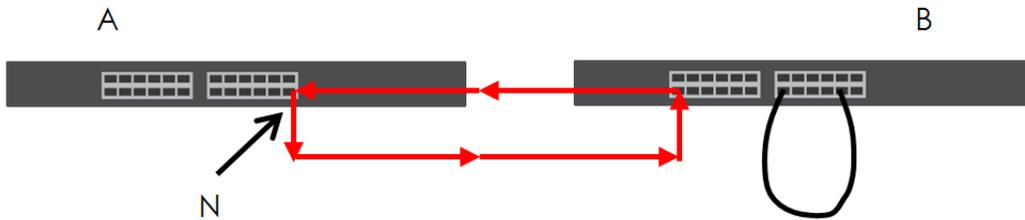
The loop guard feature checks to see if a loop guard enabled port is connected to a switch in loop state. This is accomplished by periodically sending a probe packet and seeing if the packet returns on the same port. If this is the case, the Switch will shut down the port connected to the switch in loop state.
