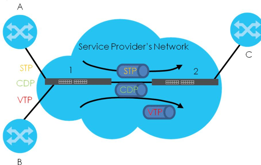
In the following example, if you enable L2PT for STP, you can have switches **A**, **B**, **C** and **D** in the same spanning tree, even though switch **A** is not directly connected to switches **B**, **C** and **D**. Topology change information can be propagated throughout the service provider's network.
