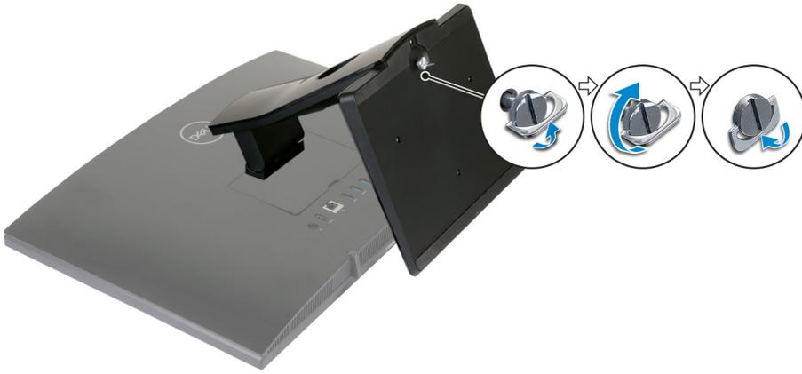
3. Tighten the captive screw to secure the base to the stand riser.
