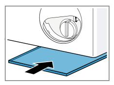
**6.** To allow the detergent solution to flow out into the container, remove the pump cap carefully.
