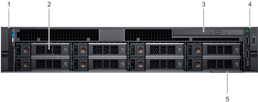
Figure 3. Front view of 8 x 3.5-inch drive system
