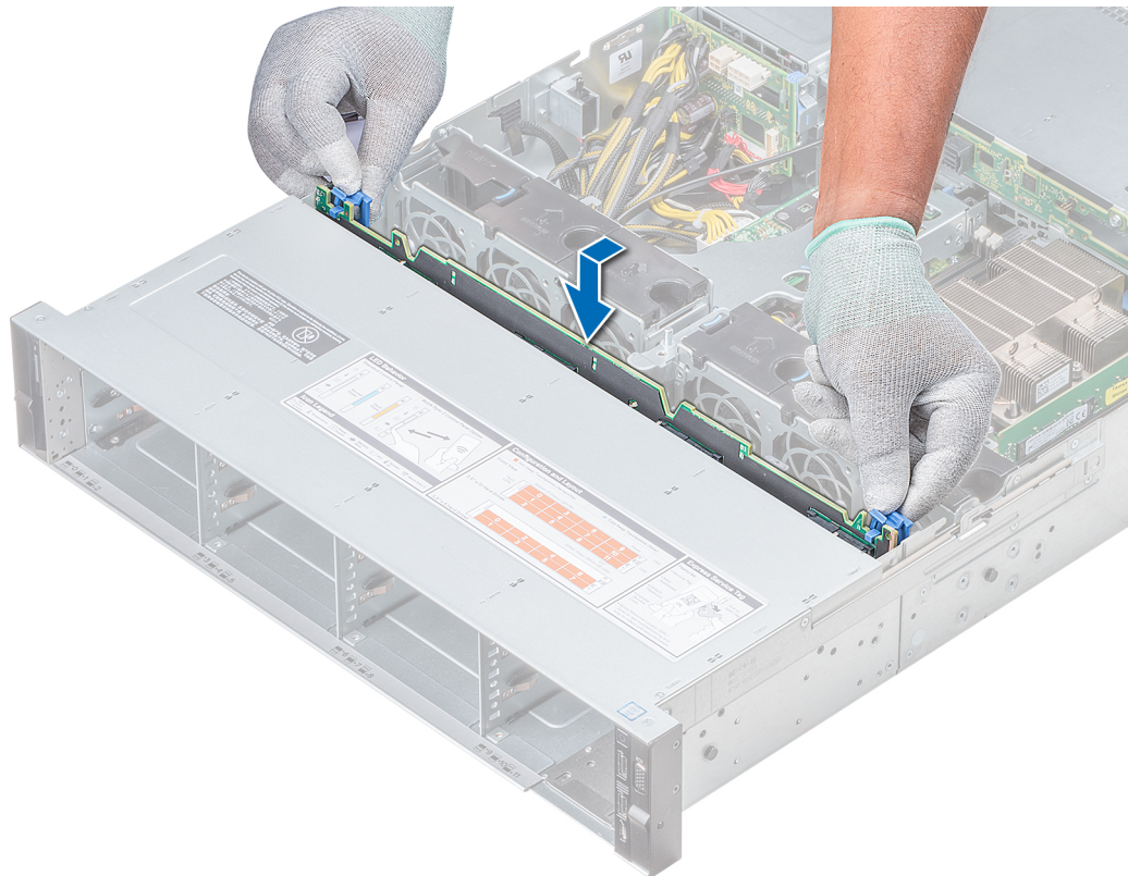
Figure 102. Installing the backplane
