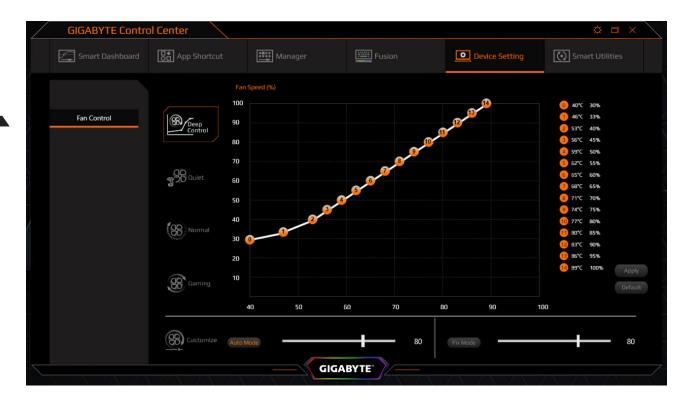
When you get into Deep Control mode, you will get 15 configurable sensing point of the Fan curve. You can drag them to the expected position to assign the different fan speed on every temperature. Remember the rule: the temperature and fan speed should always be equal or higher/faster than the previous point.
