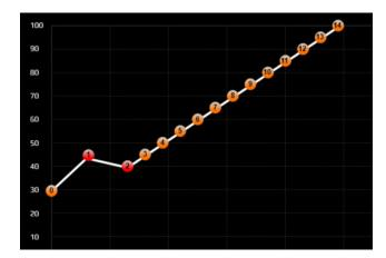
For example, let's set the No.1 point to 46°C and 44% fan speed. The speed is higher than the point No.2. Now you get two points in red color because of it against the rule. You can solve this situation easily by changing the fan speed of point No.1 lower than No.2.
