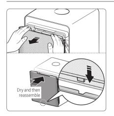
STEP1 Remove the front panel.
