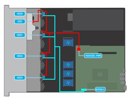
Figure 66. Cable routing -  $4 \times 3.5$ -inch cabled drive with SATA
