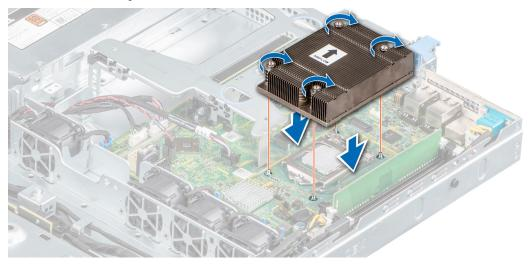
Figure 56. Installing the heat sink
