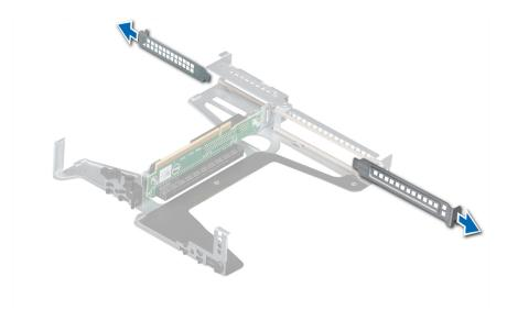
Figure 45. Removing expansion card filler
