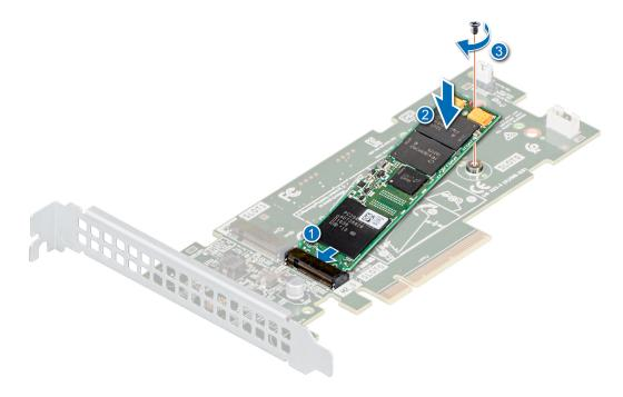
Figure 48. Installing the M.2 SSD module
