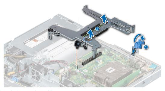
Figure 39. Removing the expansion card riser
