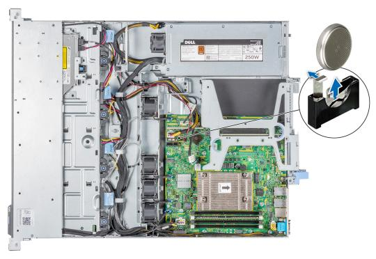
Figure 49. Removing system battery
