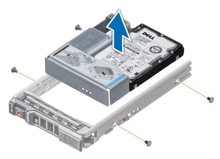
Figure 27. Removing a 3.5-inch drive adapter from a 3.5-inch drive carrier
