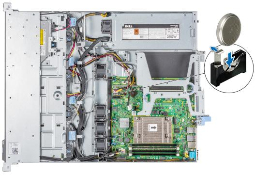
Figure 50. Installing system battery
