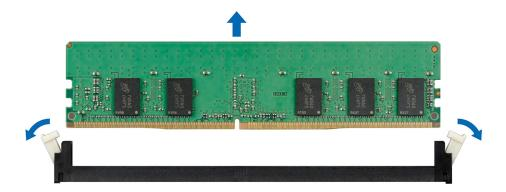
Figure 36. Removing a memory module
