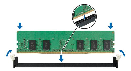
Figure 37. Installing a memory module
