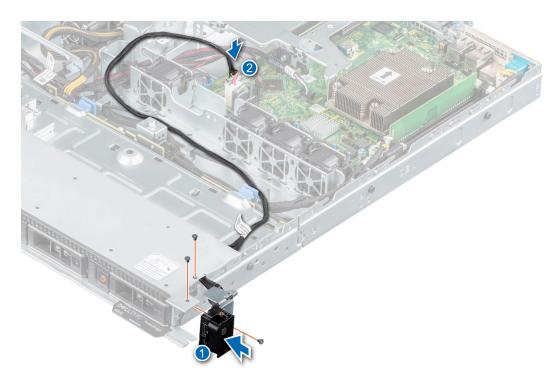
Figure 78. Installing the right control panel
