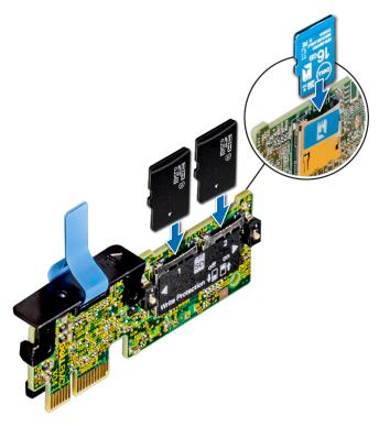
Figure 59. Installing the MicroSD card
