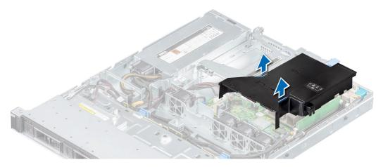
Figure 13. Removing the air shroud
