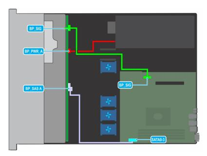
Figure 64. Cable routing -  $4 \times 3.5$ -inch drive backplane with SATA
