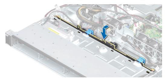
Figure 62. Installing the backplane
