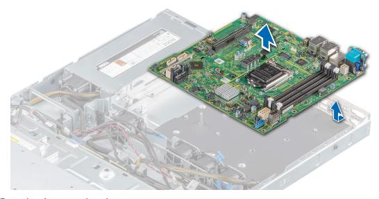
Figure 72. Removing the system board
