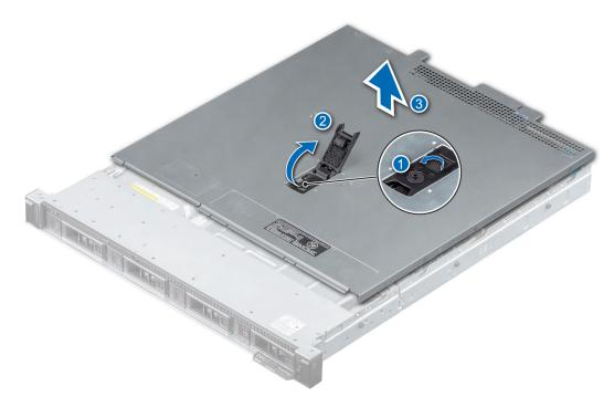
Figure 11. Removing the system cover
