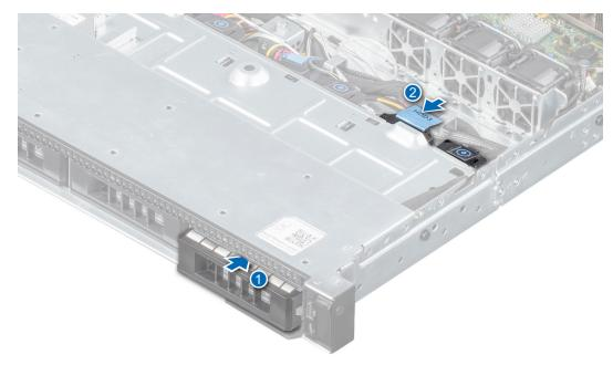
Figure 30. Installing a cabled drive
