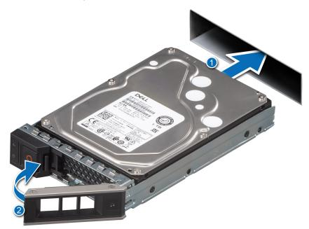
Figure 22. Installing the hot-swappable drive
