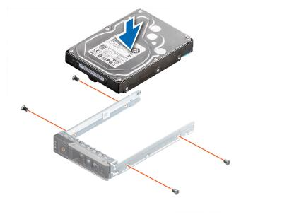
Figure 24. Installing a drive into the drive carrier
