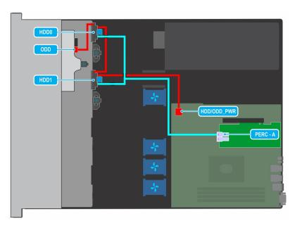
Figure 67. Cable routing -  $2 \times 3.5$ -inch cabled drive with PERC
