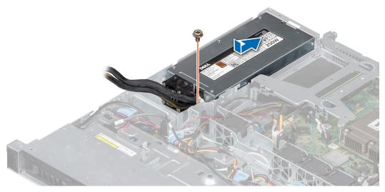
Figure 70. Installing a cabled power supply unit
