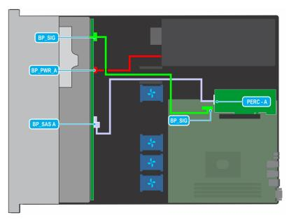
Figure 63. Cable routing - 4 x 3.5-inch drive backplane with PERC
