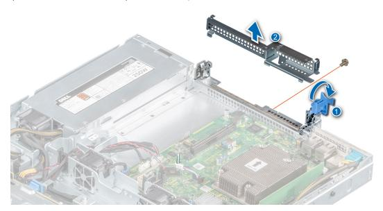
Figure 41. Removing the expansion card riser filler
