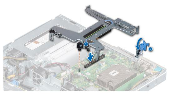
Figure 42. Installing the expansion card riser
