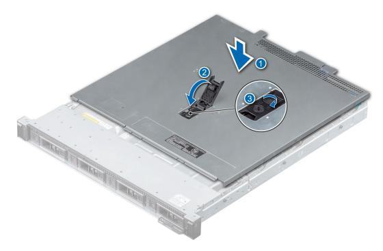
Figure 12. Installing the system cover
