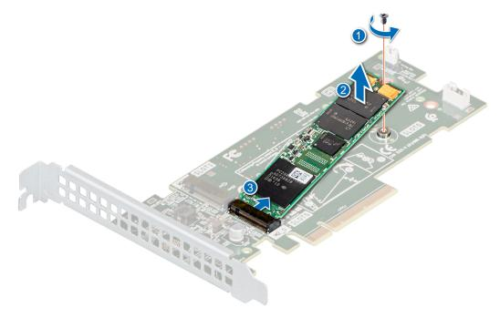
Figure 47. Removing the M.2 SSD module
