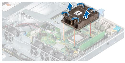
Figure 53. Removing the heat sink
