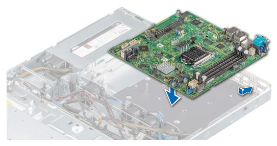
Figure 73. Installing the system board
