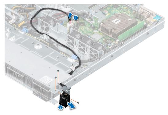
Figure 77. Removing the right control panel
