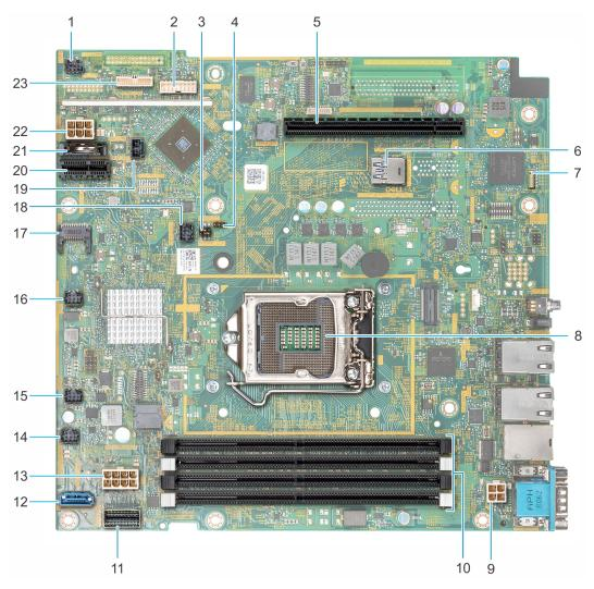
Figure 79. System board connectors
