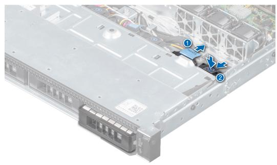
Figure 29. Removing a cabled drive
