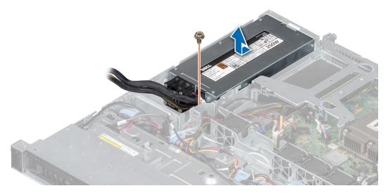
Figure 69. Removing a cabled power supply unit
