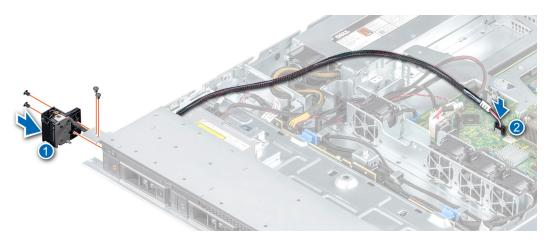
Figure 76. Installing the left control panel
