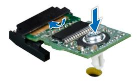
Figure 74. Installing the TPM
