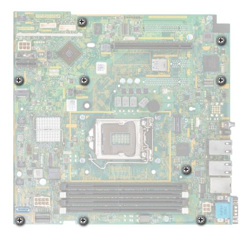
Figure 71. Screws securing the system board
