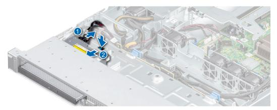
Figure 51. Removing the optional optical drive
