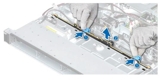
Figure 61. Removing the drive backplane
