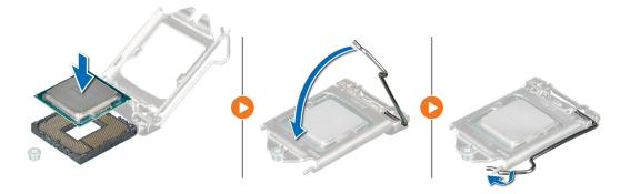
Figure 55. Installing the processor
