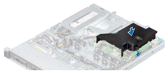
Figure 14. Installing the air shroud
