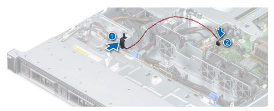
Figure 34. Installing the intrusion switch
