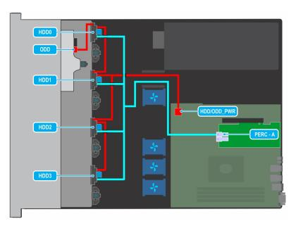
Figure 65. Cable routing - 4 x 3.5-inch cabled drive with PERC
