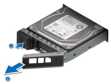
Figure 21. Removing a hot-swappable drive
