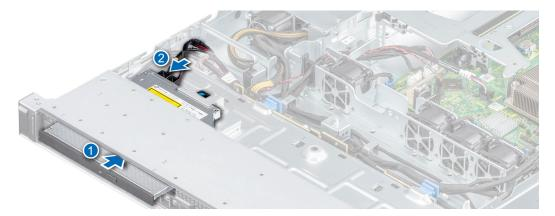
Figure 52. Installing the optional optical drive
