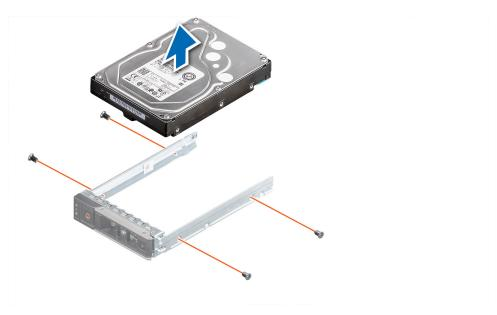
Figure 23. Removing the drive from the drive carrier
