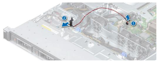
Figure 33. Removing the intrusion switch
