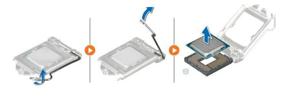
Figure 54. Removing the processor
