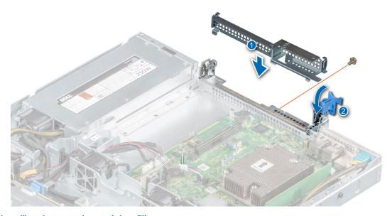
Figure 40. Installing the expansion card riser filler
