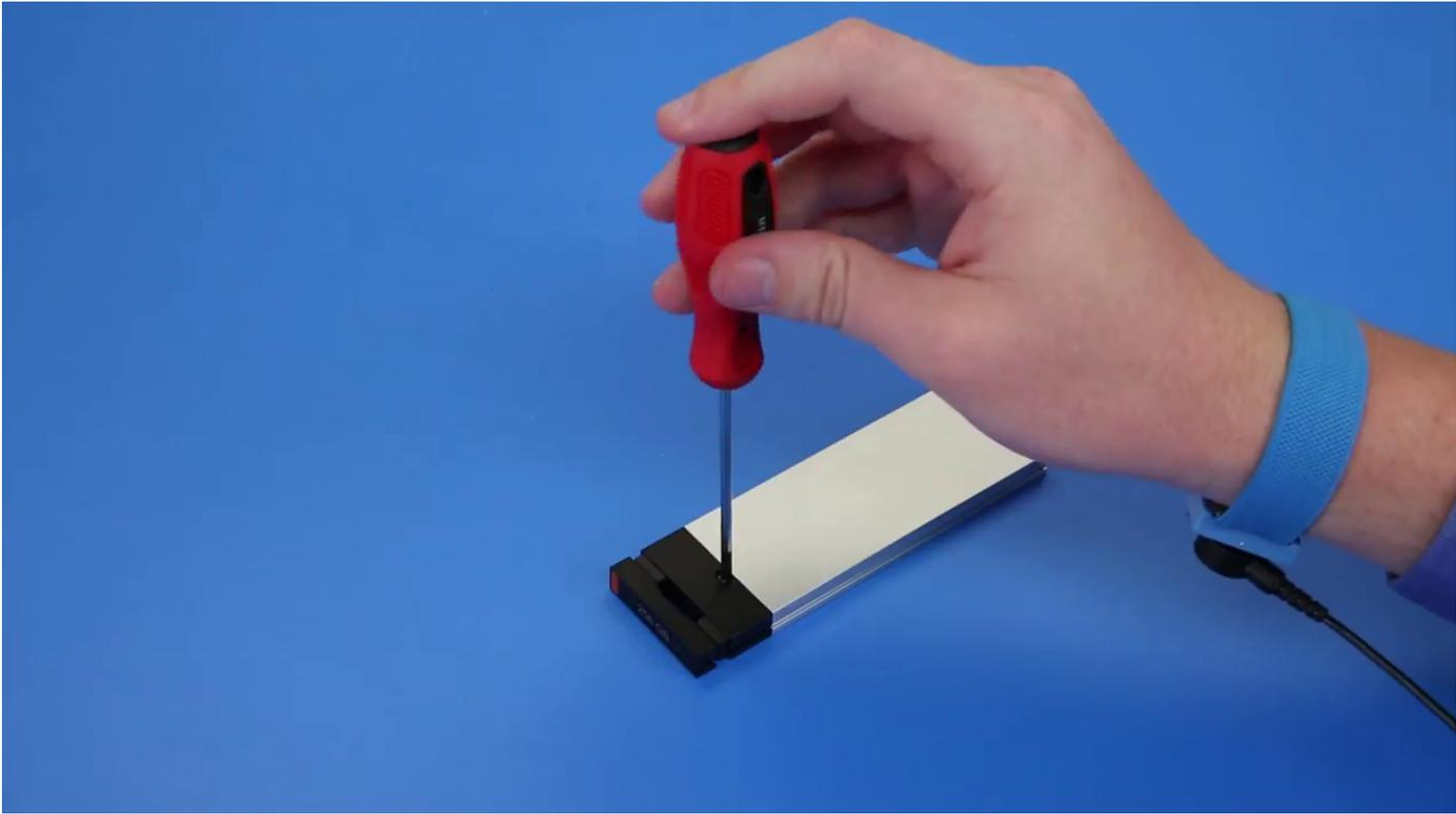
c) Slide the SSD cover from the top of the carrier.
