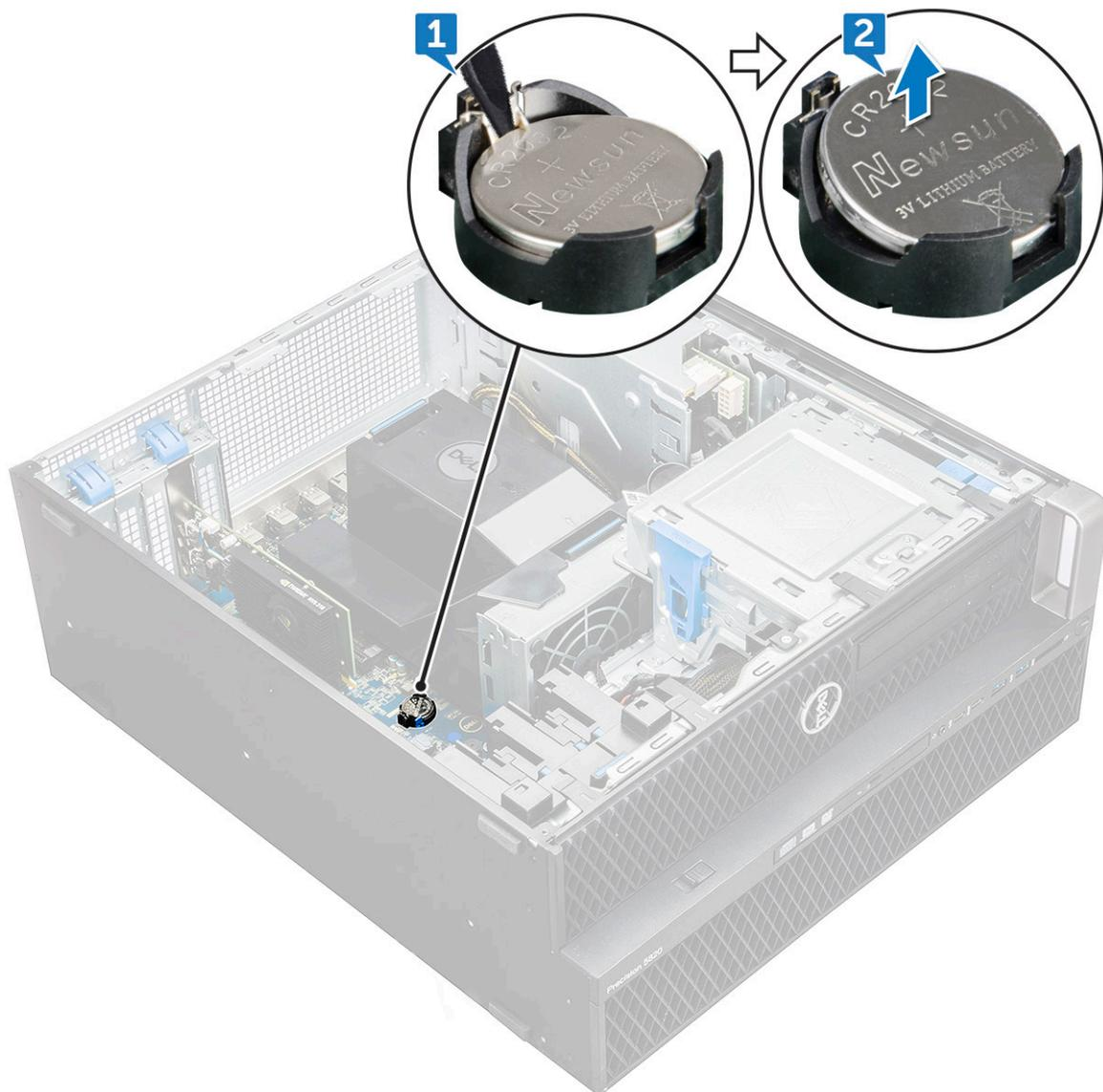
b) Lift the coin-cell battery out of the system board.
