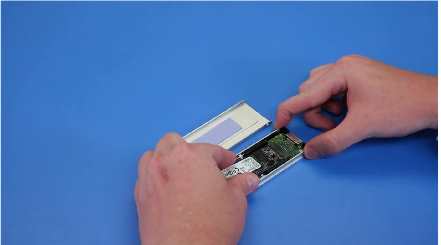
3. Replac the two side screws and the central screw.
