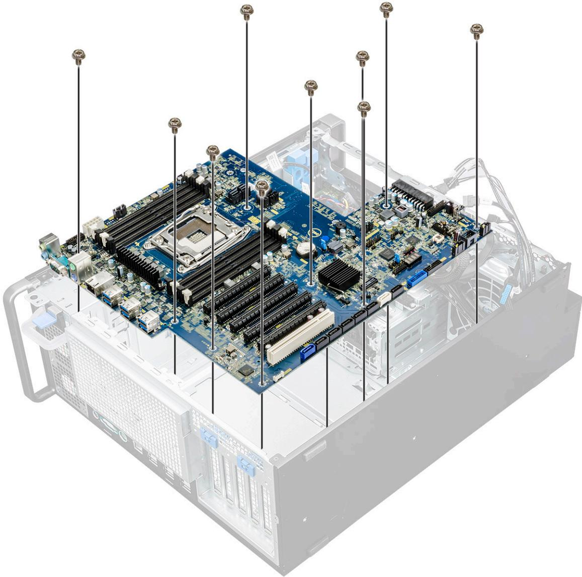
f) Slide the system board towards HDD bracket module to detach it from the system.
