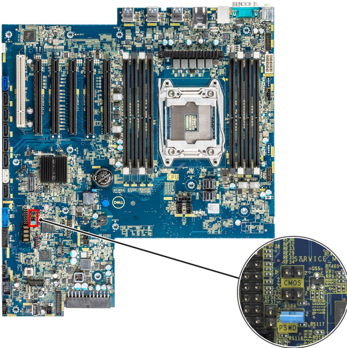
Plugging the power management cable into the Clear CMOS jumper will cause the BIOS to reset when sending a remote restart request to the Teradici card. You will then have to reset the time and BIOS settings.
