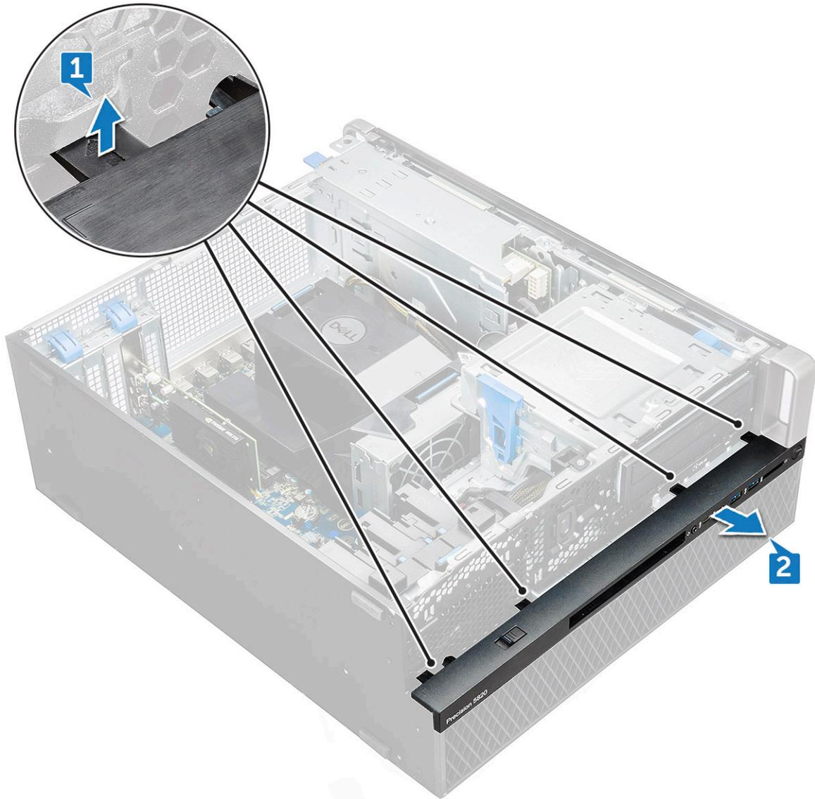
b) Lift the bezel from the chassis.
