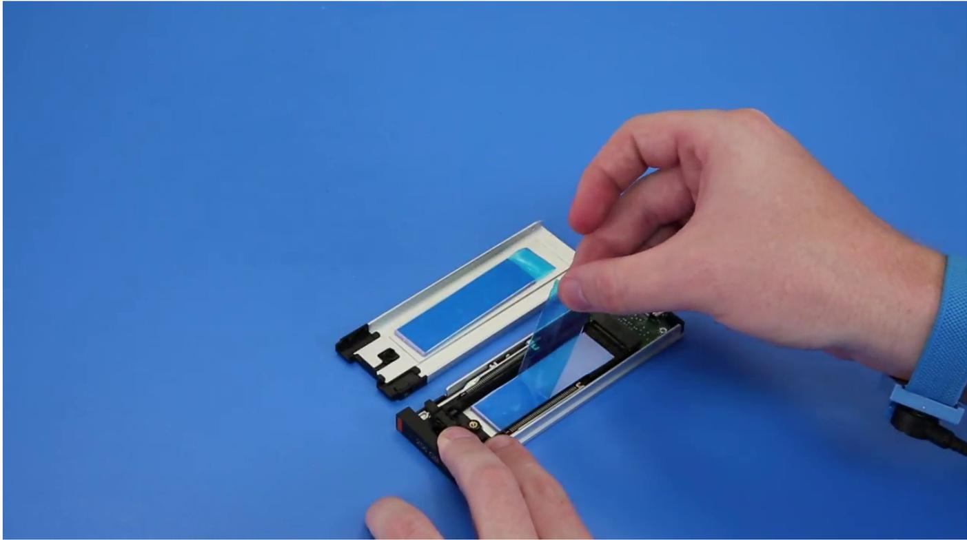
c) Peel off the adhesive tape from the SSD carrier cover.
