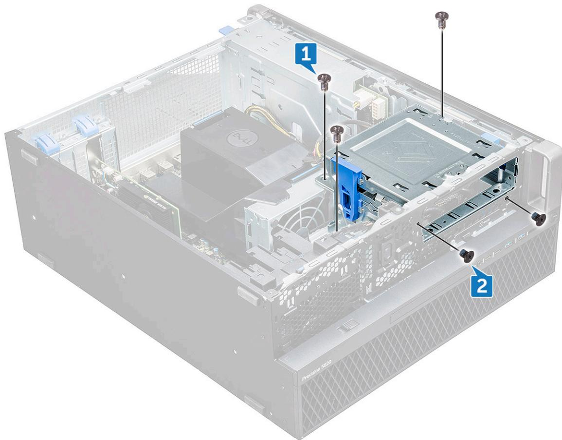
b) Slide the ODD bracket toward the rear of the system and lift it away from the chassis.
