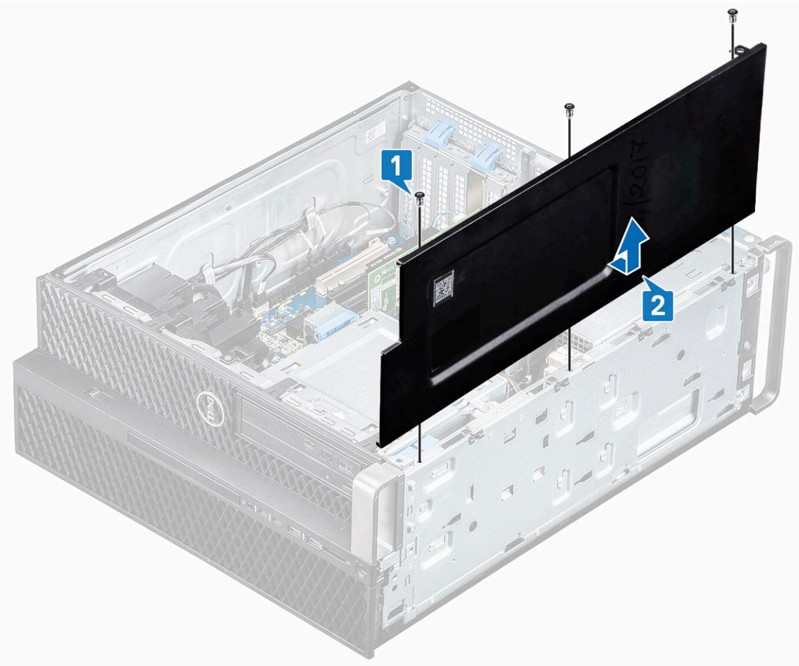
5 Align and install the side cover to the system.
