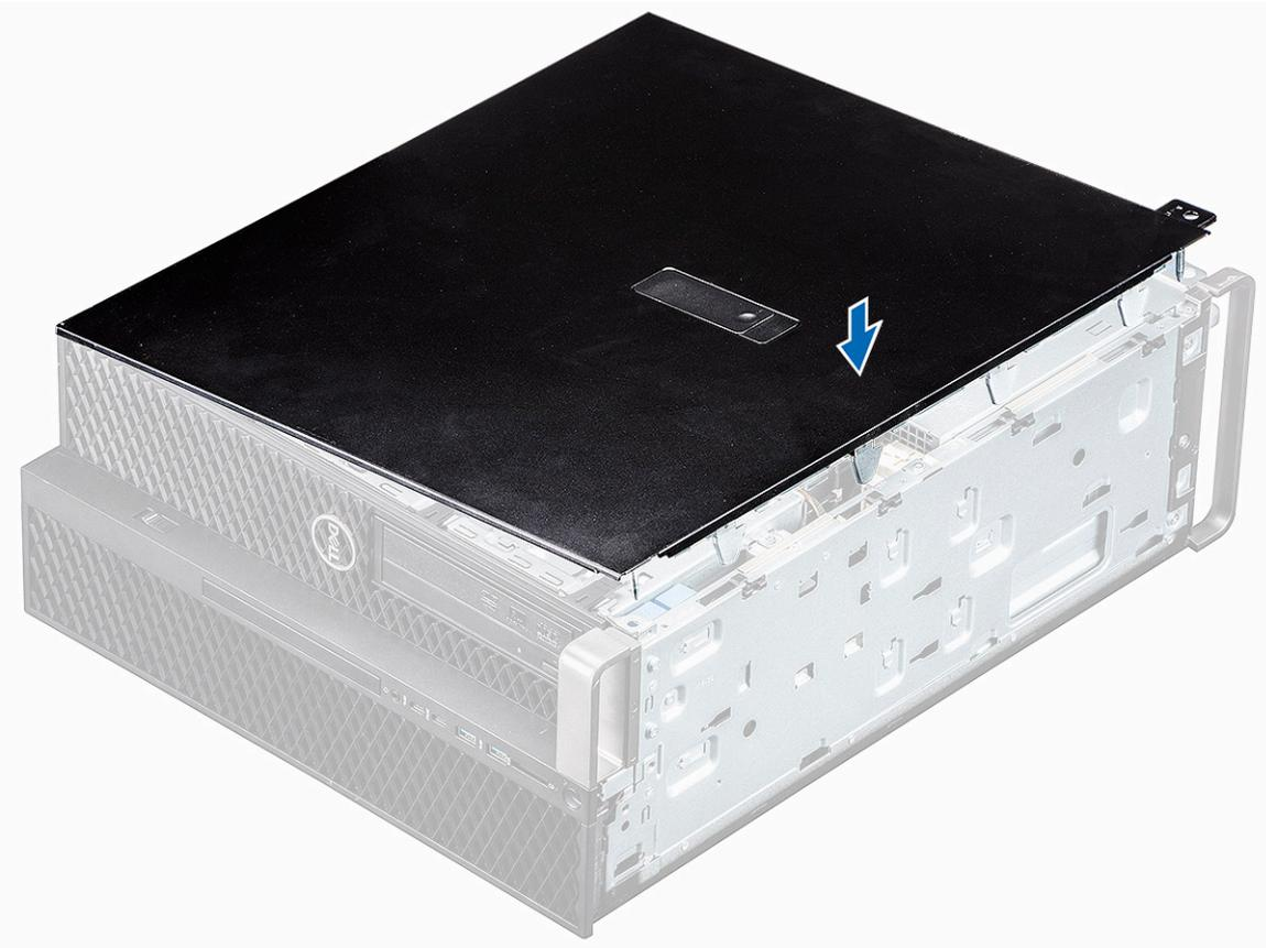
**⚠ CAUTION:** Ensure to install the side cover on the system to prevent any hazards or loss of components.
