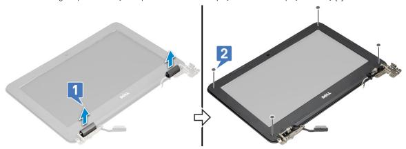
4. Remove the four M2.5x3.5 screws and pry the edges to release the display bezel from the display assembly [2,3].
