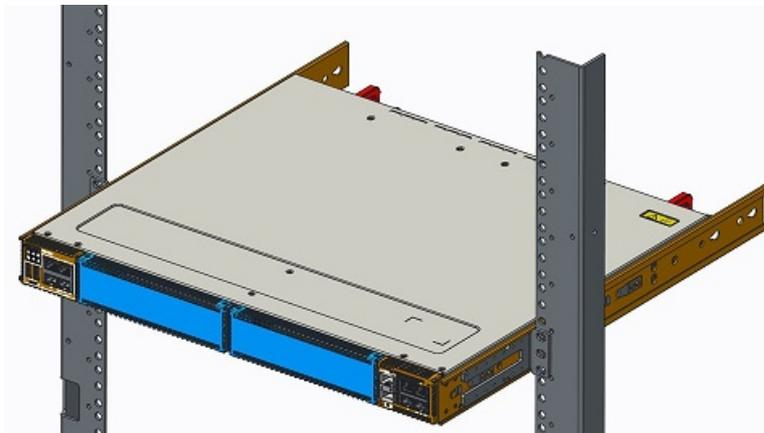
**Figure 9. Platform two-post installed**
