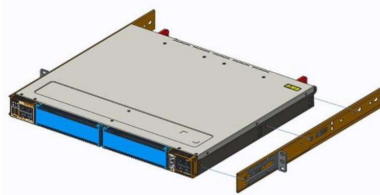
**Figure 8. Platform rail attachment**
