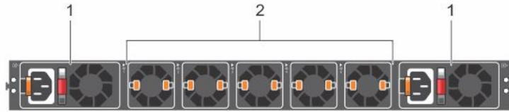
**Figure 3. VEP4600 PSU-side view**
