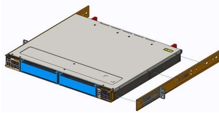
**Figure 4. Platform rail attachment**
