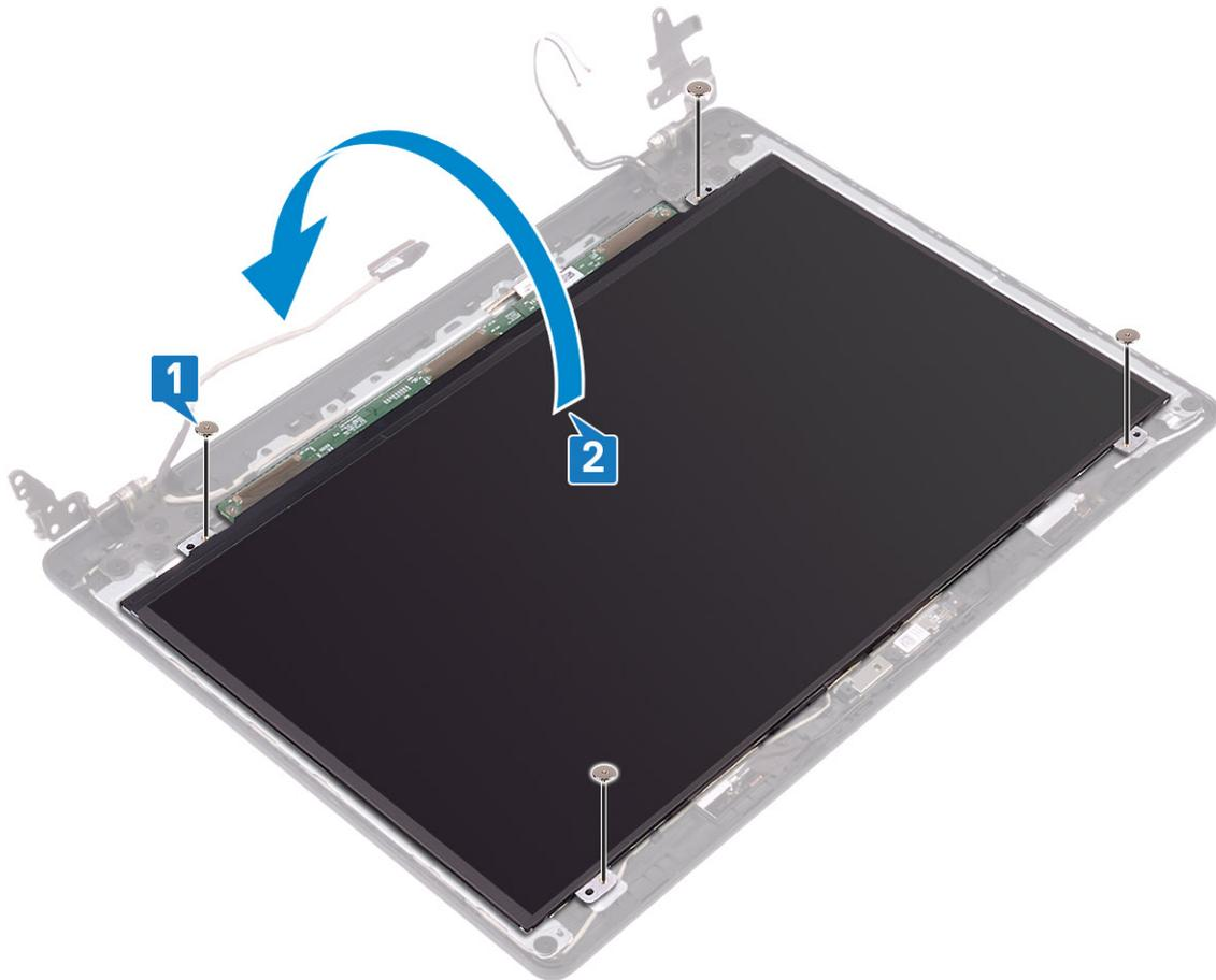
3. Peel the tape that secures the display cable to the back of the display panel [1].
