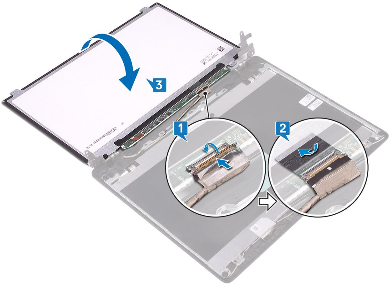
3. Turn the display panel over and place it on the display back-cover and antenna assembly [3].
