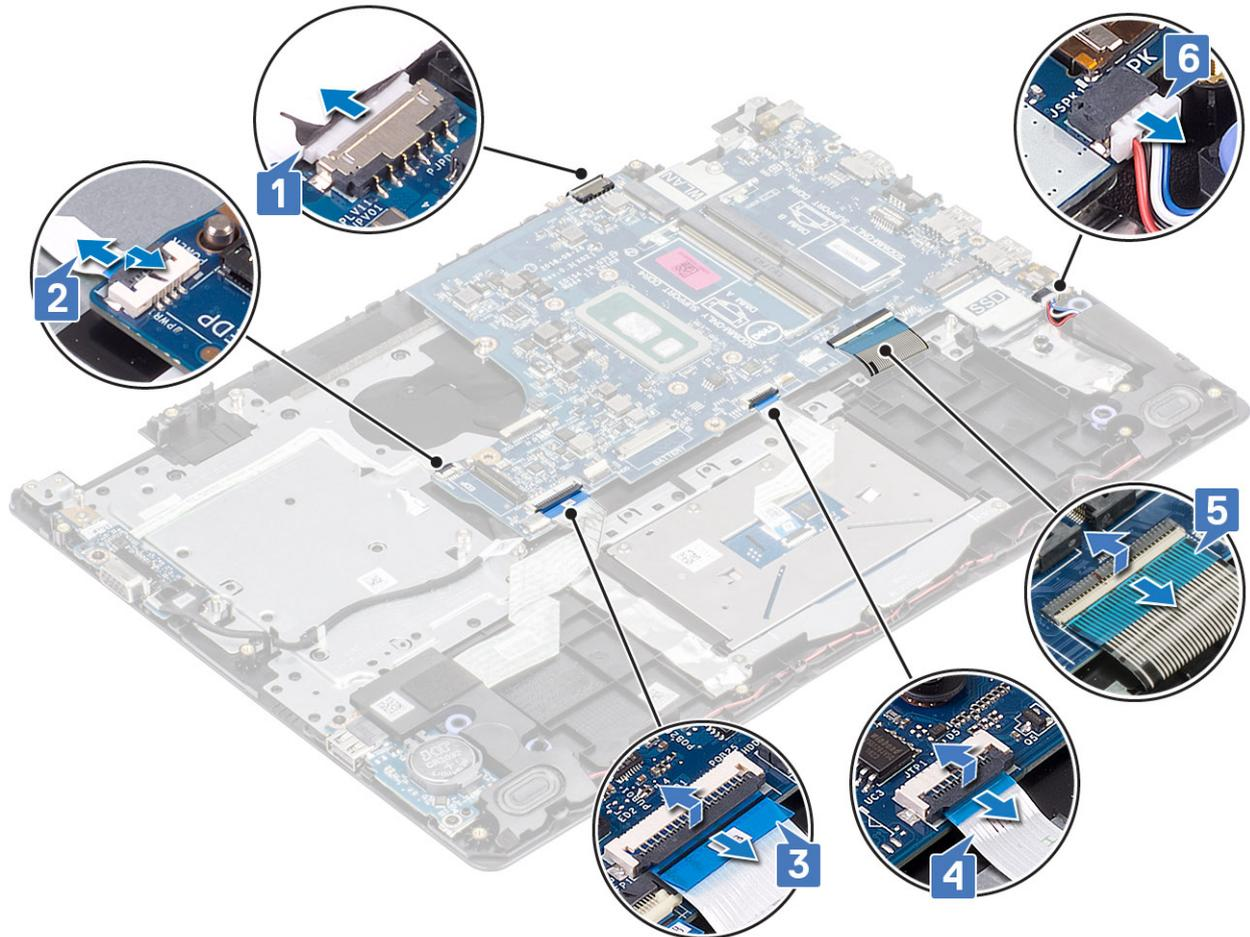
2. Remove the single (M2x4) screw that secures the system board to the palmrest and keyboard assembly [1].
