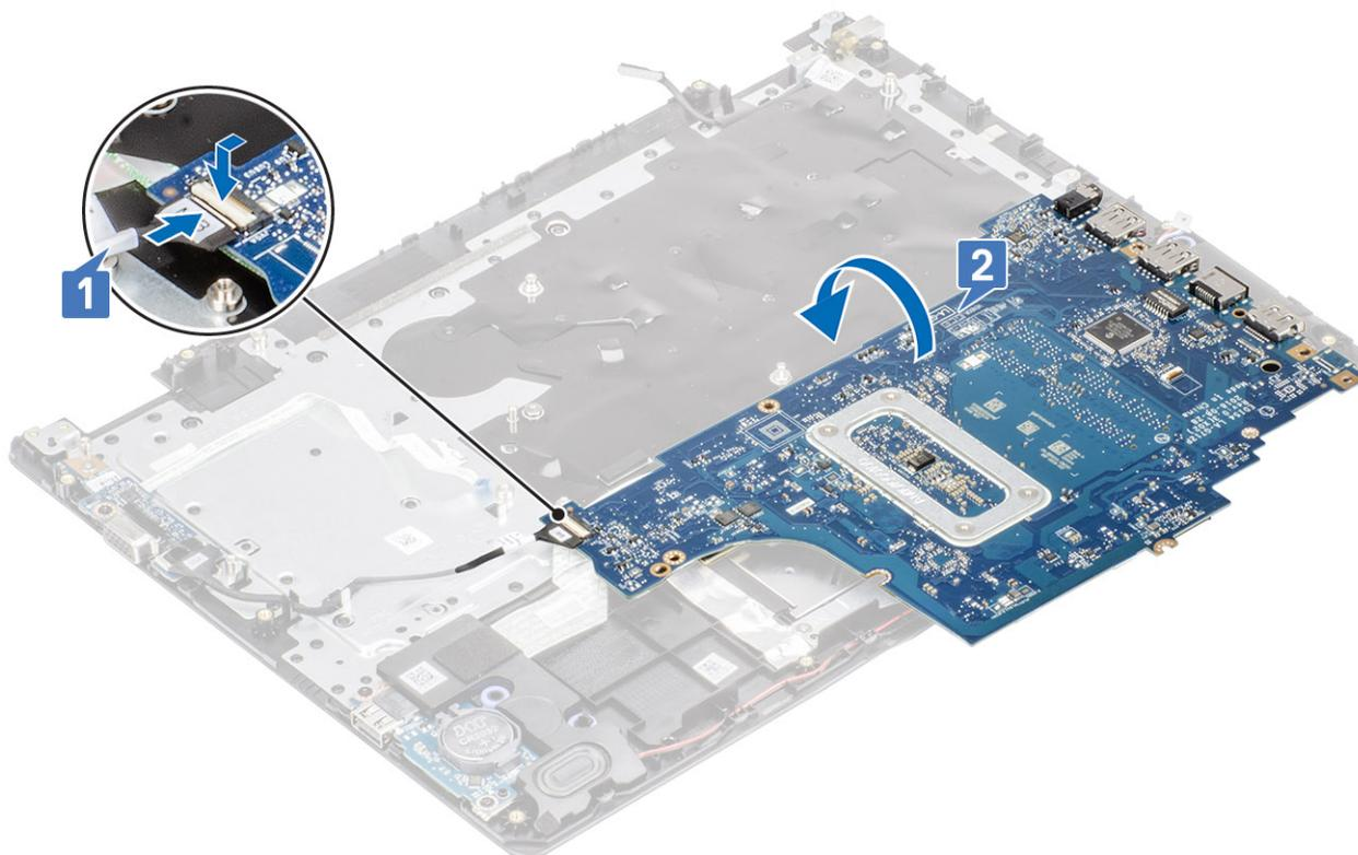
3. Align the screw hole on the system board with the screw hole on the palmrest and keyboard assembly [1].
