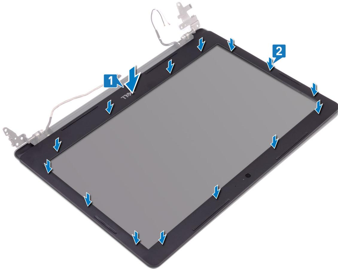
2. Insert the tabs on the display-hinge cover to the slots on the display back-cover and antenna assembly.
