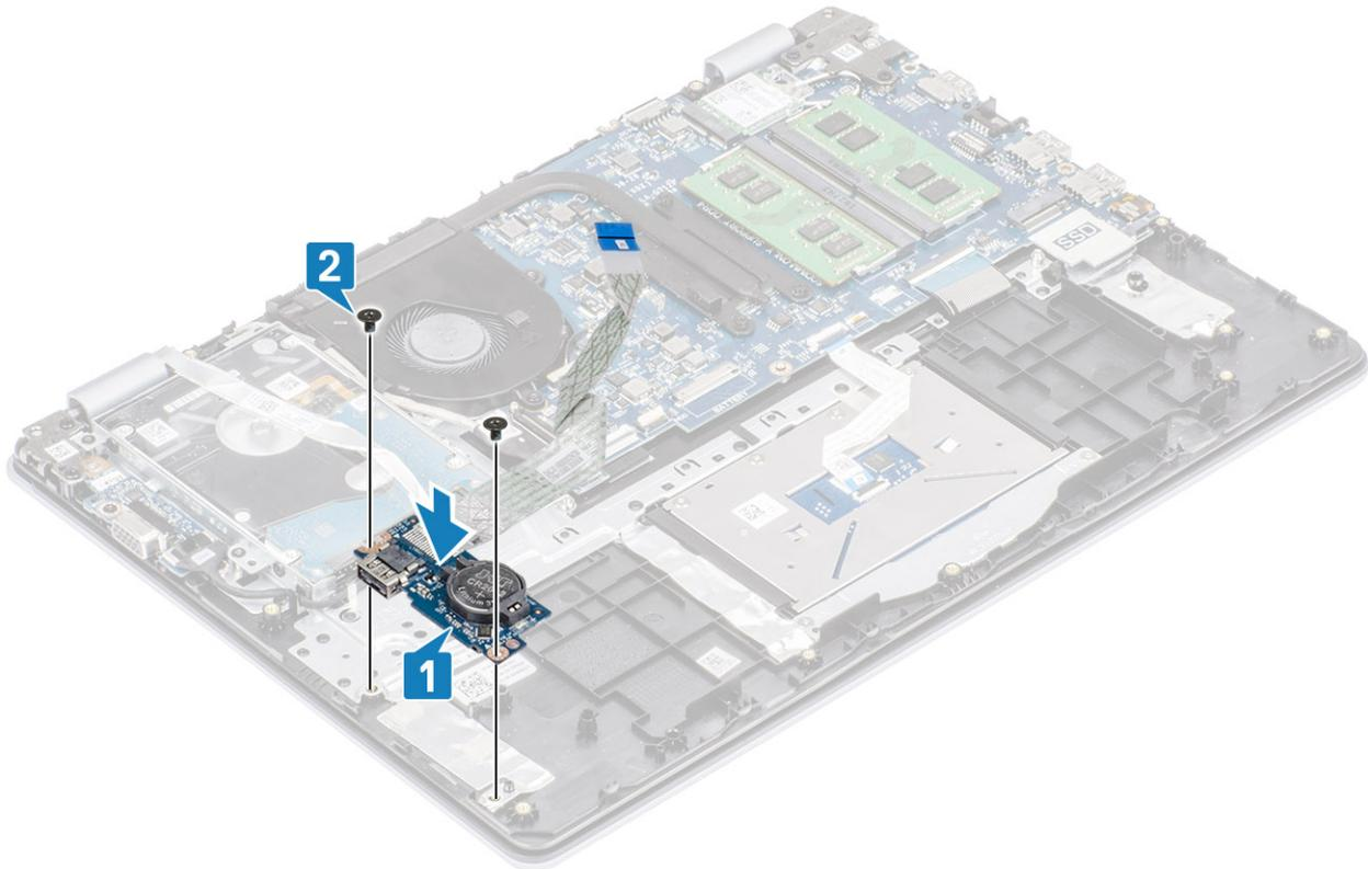
3. Adhere the I/O board cable to the palm rest and keyboard assembly [1].
