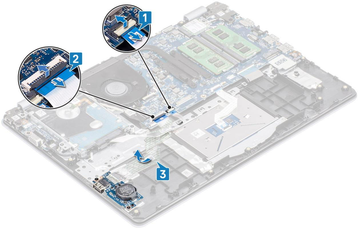
4. Remove the two (M2x4) screws that secure the I/O board to the palm rest and keyboard assembly [1].
