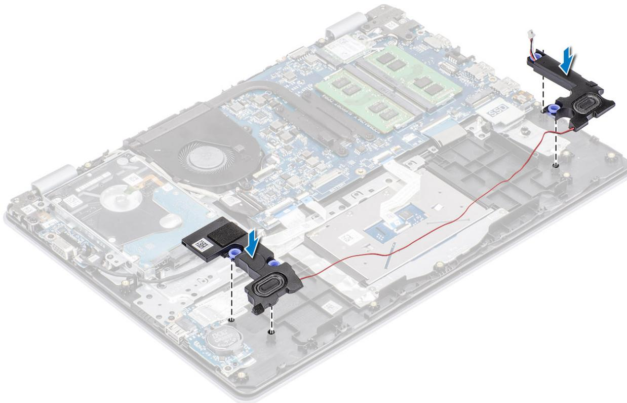
2. Route the speaker cable through the routing guides on the palm rest and keyboard assembly [1].
