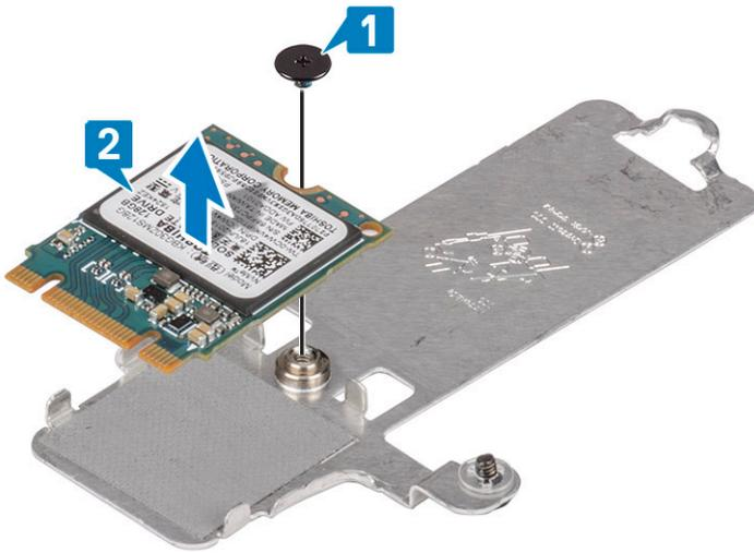
3. Align the notch on the solid-state drive with the tab on the solid-state drive slot.
