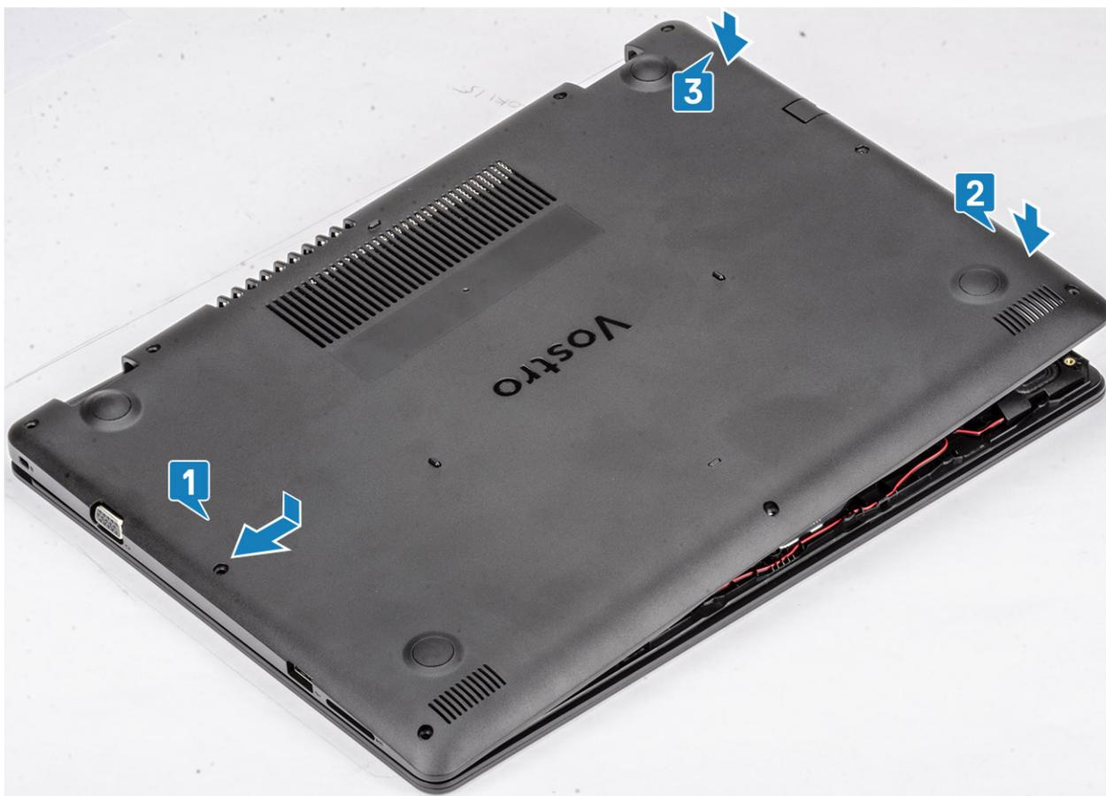
3. Tighten the three captive screws and replace the six (M2.5x6) screws that secure the base cover to the palmrest and keyboard assembly [1, 2].
