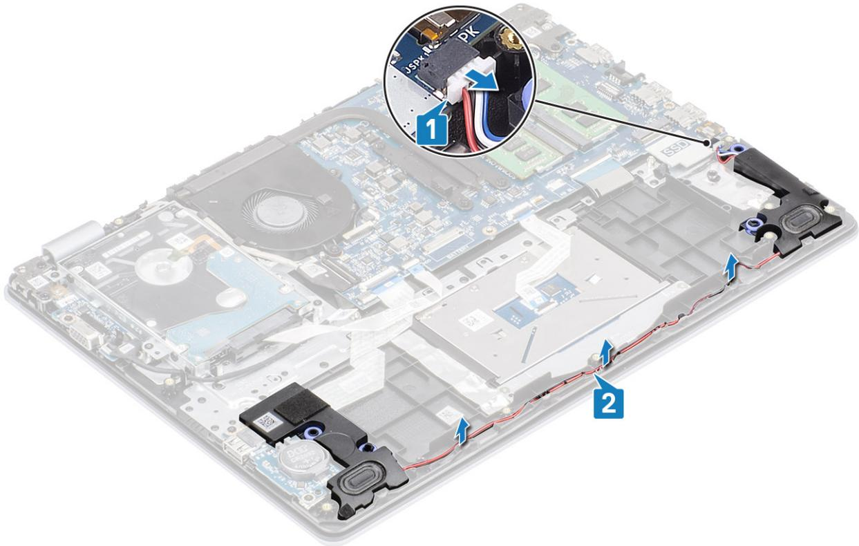
3. Lift the speakers, along with the cable, off the palm rest and keyboard assembly [3].
