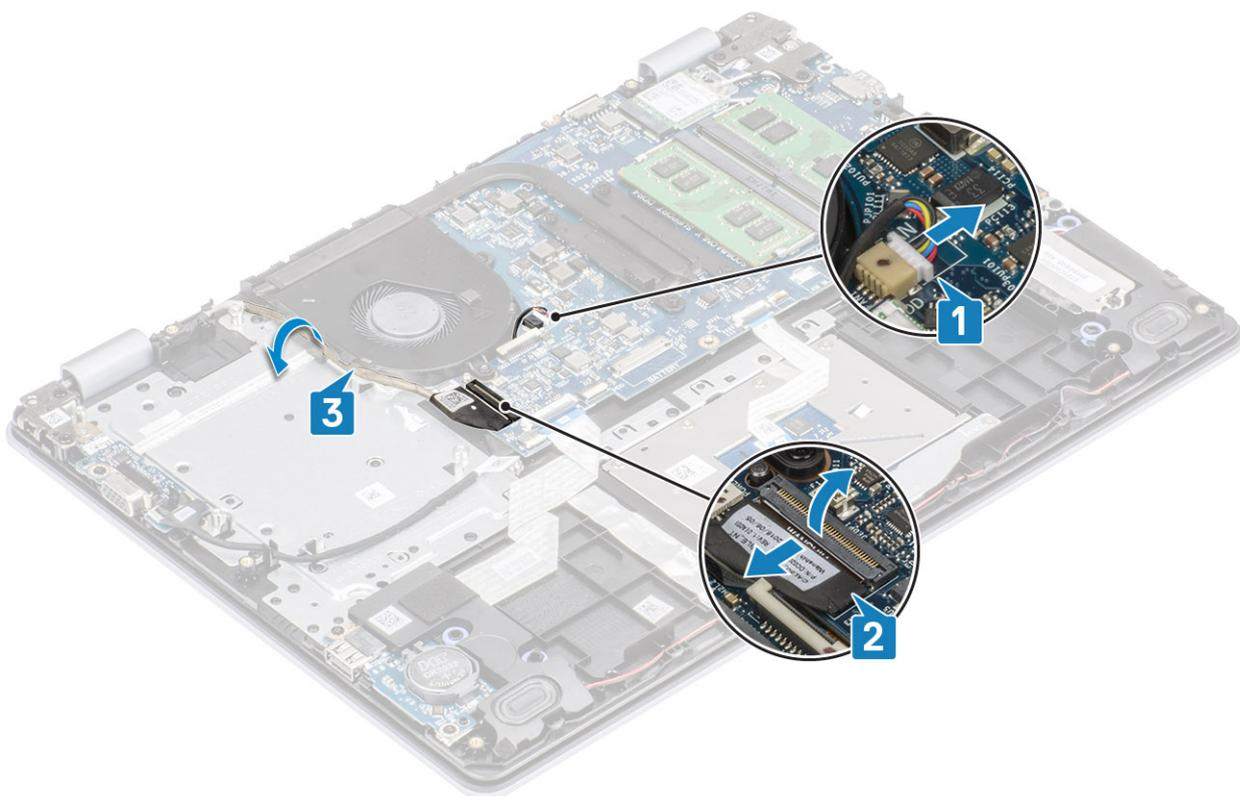
3. Remove the two (M2x5) screws that secure the fan to the palm rest and keyboard board assembly [1].
