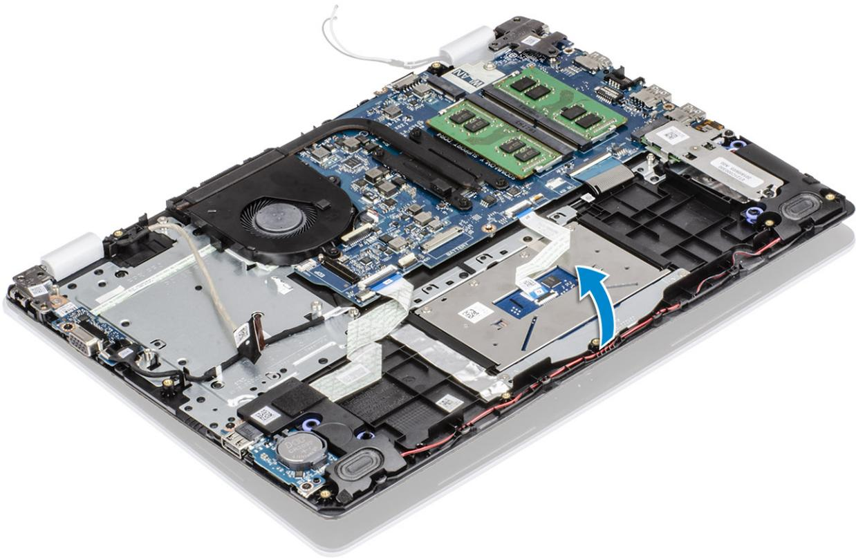
3. Replace the four (M2.5x6) screws that secure the left and right hinges to the system board, and palmrest and keyboard assembly.
