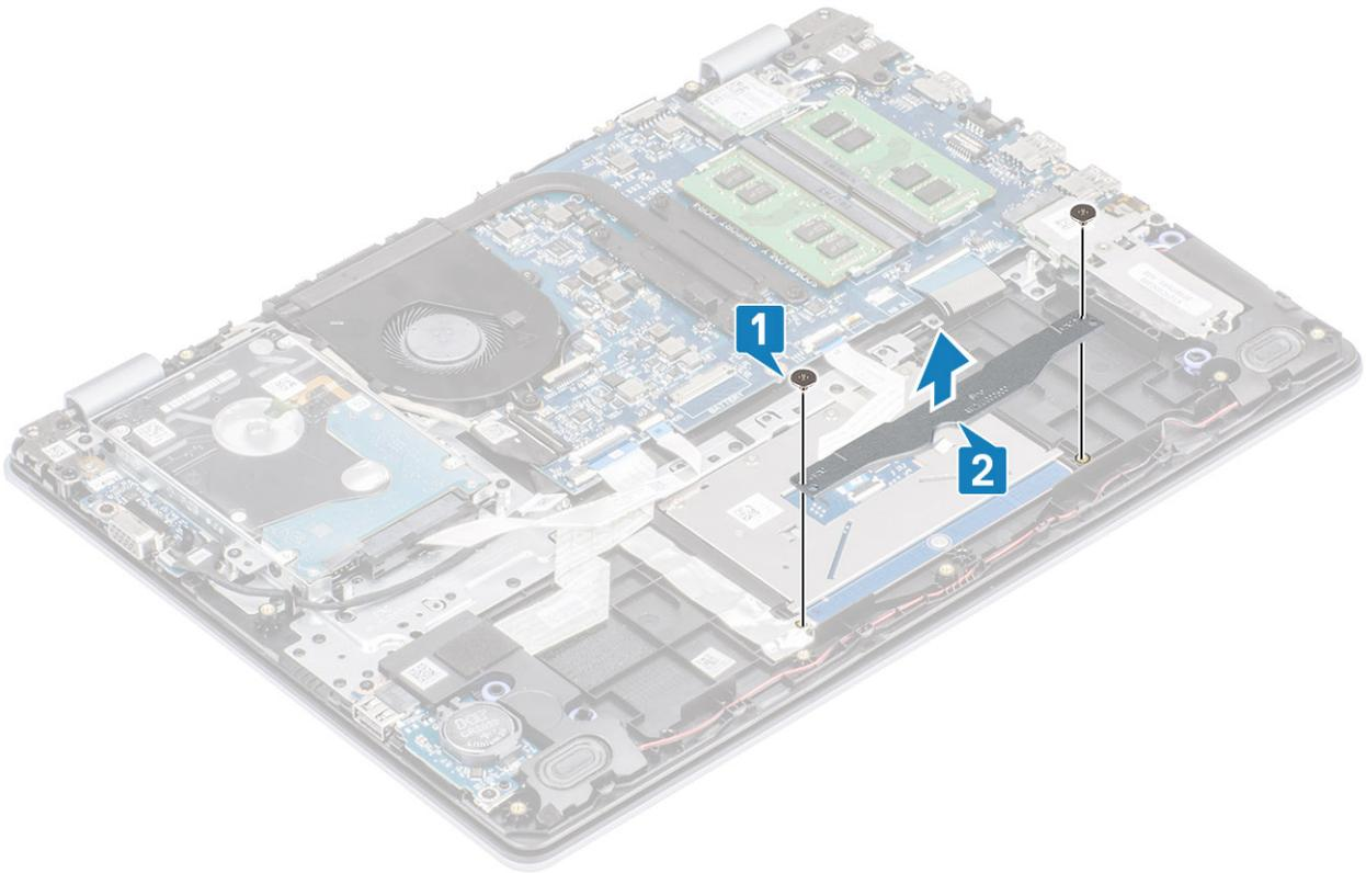
3. Open the latch and disconnect the touch pad cable from the system board [1].
