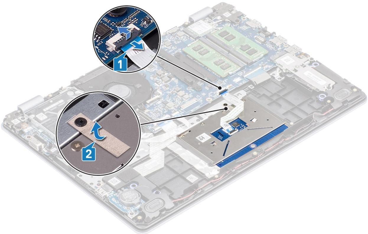
5. Remove the four (M2x2) screws that secure the touch pad to the palmrest and keyboard assembly [1].
