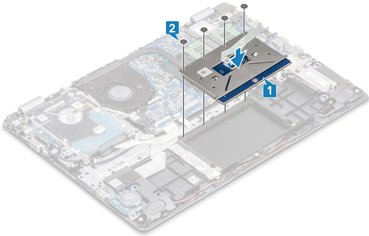
3. Adhere the tape that secures the touch pad to the palmrest and keyboard assembly [1].
