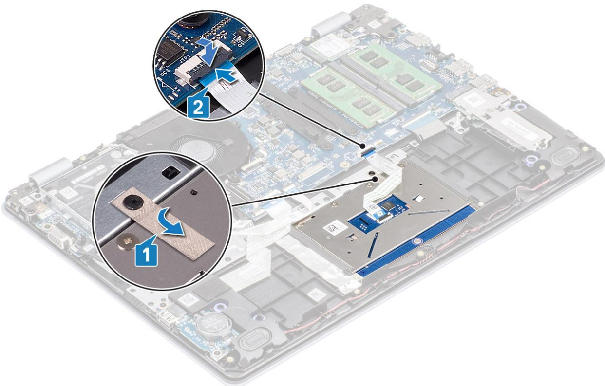
5. Place the touch pad bracket into the slot on the palmrest and keyboard assembly [1].
