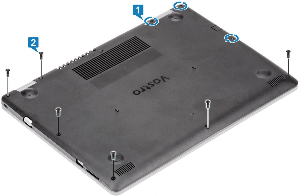
3. Pry the base cover from the top-right corner [1] and continue to open the right side of the base cover [2].
