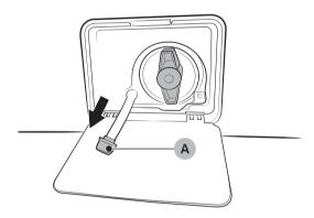
**3.** Put an empty, spacious container around the cover, and stretch the emergency drain tube to the container while holding the tube cap (A).
