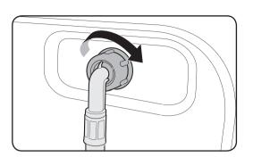
**8.** Connect the other end of the water hose to the inlet valve on the back of the washing machine. Turn the hose clockwise to tighten.
