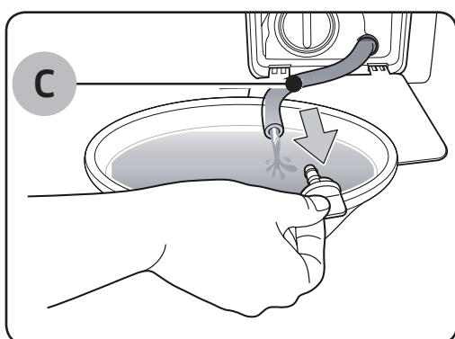
4. Open the tube cap and let water in the **Emergency drain tube (C)** flow into the container.
