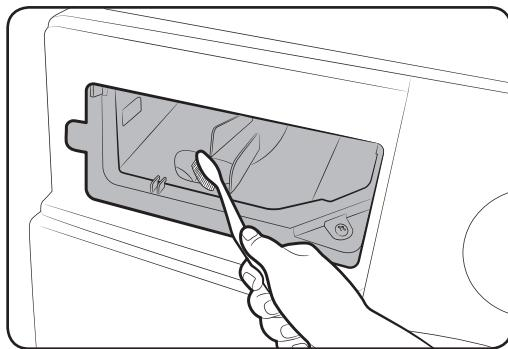
1. While holding down the **release lever (A)** on the inner of the drawer, slide open the drawer.
