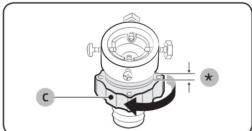
3. Hold the adaptor and turn part (C) in the arrow direction to loosen it by 5 mm (\*).
