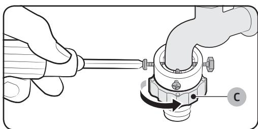
4. Insert the adaptor into the water tap, and tighten the screws while lifting up the adaptor.
