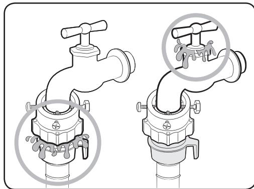
9. Open the water tap and check if there are any leaks around the connection areas. If there are water leaks, repeat the steps above.
