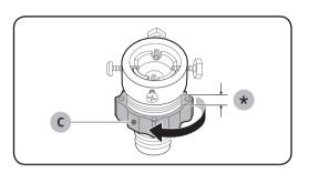
**3.** Holde the adaptor and turn part (C) in the arrow direction to loosen it by 5 mm (\*).
