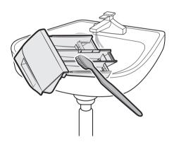
**2.** Clean the drawer components in flowing water using a soft brush.
