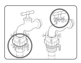
**9.** Open the water tap and check if there are any leaks around the connection areas. If there are water leaks, repeat the steps above.
