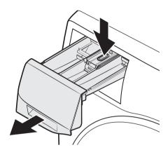
**1.** While holding down the release lever inside the drawer, slide open the drawer.
