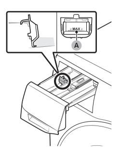
First insert the provided liquid detergent container in the II main-wash compartment. Then, apply liquid detergent to the container below the marked max line (A).
