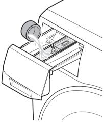
3. Apply fabric softener to the softener compartment. Do not exceed the max line.
