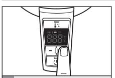
The display will show the default temperature 100° C. Press the "+" or "-" buttons to select your desired water temperature, from 50°C to 100°C.
