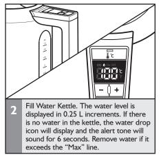
**NOTE:** There must be a minimum of 0.25 L of water for the Kettle to operate. Do not exceed the "Max" fill line.
