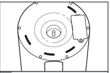
To provide power to the display when the Water Kettle is not on the base, insert 2 AA batteries (not inlcuded) in the battery housing on the underside of the kettle.
