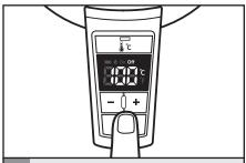
4 Once the desired temperature has been reached, three beeps will sound and the word "Off" will show in the top corner of the display.
