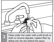
**NOTE:** If limescale deposits remain on the filter, let it stand overnight in a solution of water and white vinegar. Rinse the filter thoroughly and replace in the Water Kettle.
