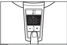
Press the Start/Cancel button ((b)) to save temperature and to begin heating the water. "On" will be displayed on the screen to indicate the Water Kettle is heating. The Start/Cancel button ((b)) does not function when the Water Kettle is off the base.
