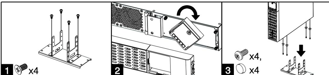
1. Attach the brackets to the baseplate with the provided M4 flat head screws.
