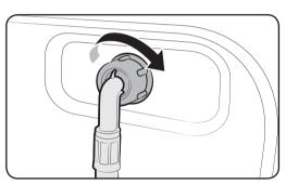
**8.** Connect the other end of the water supply hose to the inlet valve on the back of the washing machine. Turn the hose clockwise to tighten.
