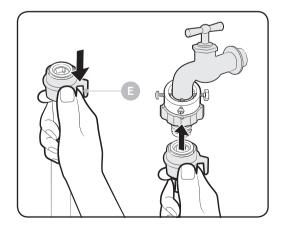
**6.** While holding down part (E), connect the water supply hose to the adaptor. Then, release part (E). The hose fits into the adaptor with a clicking sound.
