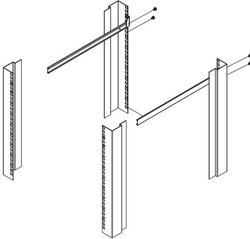
2. While one person inserts the unit into place by sliding its left and right side bars into the left & right L-shaped brackets (on the rack), have a second person screw the front brackets to the rack.
