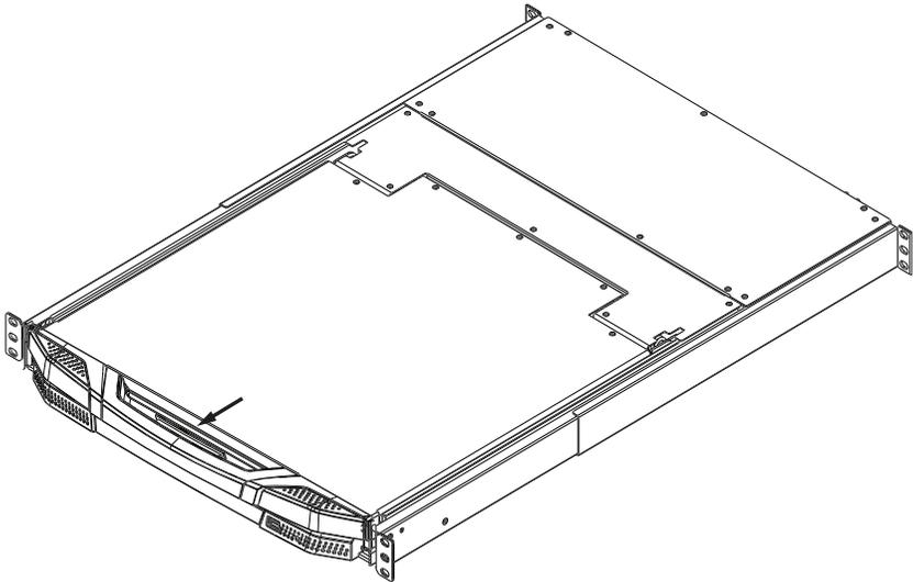
2. Slide the module all the way out until it automatically locks in place.
