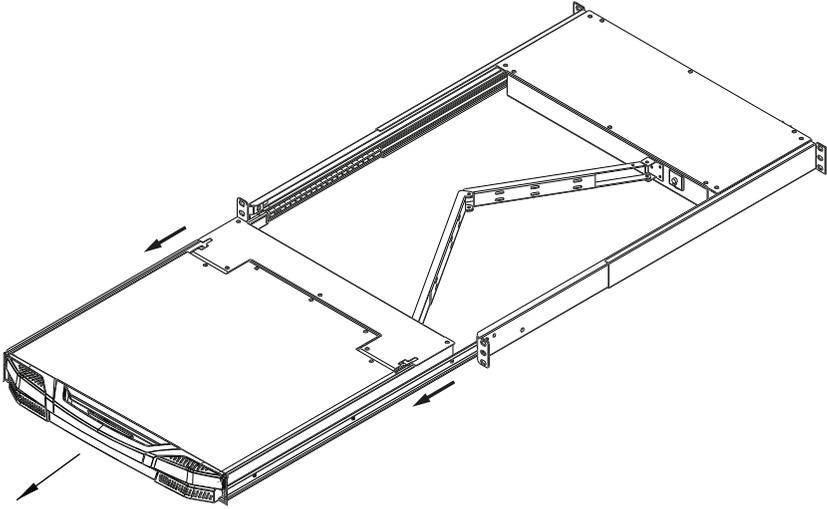
3. Open the cover by pulling the Release Bar on the handle as pictured below.
